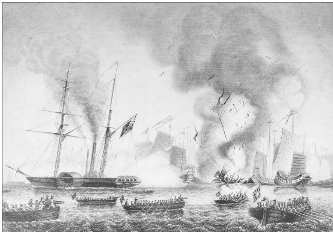
The Opium War: the British steam-powered paddle wheeler Nemesis destroying a Chinese fleet in a battle on January 7, 1841, near Guangzhou. Nemesis , aptly named, was one of the first iron-hulled steam vessels; it was designed with a shallow draft so that it could attack inland shipping. Its guns had far greater range and accuracy than those of the Chinese ships or shore batteries, and its easy success made it a symbol of Western naval and military superiority. (Rischgitz/Getty Images)
