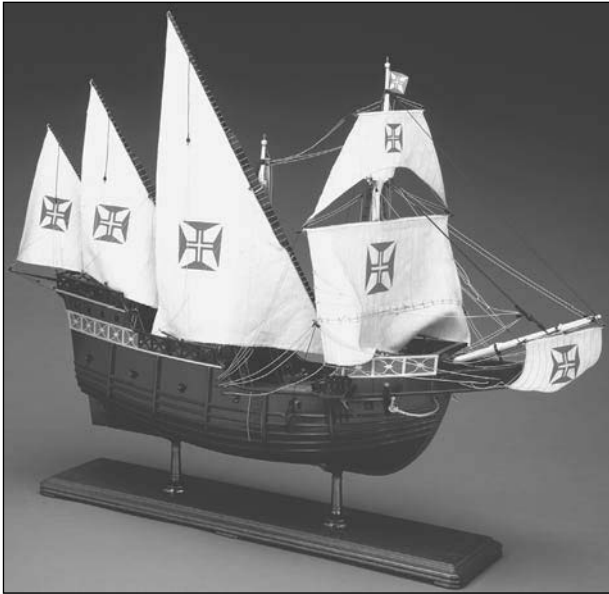
This model of a four-masted caravel illustrates the triangular lateen sails combined with square sails for sailing with the wind. ( Museu de Marinha, Lisbon, Portugal/National Maritime Museum )
