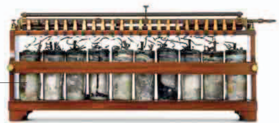
row of cells connected to terminals
