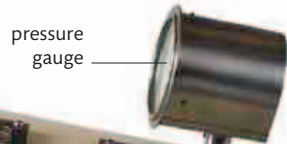
Pressure gauge The pressure generated for each patient was indicated on a gauge on top of the tank. Changes in pressure enabled the lungs to inflate and deflate.
