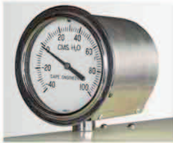
Pressure gauge The pressure generated for each patient was indicated on a gauge on top of the tank. Changes in pressure enabled the lungs to inflate and deflate.
