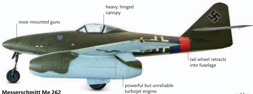
Messerschmitt Me 262 With a top speed of 540 mph (869 km/h) the Messerschmitt was the world's first turbojet fighter and regarded as the best fighter plane of WWII.
