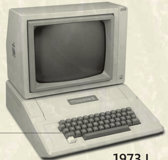
keyboard integrated with body of computer
