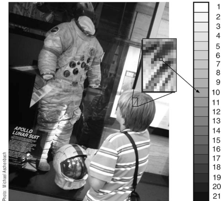
Fig. 1.23 Black and white photo, with one pixel of Ian’s hair depicted. Also shown is the scale of shades of grey , with the actual shade of the chosen pixel corresponding to the number 10. The photo highlights the broad range of STEM education and expectations
