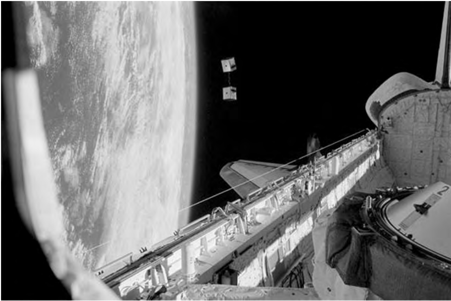
Figure 4.12: MEPSI-1A and -1B, connected by a short tether, are released from the Space Shuttle on mission STS 113. (Courtesy of NASA.)
