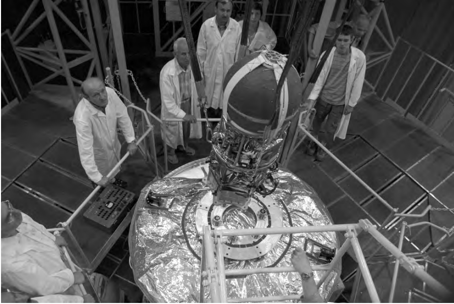
Figure 4.15: YES-2 being lowered onto the Foton-M3 spacecraft in preparation for launch. (Courtesy of ESA.)
