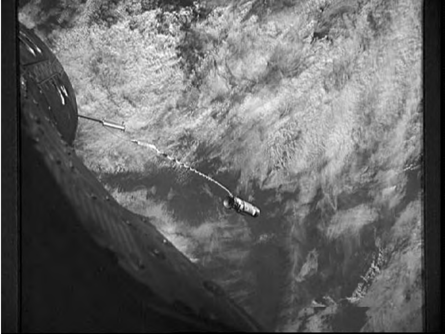
Figure 4.3: The Agena and tether seen from Gemini 12, in their gravity-gradient stabilized position. (Courtesy of NASA.)
