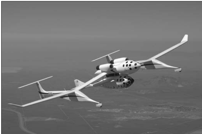
Figure 22-1: SpaceShipOne (lower center) aboard the White Knight carrier aircraft, which lifts SpaceShipOne off the ground for an air launch.
