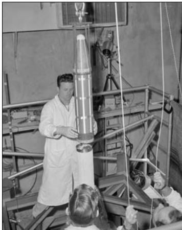
Figure 6-2: The Explorer 1 satellite, which was smaller than Sputnik 1 , had a cylindrical design, much like a small rocket.
