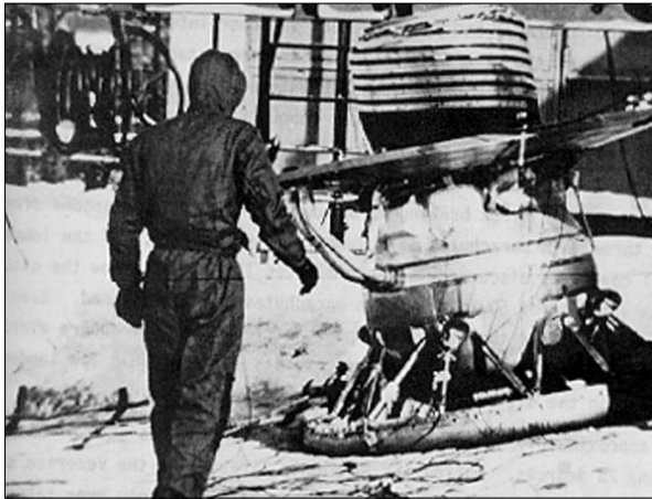
Figure 11-2: The Soviets used Venera landers (shown during testing) to explore Venus.
