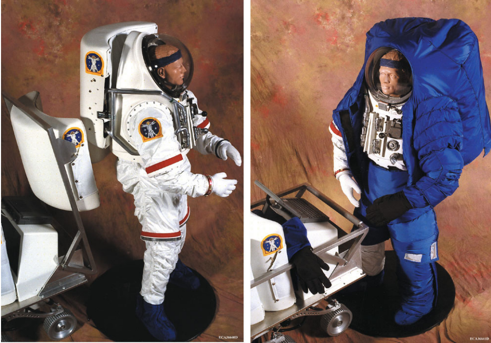
Figure 11.3.22. Changeable PLSS and removable garments mockup (courtesy Hamilton Sundstrand).
