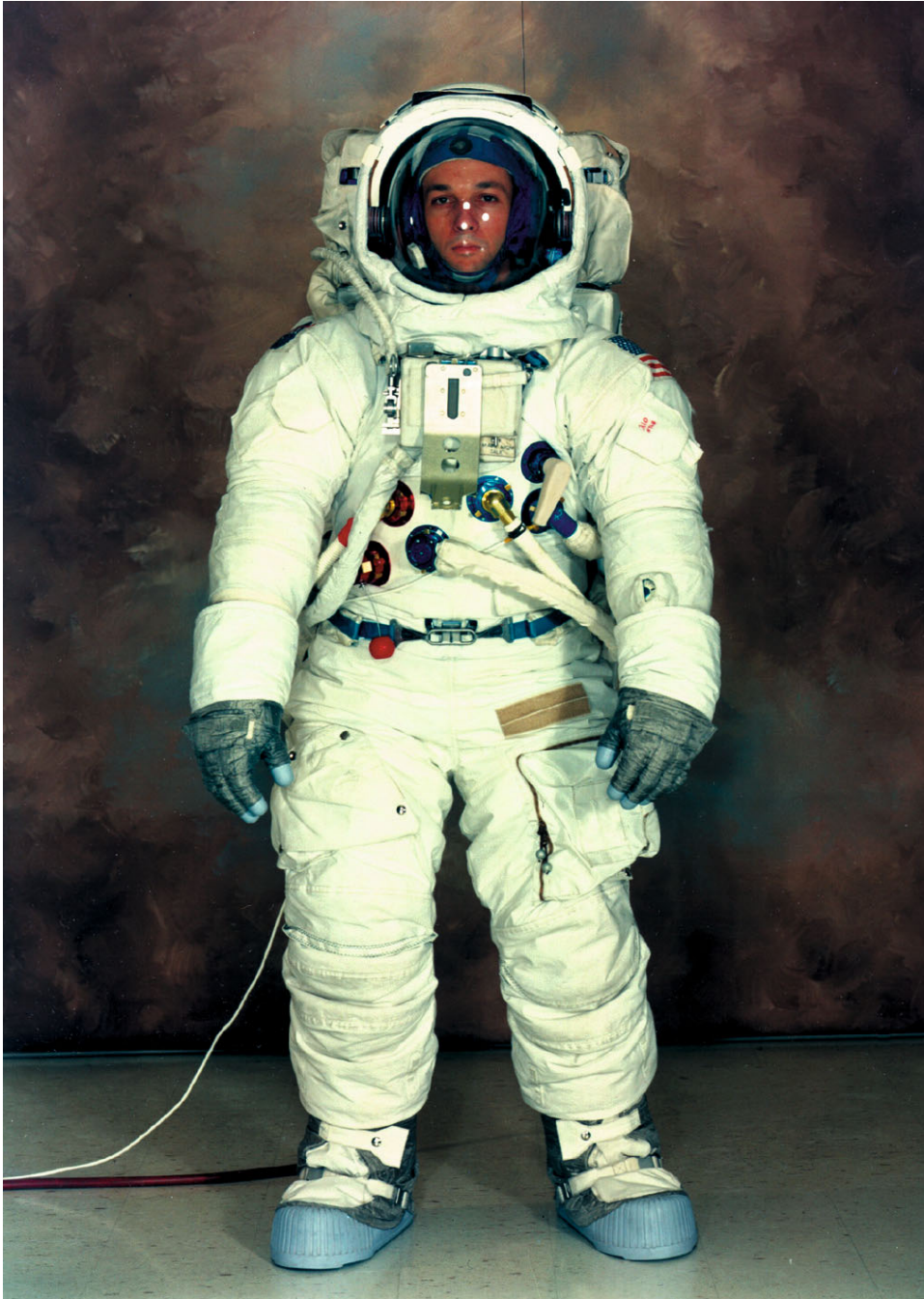
Figure A.9. Apollo 15–17: EMU (ILC A7LB suit, HS-7 portable life support system) (courtesy G. L. Harris).
