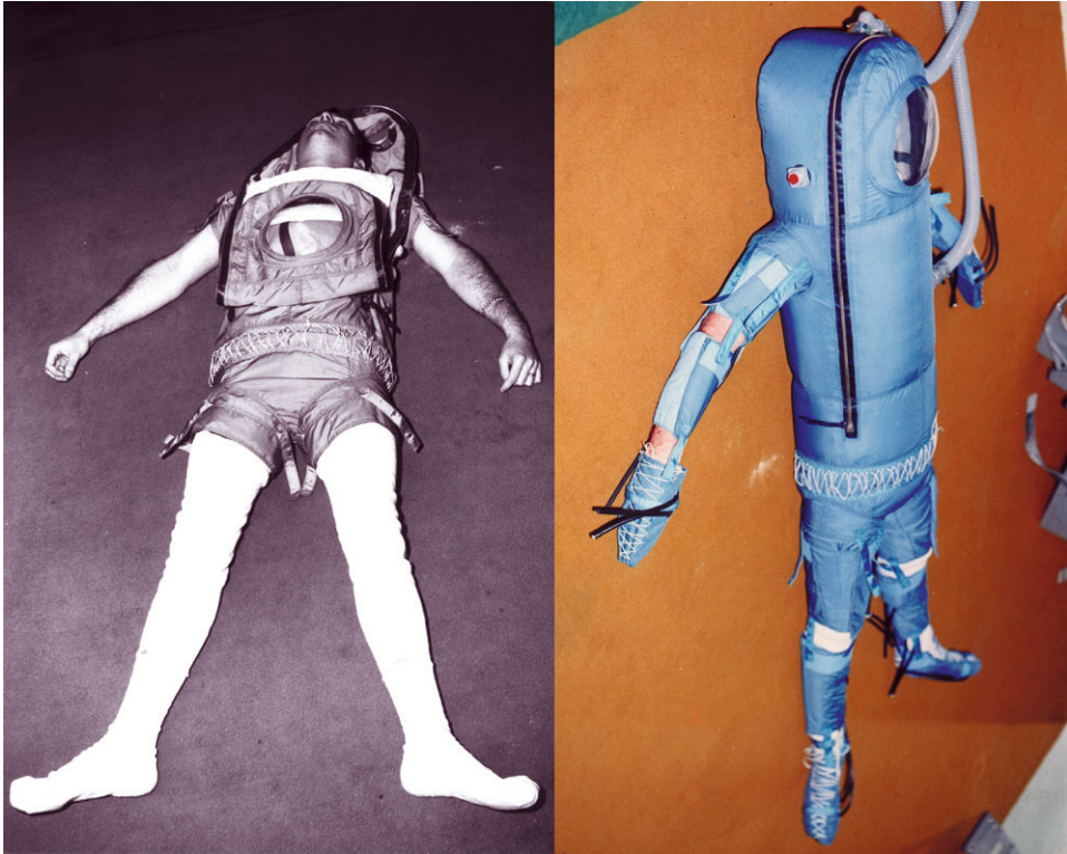
Figure 8.4.7. 1969 human testing of SPCA suit (courtesy Hamilton Sundstrand).
