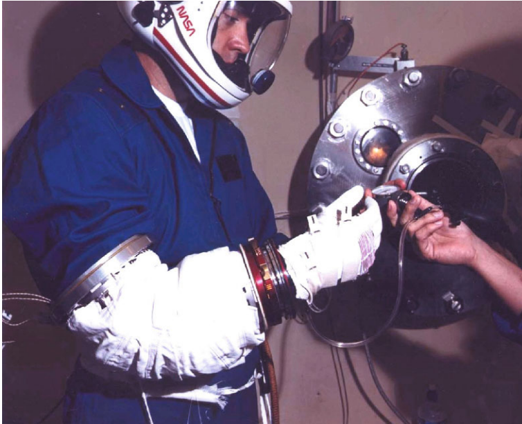
Figure 11.3.16. Honeywell mechanical counter-pressure (MCP) glove (courtesy NASA).
