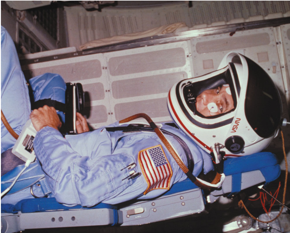
Figure 4.5.2. DCC 1982–1986 launch/entry helmets (courtesy NASA).
