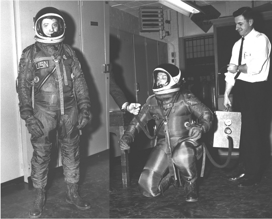
Figure 2.7. 1959 era BFG Mark III/IV-type full pressure suit (courtesy Hamilton Sundstrand).
