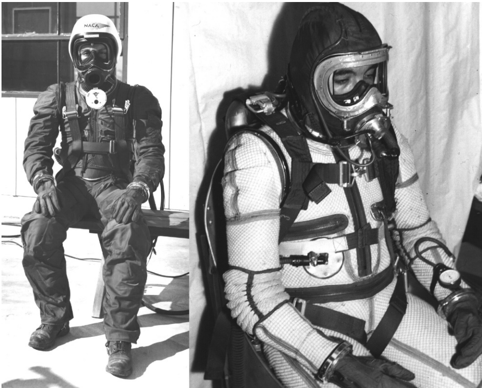
Figure 2.6. 1951 DCC D-558-II full pressure suit with “Link-net” (courtesy, left and right, David Clark Co. and G. L. Harris, respectively)
