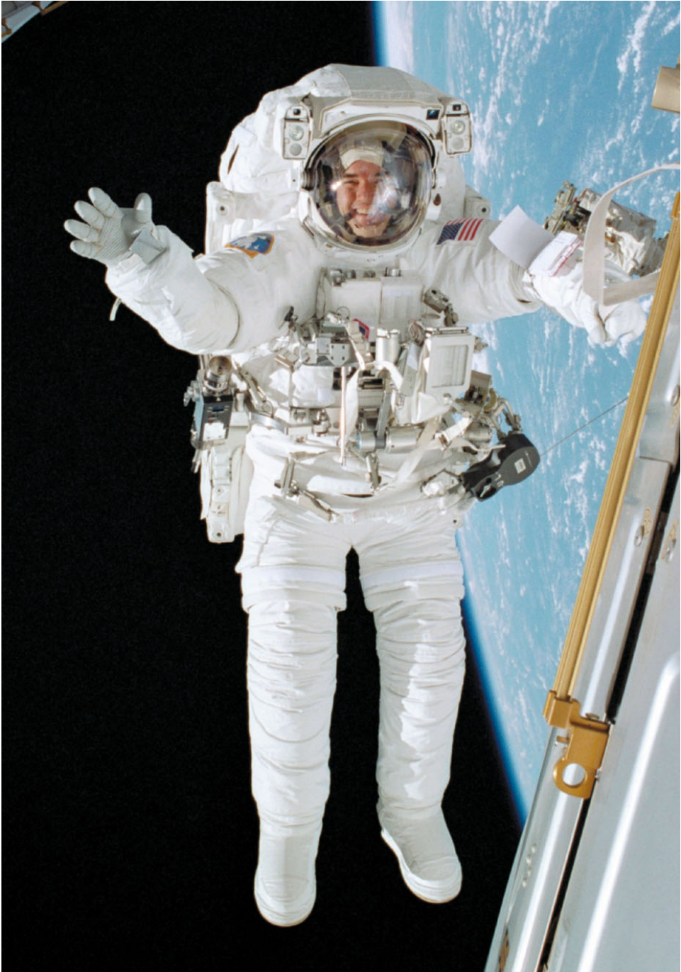
Figure A.15. HS/ILC Shuttle enhanced EMU EVA spacesuit system (courtesy NASA).
