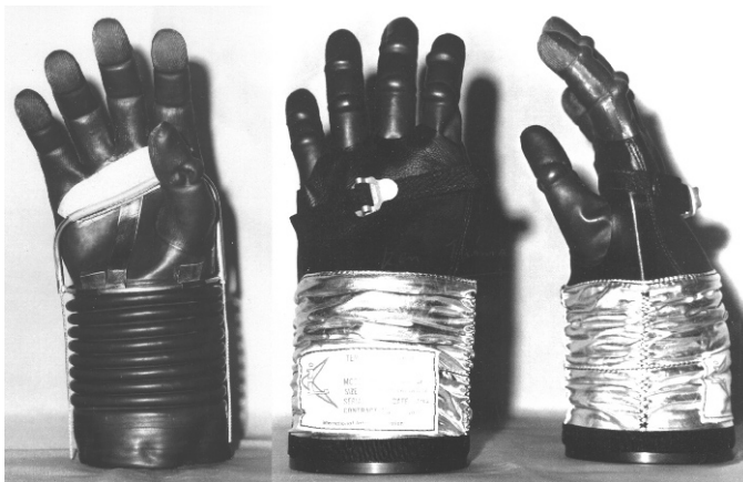
Figure 6.2.2. 1963–1964 Apollo pressure glove views (courtesy ILC Dover LP).
