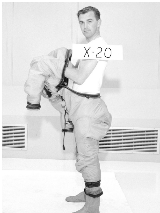
Figure 8.1.1. David Clark Co. (DCC) X-20 suit restraints and entry (courtesy Hamilton Sundstrand).
