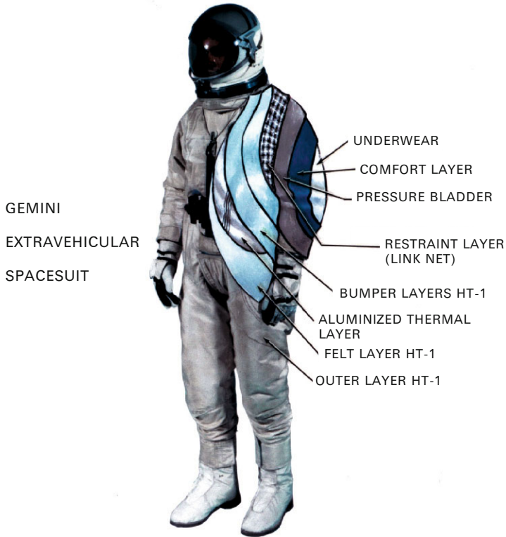
Figure 5.3.1. DCC Gemini IV suit materials (courtesy NASA).
