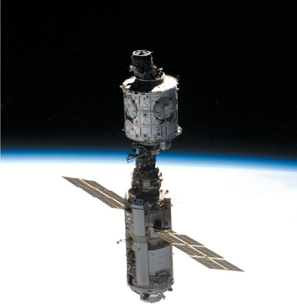
Figure 10.2.12. First step in assembling the ISS completed (courtesy NASA).
