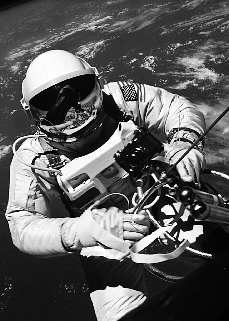
Figure A.4. Gemini IV DCC G4C suit, NASA/AiResearch ventilation control module (courtesy NASA).
