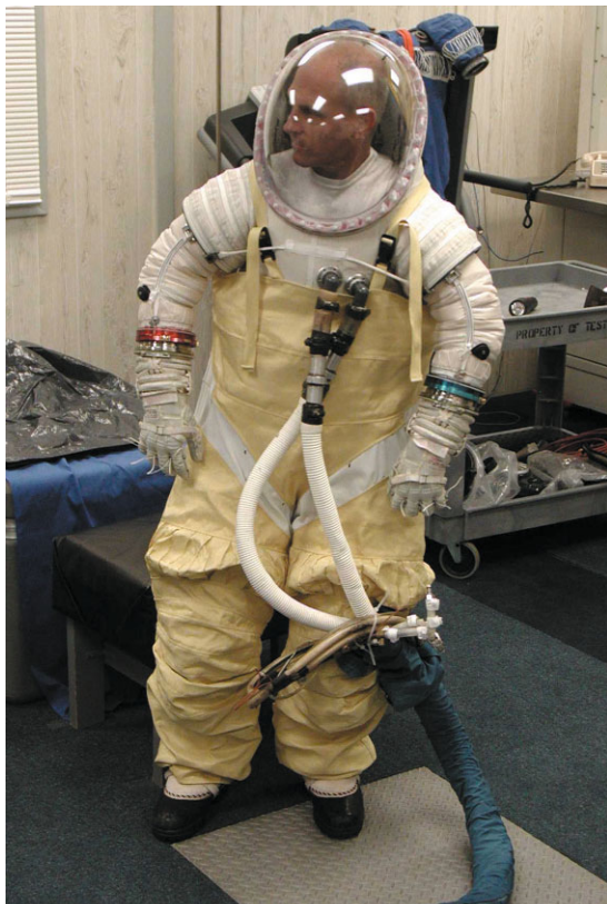
Figure 11.3.30. 2008 fifth-generation all soft recompetition I-suit (courtesy ILC Dover, Fredrica, DE).
