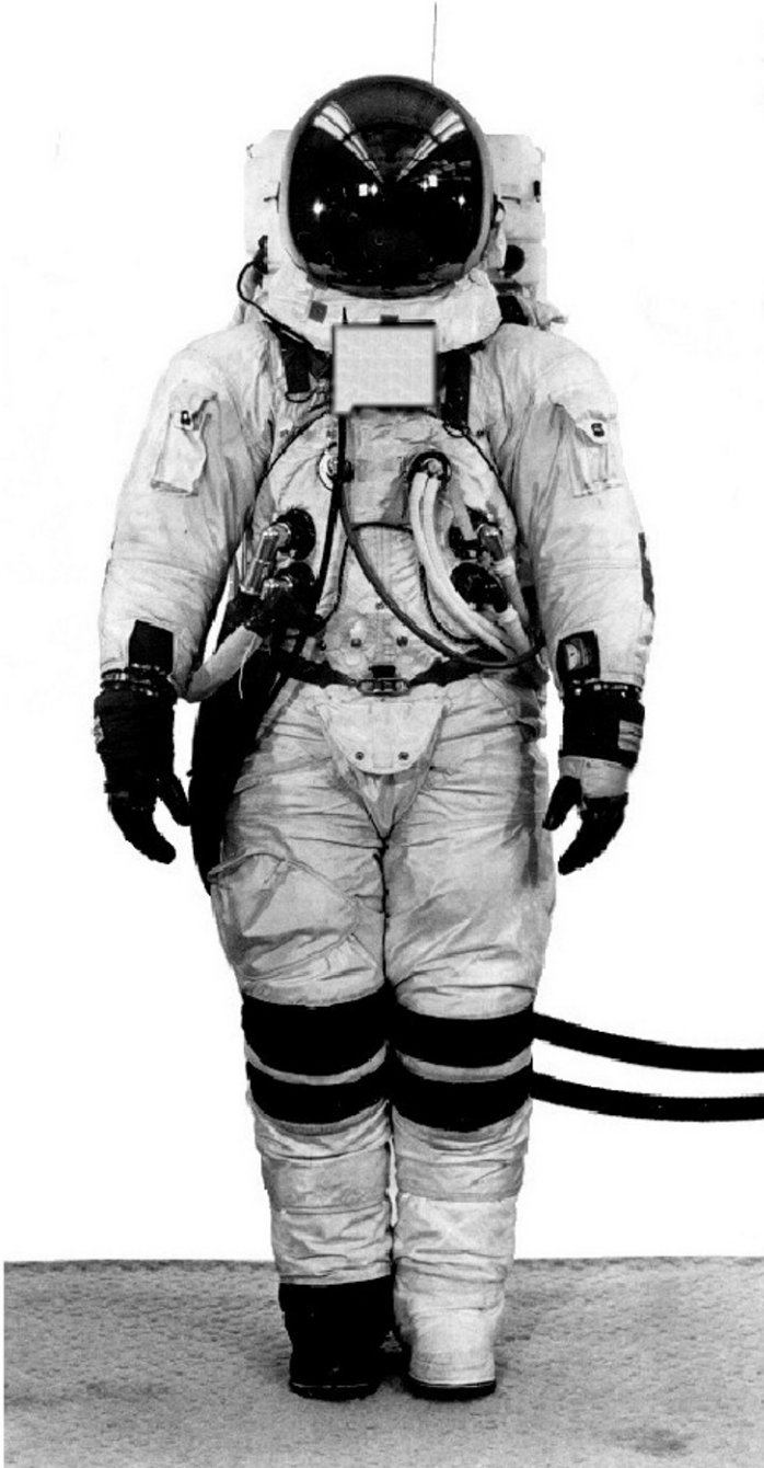
Figure A.7. Apollo 9 and 10: EMU (ILC A7L suit, HS-5 portable life support system) (courtesy Hamilton Sundstrand). Note: Development/certification EMU shown.
