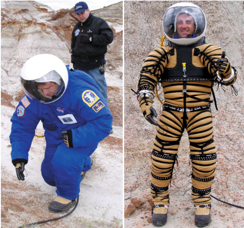
Figure 11.3.6. 2006 NDX-1 prototype (with and without cover garments) (courtesy University of North Dakota).
