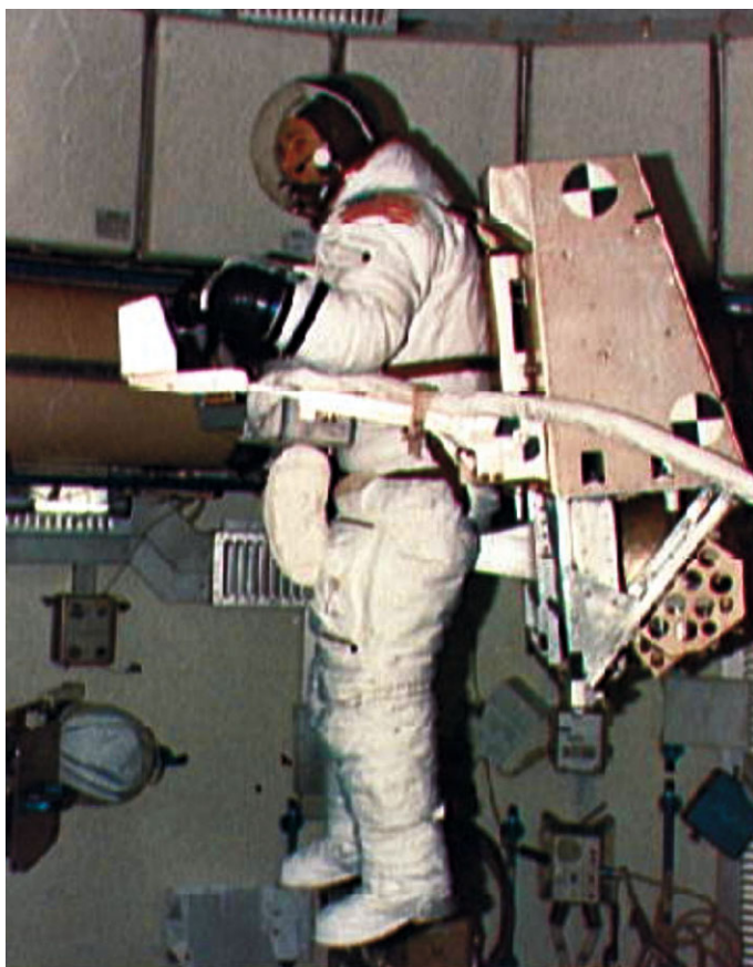
Figure 9.4.4. Alan Bean in IVA test of the automatically stabilized maneuvering unit (courtesy NASA).
