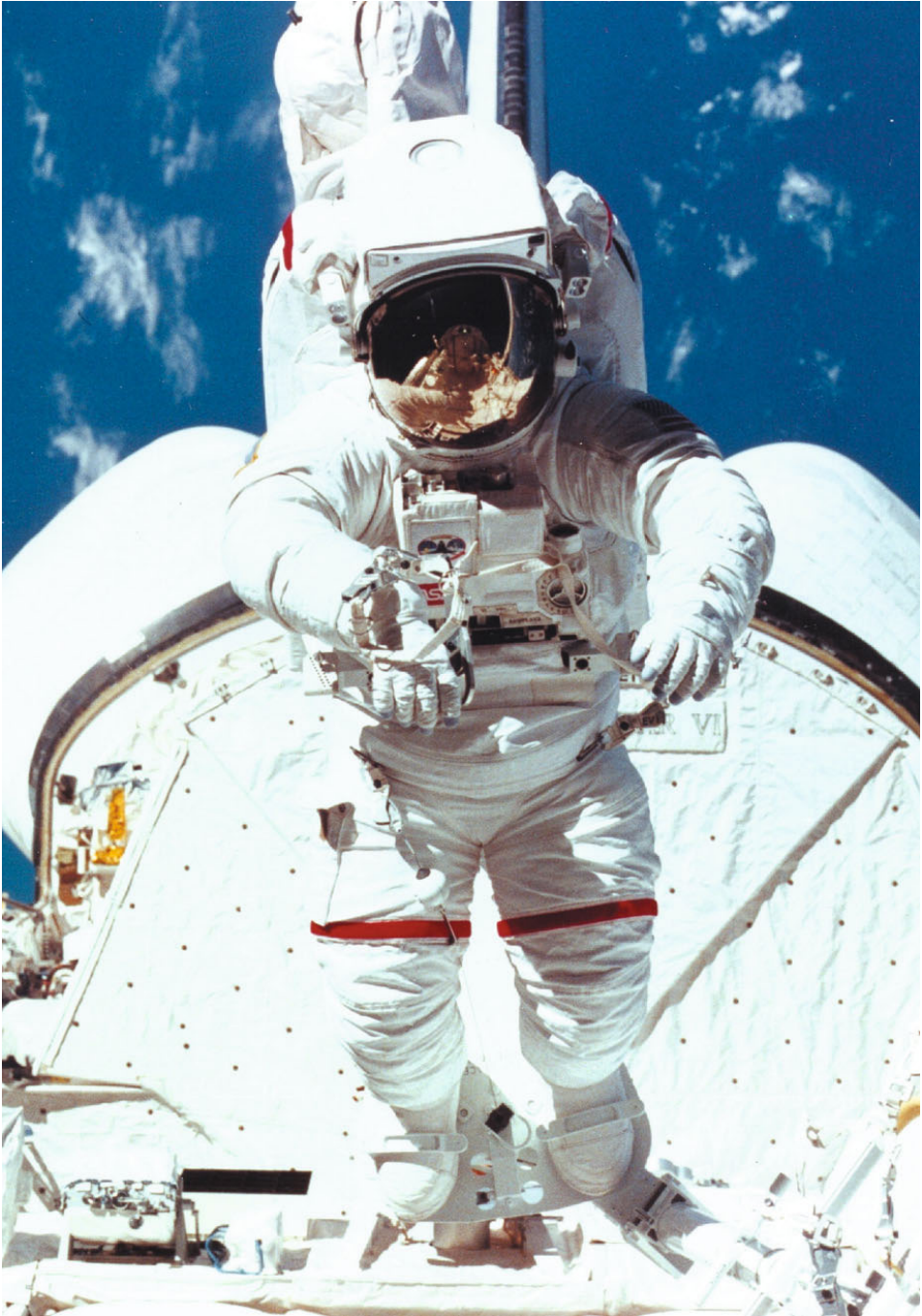
Figure A.12. HS/ILC Shuttle baseline EMU EVA spacesuit system (courtesy NASA).
