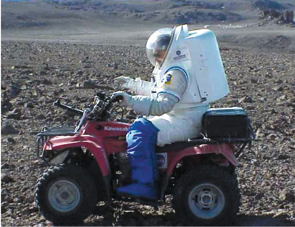
Figure 11.3.19. Evaluating transportation/suit interfaces (courtesy Hamilton Sundstrand).
