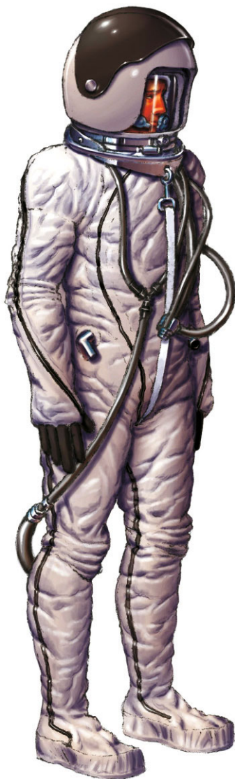
Figure 8.2.1. Mauch mechanical counterpressure suit.
