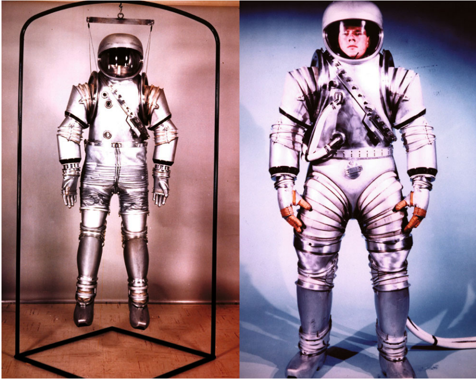
Figure 7.1.1. Litton’s RX-1 (left) and RX-2 (right) prototypes (courtesy Hamilton Sundstrand).
