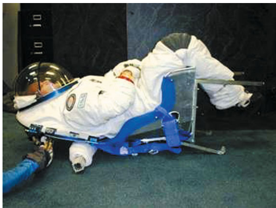
Figure 11.3.29. ILC fourth-generation I-suit in launch comfort demo (courtesy ILC Dover, Fredrica, DE).
