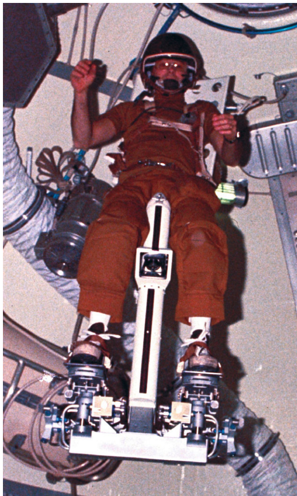
Figure 9.4.5. Owen Garriott testing the foot-controlled maneuvering unit (courtesy NASA).
