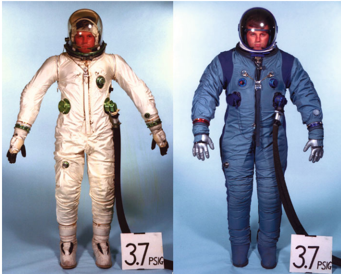
Figure 6.5.9. DCC (left) AX1C and HS/BFG AX6H 1965 (right) competition suits (courtesy NASA).
