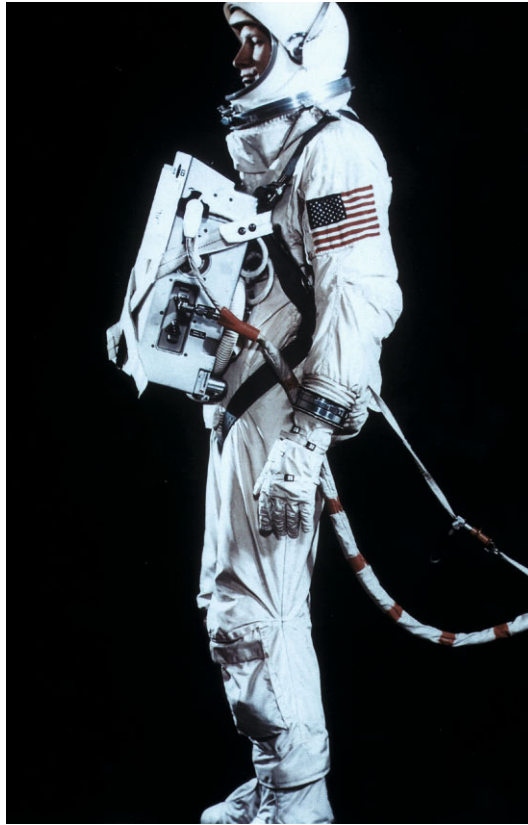
Figure 5.6.9. Gemini X to XII base suit system configuration (courtesy NASA).
