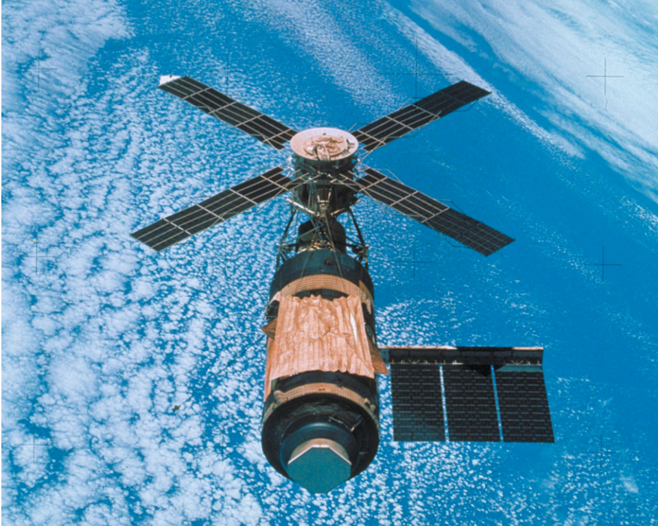
Figure 9.4.3. Thermal shield in place on Skylab (courtesy NASA).
