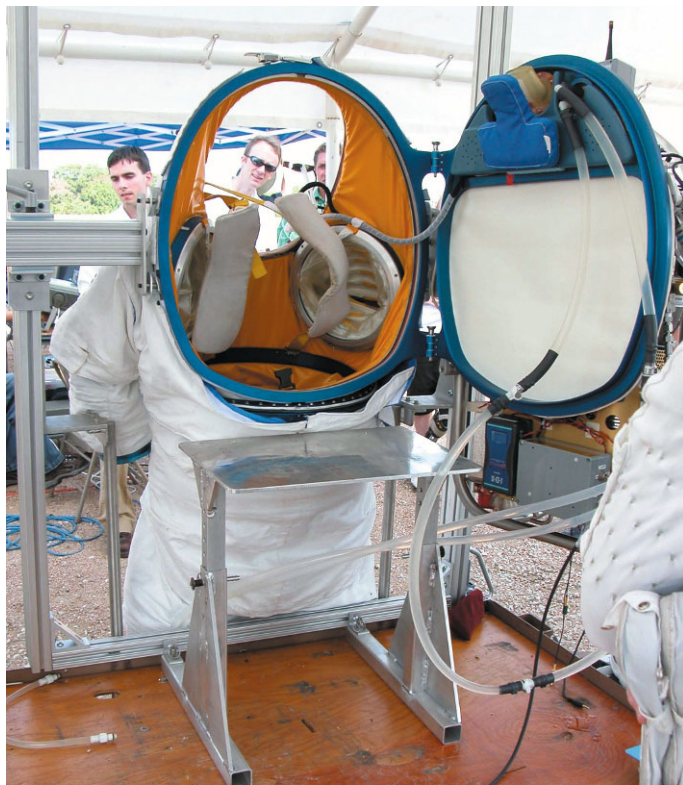
Figure 11.3.26. Rear-entry 2005 ILC third-generation I-suit (courtesy ILC Dover, Fredrica, DE).
