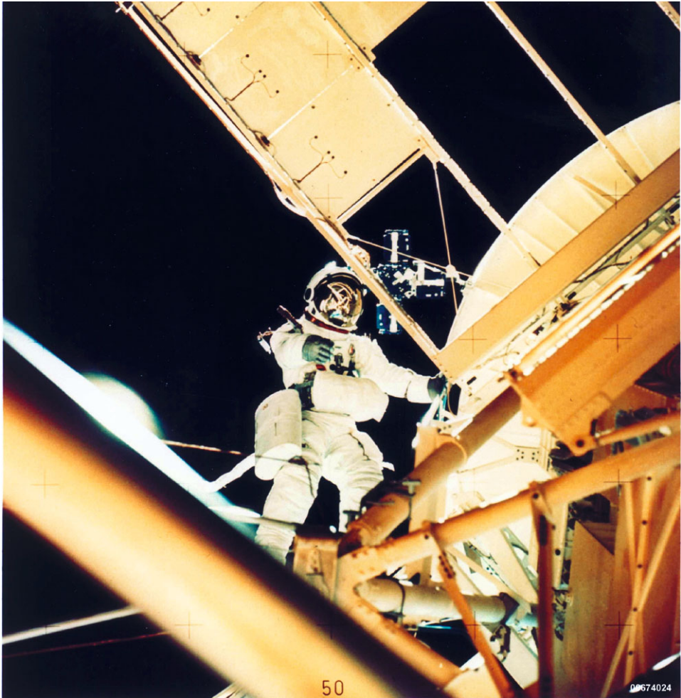
Figure 9.3.7. SOP shown on Owen Garriott's EMU during a Skylab 3 EVA (courtesy NASA).
