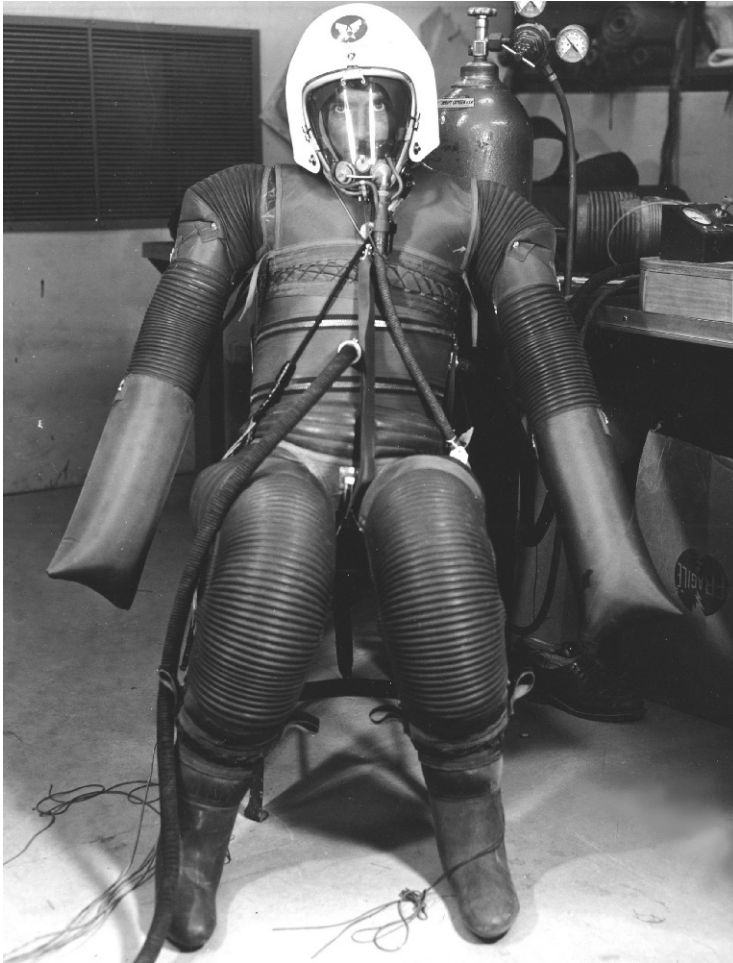
Figure 4.1.1. 1957 International Latex XMC-2-ILC X-15 prototype (courtesy ILC Dover LP).
