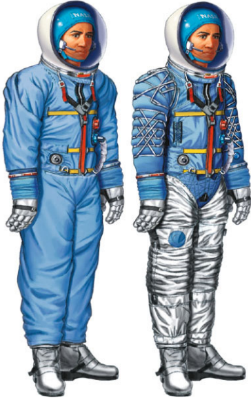
(R) HS "mobility suits"— modified ILC suits (1/65) (a) External view (b) Without covers
