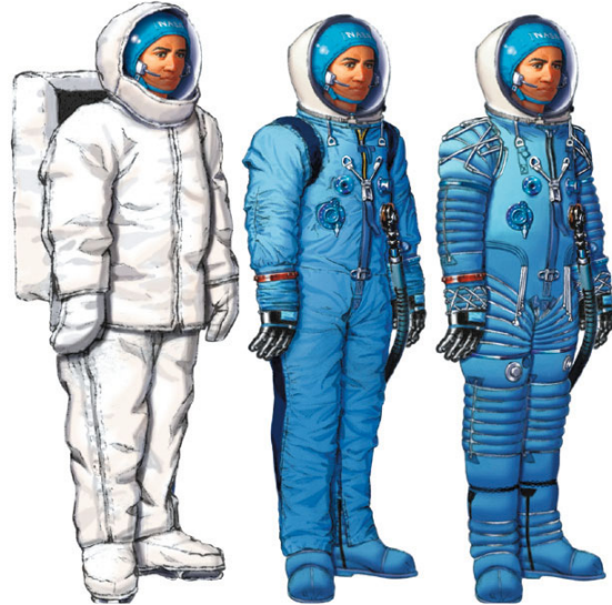
(U) HS AX5H suits (3/65–6/65) (a) EVA external view (b) IVA external view (c) Without covers
