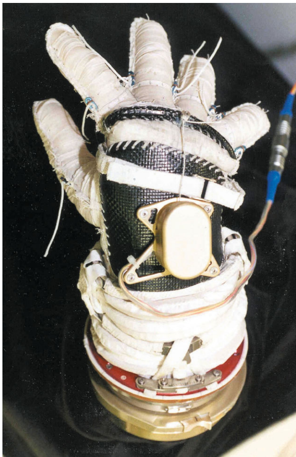
Figure 11.1.19. University of Maryland/ILC power-assisted glove (courtesy ILC Dover LP).
