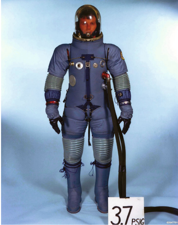
Figure 6.5.10. The ILC AX5L 1965 competition suit (courtesy NASA).
