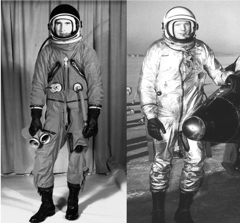
Figure 4.1.4. The DCC A/P 22S-2 improved X-15 aviation/space suit (Pilot Neil Armstrong, right) (courtesy David Clark Co.).
