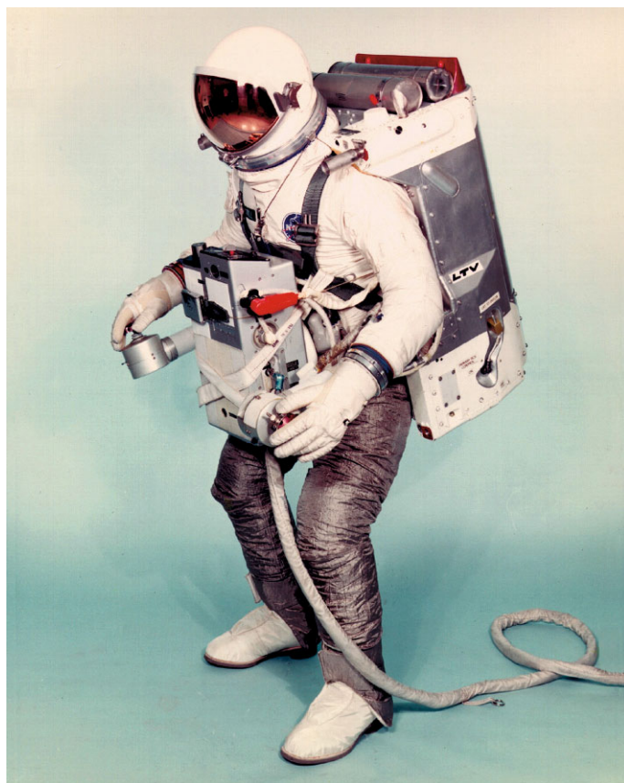
Figure 5.6.5. The Gemini IX EVA suit system (courtesy NASA).
