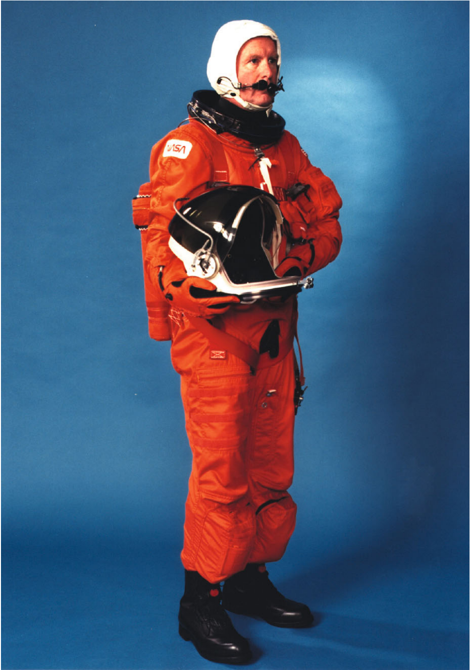
Figure A.13. DCC Shuttle launch/entry IVA spacesuit system (courtesy David Clark Co.).
