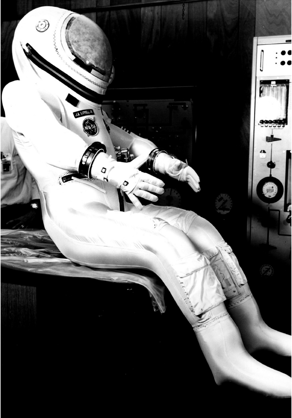
Figure A.6. DCC Gemini VII G5C IVA spacesuit (courtesy NASA).
