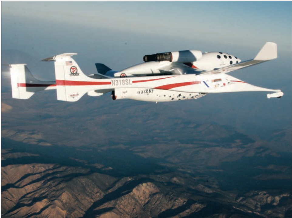
Slung under White Knight , SpaceShipOne was carried upward on this flight, the first of two required by the Ansari X Prize rules.
