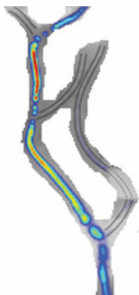
Figure 9.7 Example of microscopic submarines being steering along the planned path using DFN.
