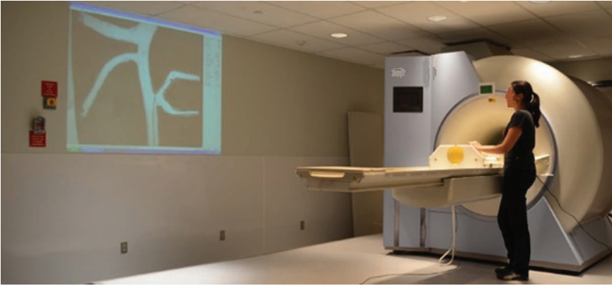
Figure 8.1 Photograph showing an MRI-tracked position plotted on a computer-generated map of an arterial network being projected at a larger scale on one of the walls of the interventional room.
