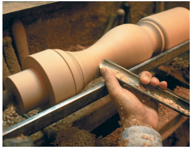
A lathe turns an object on a horizontal axis so it can be cut with a fixed tool. Photograph by Pedro Coll. Stock Market. Reproduced by permission.
