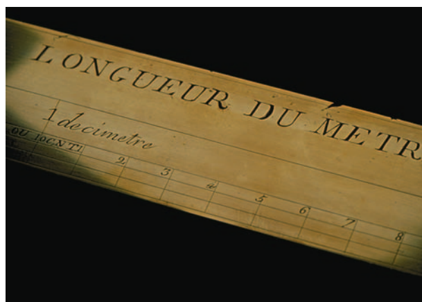
The first provisional standard scale of a meter. Made of copper in 1793, the scale is housed in the Archives Nationales de France, Paris. Photograph by Thomas Ernsting. Stock Market. Reproduced by permission.
