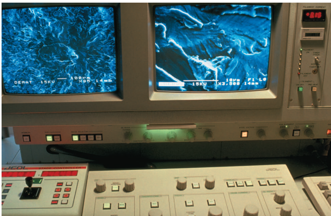
A scanning electron microscope at the Billancourt Centre, Boulogne, France. This system is used in the testing of Renault Sport's motor racing engines. The samples on screen are the fracture faces of components subjected to a tensile strength test. Photograph by Philippe Plailly. Eurelios/Science Photo Library, National Audubon Society Collection/Photo Researchers, Inc. Reproduced by permission.
