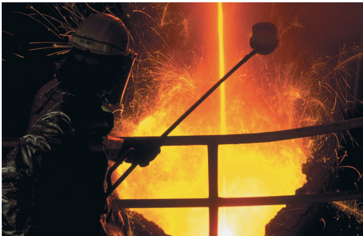
A steel worker sampling the quality of “hot steel” during production. Photograph by John Olson. Stock Market. Reproduced by permission.
