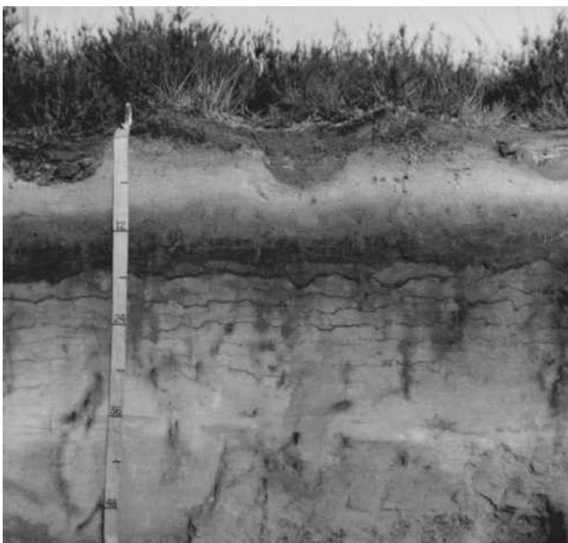
Photograph of a soil profile showing horizons. The dark crescent-shaped spots at the soil surface are the result of plowing. The dark horizon is the principal horizon of accumulation of organic matter that has been washed down from the surface. The thin wavy lines were formed in the same manner. 1 in. = 2.5 cm.
