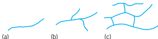
Fig. 1. Polymer chains. (a) Linear polymer chain. (b) Branched polymer chain. (c) Cross-linked polymer chain.
