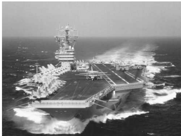
Fig. 2. Nuclear-powered aircraft carrier, Nimitz CVN 68 class. USS Theodore Roosevelt (CVN 71) is shown. (U.S. Navy photo)
