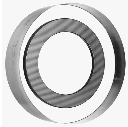
Optical flat being used to determine flatness of seal ring. Interference bands on seal ring face show lines of constant depth. (Van Keuren Co.)
