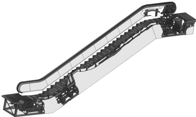
Cutaway view of escalator. (Otis Elevator Co.)
