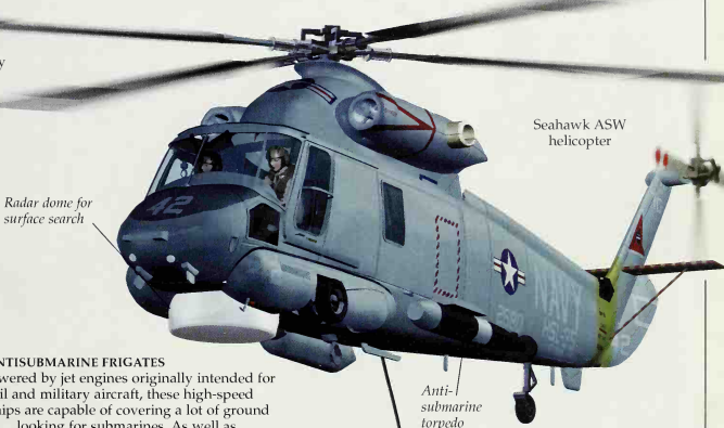
Helicopter drops device into water to listen for submarines
