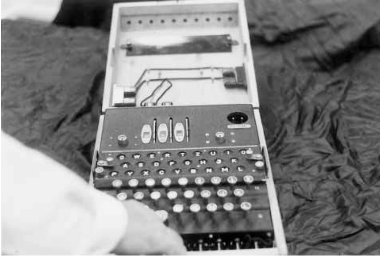
Plate 9.3 The Enigma with lid closed, ready for use. The current positions of the three wheels are visible through the windows.
