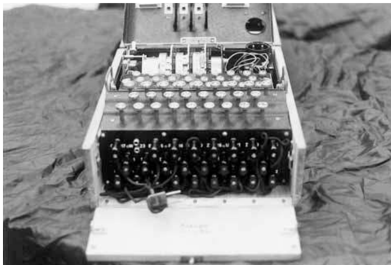
Plate 9.4 The Enigma with the top and flap open. The three wheels and reflector are now visible as is the plugboard at the front.
