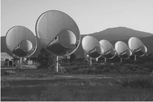
Part of the Allen Array, a set of 42 radio dishes in northern California that can do general radio astronomy, but also the most powerful SETI experiment in history. The eventual goal is 350 dishes, all acting in concert to look for artificial radio signals from many thousands of stars like the Sun at distances of up to a few thousand light years (courtesy SETI Institute).
