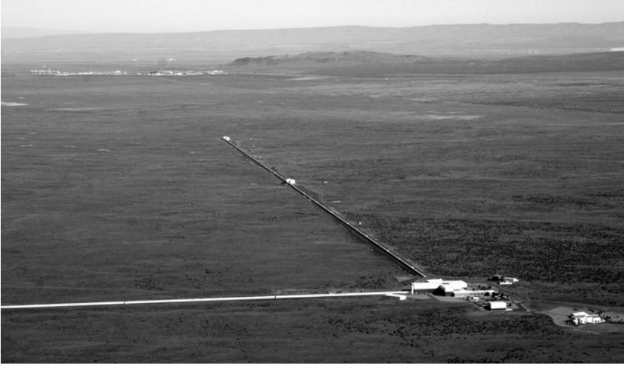
Fig. 4.11 The LIGO Hanford Observatory, in Washington State, consists of two 4-km arms at right angles, each with laser beams in high vacuum. There is an identical observatory in Louisiana, and the two installations work in tandem. The objective is to detect gravity waves by searching for changes in arm length that are a thousand times smaller than an atomic nucleus. (Credit: LIGO Laboratory)
