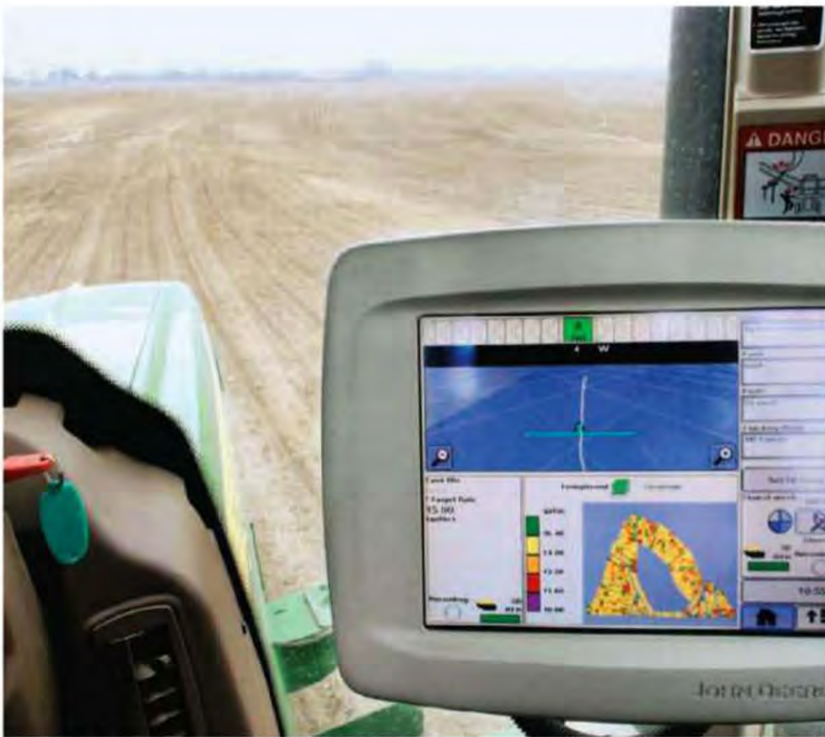
GPS TECHNOLOGY installed in his tractor helps an Illinois farmer track his path as he spreads fertilizer and sprays herbicides.
