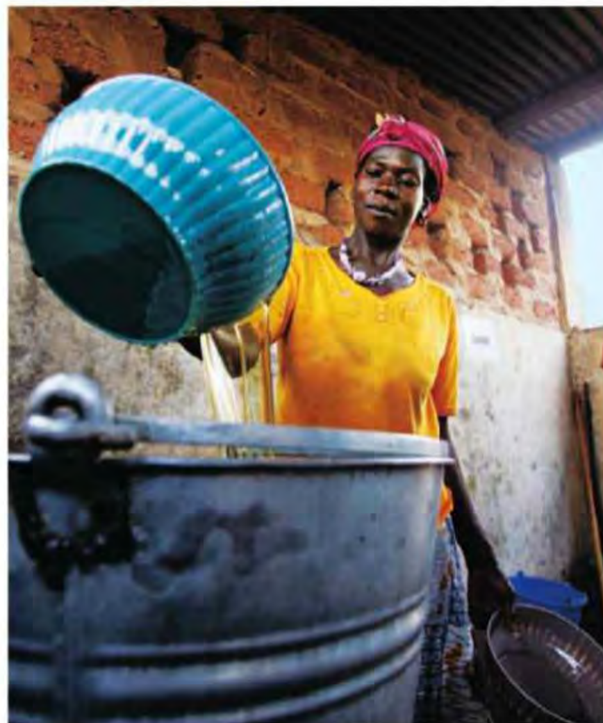
STRAINING OFF THE OIL extracted from shea or karite nuts, a woman in Burkina Faso performs one of the many arduous steps in manufacturing shea butter. Women from her country produced 20 tons in 2007.
