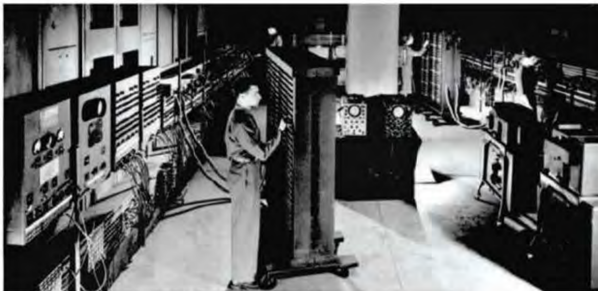
THE WORLD’S FIRST MODERN COMPUTER, ENIAC —an acronym for Electronic Numerical Integrator and Computer—required an entire room at the University of Pennsylvania. Shown here in 1946, it generated 150 kilowatts of heat and could perform a record 5,000 additions per minute.
