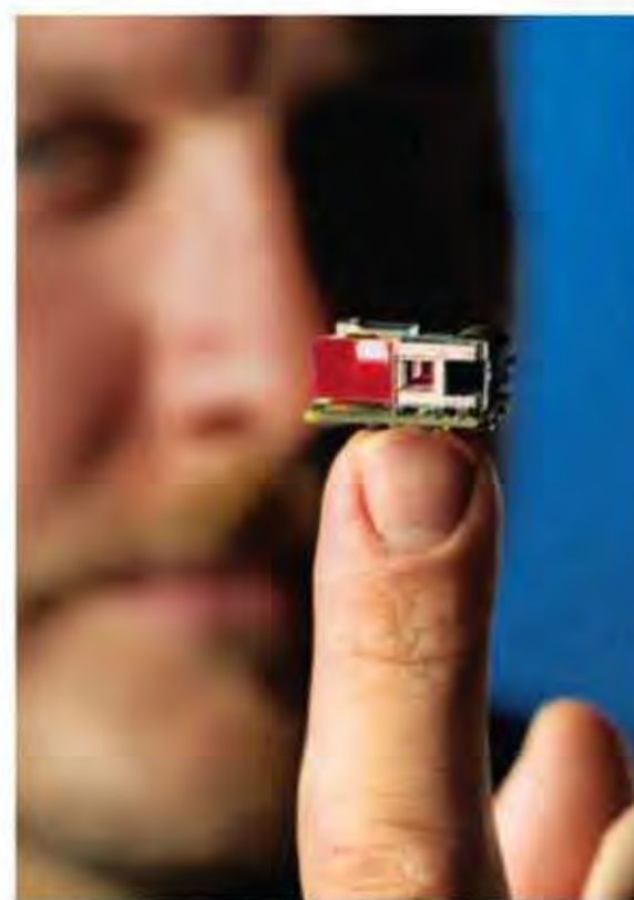
THANKS TO TINY MEMS —micro-electro-mechanical systems—laser scanners read bar codes 40 times faster.
