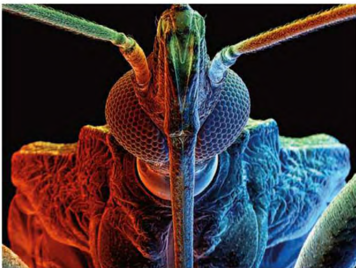
A SCANNING ELECTRON MICROSCOPE creates images of minuscule objects, like an insect’s face (above), by shooting a beam of electrons and collecting those that scatter back from the specimen’s surface. The instrument changes light into electric current and amplifies it by a factor of 10,000 or more.
