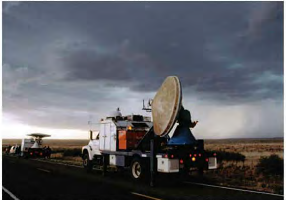
A DOPPLER RADAR ANTENNA tracks storms in the Texas Panhandle. Weather radar tools sense precipitation's intensity and motion; the information is projected onto maps for the general public, using colors to distinguish different types of precipitation.
