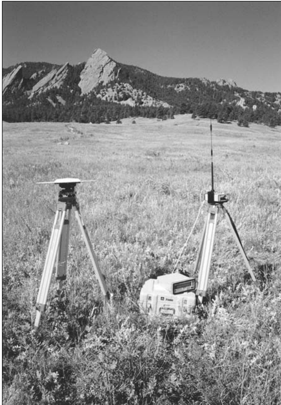
Figure 8-1: A typical GPS receiving station.
