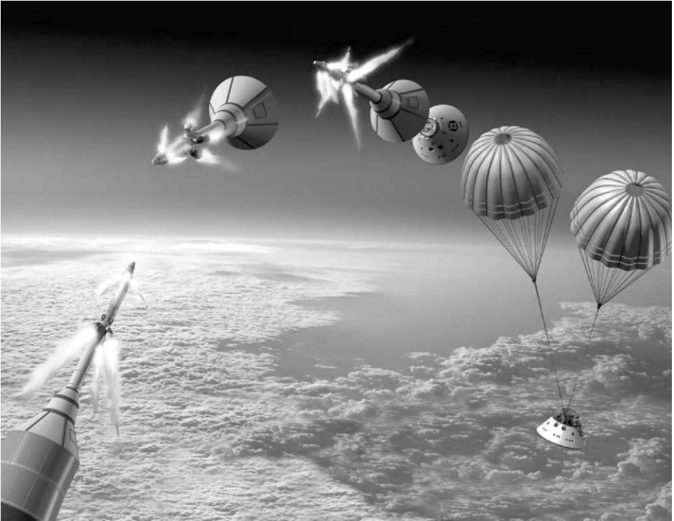
Figure 6.8 Ares I Launch Abort System. (NASA.)
