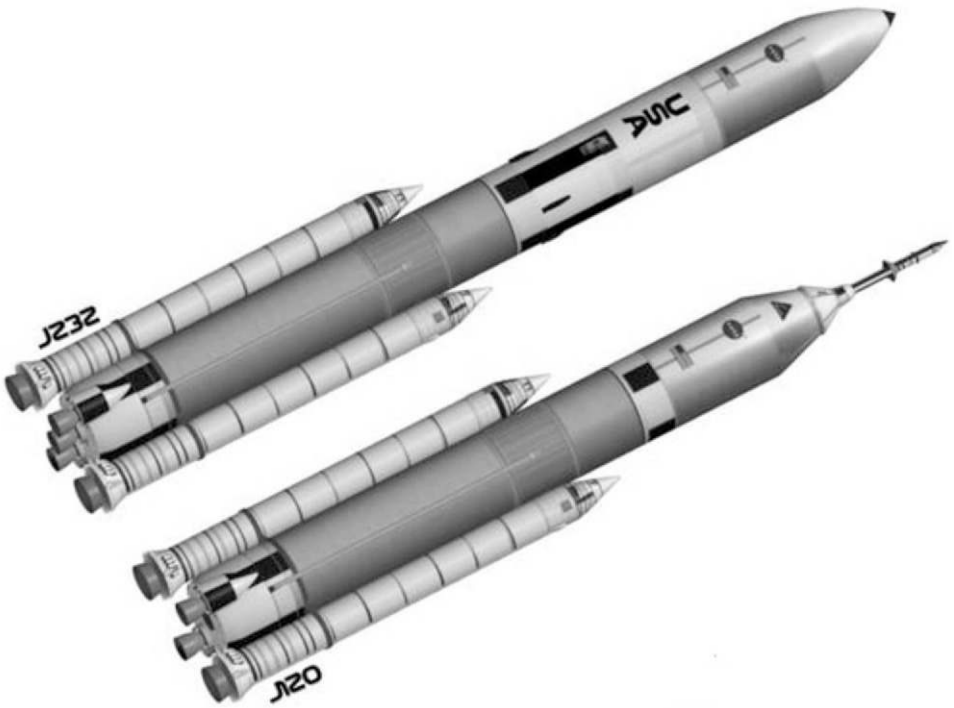
Figure 3.20 DIRECT 2.0 Jupiter 120 and 232 launch vehicles. (António H.F. Maia/DIRECT.)
