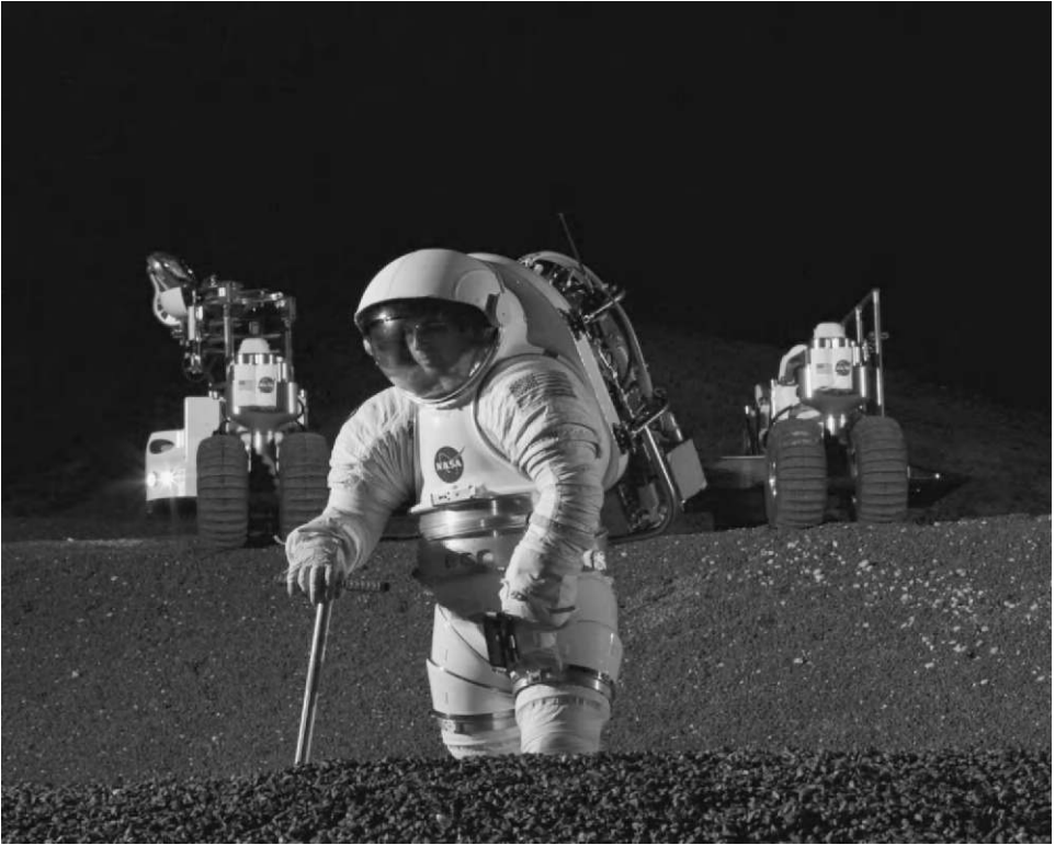
Figure 10.1 Spacesuit engineer Dustin Gohmert simulates work in a mock crater of JSC's Lunar Yard wearing the Mark III spacesuit. (NASA.)
