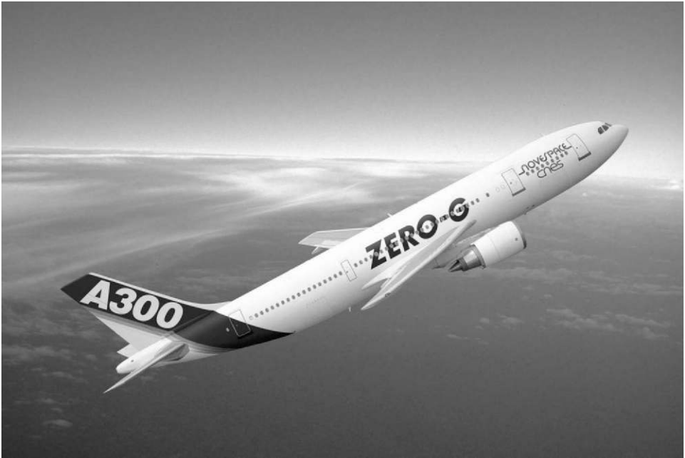
Figure 7.1 The Airbus A300 performing parabolic flight. (Novespace.) See Plate 11 in color section.
