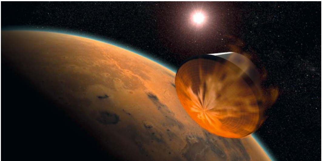
PLATE 5 Aerocapture is a flight maneuver used to insert a spacecraft into orbit using the atmosphere as a brake. The atmosphere creates friction, used to slow the vehicle, transferring the energy generated by the vehicle's high speed into heat. The maneuver enables quick orbital capture without the requirement for heavy loads of propellant. (NASA.)
