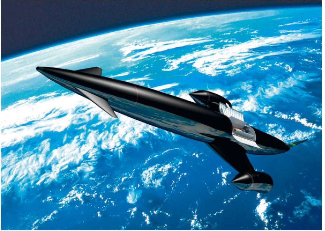
PLATE 4 The Skylon Single-Stage-to-Orbit (SSTO) spaceplane in orbit. (Adrian Mann, Reaction Engines Limited.)
