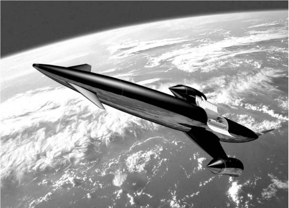
Figure 3.5 The Skylon Single-Stage-to-Orbit (SSTO) spaceplane in orbit. (Adrian Mann, Reaction Engines Limited.) See Plate 4 in color section.
