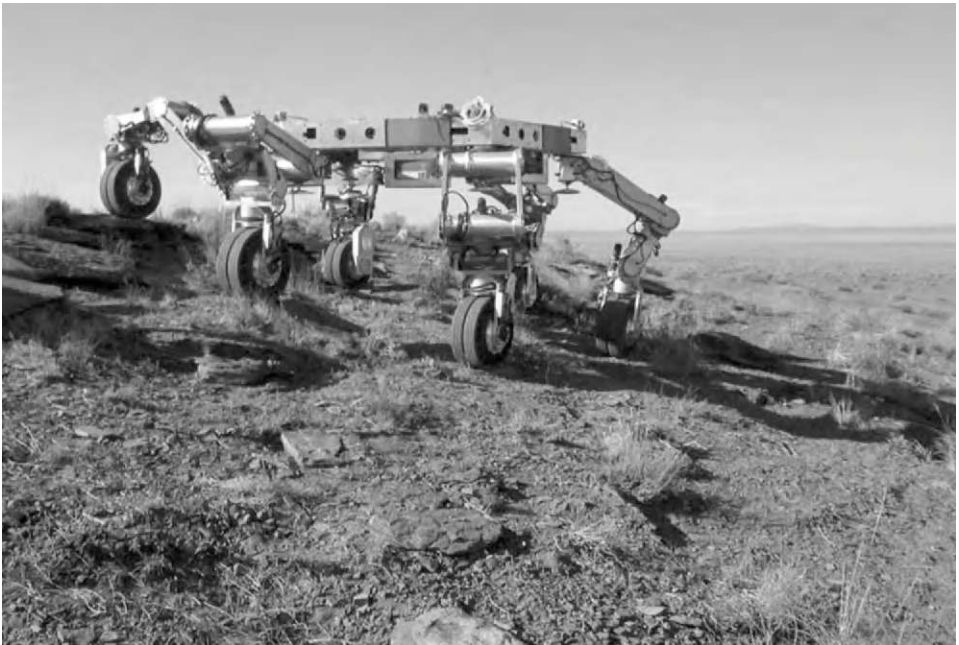
Figure 10.6 The All-Terrain Hex-Limbed Extra-Terrestrial Explorer (ATHLETE) will provide multi-wheeled dexterity to Martian surface operations. (NASA.)
