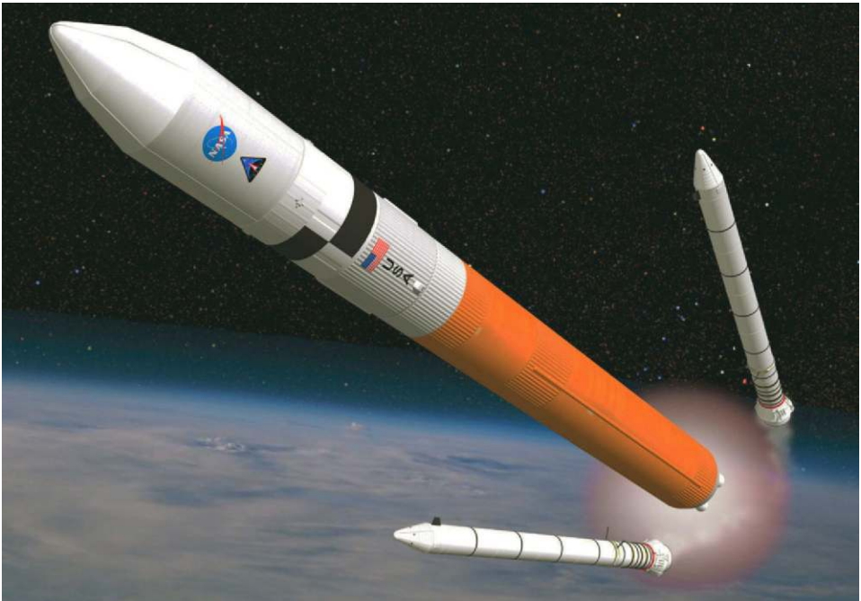
PLATE 3 NASA's Ares V is a two-stage, vertically stacked launch vehicle capable of carrying 188 metric tonnes to low-Earth orbit. For the initial insertion into Earth orbit, the Ares V first stage utilizes two five and a half segment reusable solid rocket boosters derived from the Space Shuttle's solid rocket boosters. In the Mars Direct architecture, the Ares V would deploy a forty-tonne cargo payload into a direct trans-Mars trajectory. (NASA.)
