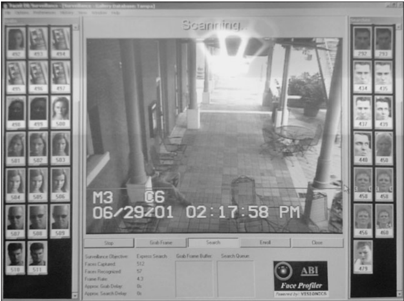
A screen image of the Visionics FaceIt system scanning for faces from a video feed. Courtesy Tampa Tribune . Reprinted with permission.
