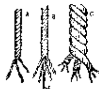
Cordage 1214-MN A Hawser-laid Rope; B Shroud-laid Rope (a) Heart; C Cable-laid Rope
