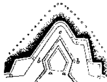
Bastion 341R-WN a Curtain angle; b Shoulder c Salient angle; aa Gorge; ab Flank; ad Curtain; bc Face
