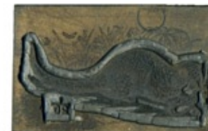
The circle at the top of this engraving is a plug that was put in the block to repair an imperfection before the engraving was done.
