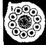
Submarine Telegraph Cable 2412-WN a Copper wires with sheaths of Gutta- percha, Yarn, Iron wire, etc. b Trans- verse Section of same
