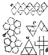
Stereography a Tetrahedron; b Hexahedron; c Octahedron; d Dodecahedron; e Icosahedron 3227-W4
