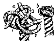
Wall Knot 2715 WN a. Strands arranged to form b. completed knot
