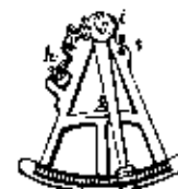
Hadley's Quadrant 2871R-W4 h Horizon-glass; i Index-glass; s Sigit
