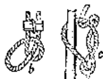
Hitches 1870R-MN b Half Hitch; c Timber Hitch
