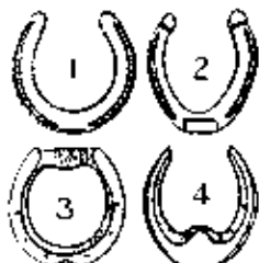
Horse Shoes 6426R-ML 1 Plain Shoe; 2 Shoe with toe & heel calks; 3 Unlucky horse shoe; 4 Lucky horse shoe.
