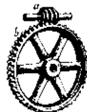
Worm Gearing a Worm Gear b Worm Wheel 4151R-MN
