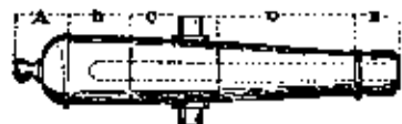
Cannon 455-W4 (Muzzle-loading) A Formerly called Cascabel; B First Reinforce; C Second Reinforce; D Chase; E Swell of Muzzle
