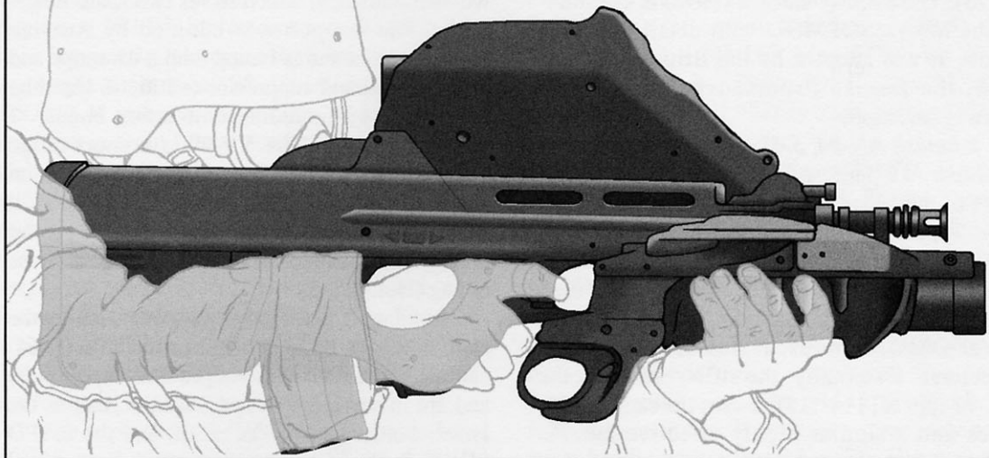
FN F2000 assault rifle with LG1 under-barrel grenade launcher and integrated fire control system.
