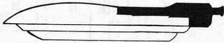
Schematic showing streamlining and size relationship of drives (dark area) to overall ship size.
