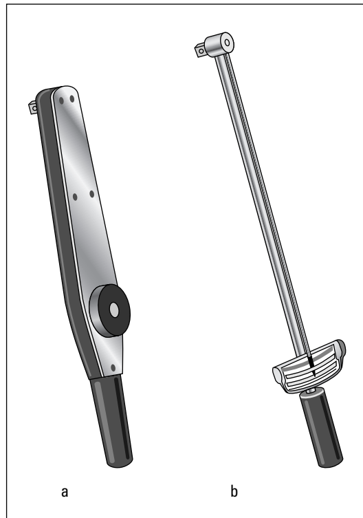
Figure 3-7: A dial torque wrench (a) and a deflecting beam torque wrench (b).
