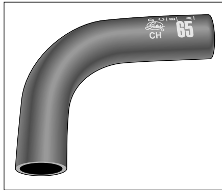
Figure 12-4: A preformed top radiator hose.
