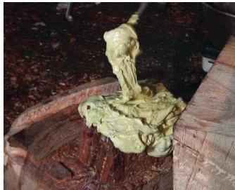
Melting waste plastic to create my toaster case
