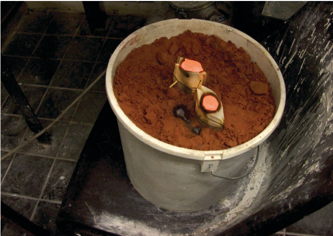
Casting the three copper pins in cuttlefish shell moulds
