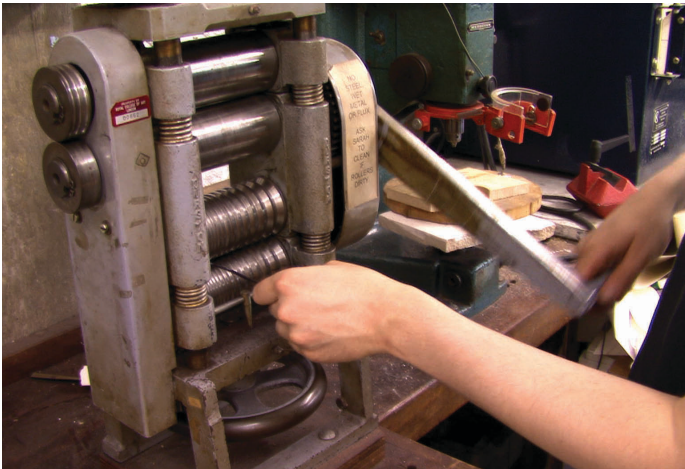
Rolling out the wire
