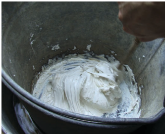
Melting waste plastic to create my toaster case
