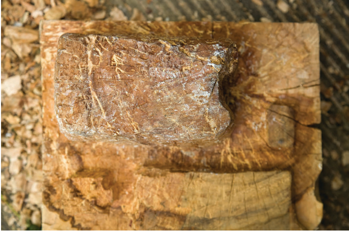
The male part of the mould, or the "plug member"
