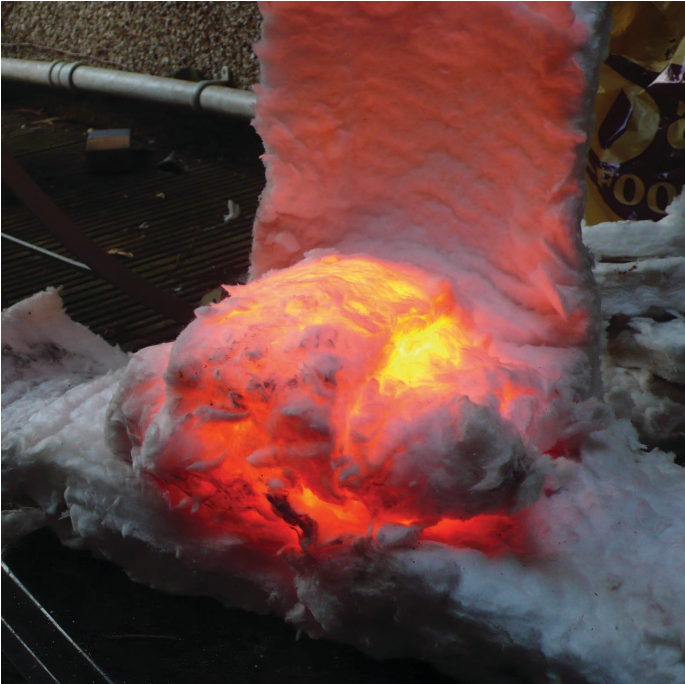
A success! The crucible glowing white hot in its partially unwrapped insulation
