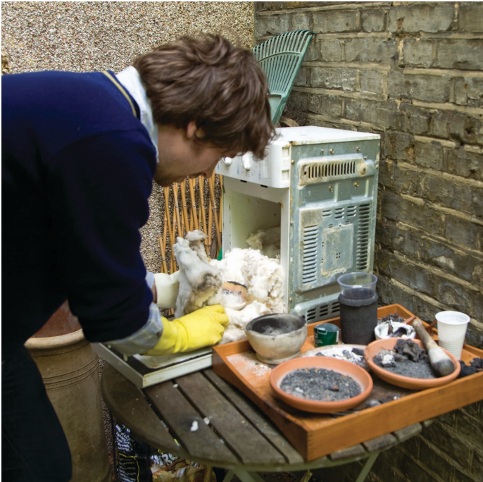
Insulating the crucible with ceramic wool to maximise the heat gained
