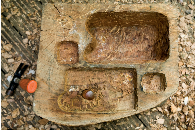
The female part of the mould, or the “mould cavity”
