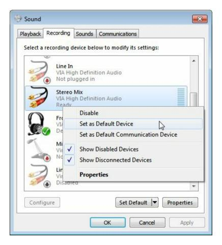
Now stereo mix is enabled and ready to use! Any audio coming through your speakers will also be piped to stereo mix which can be selected as an audio piping source in most programs that require one.
