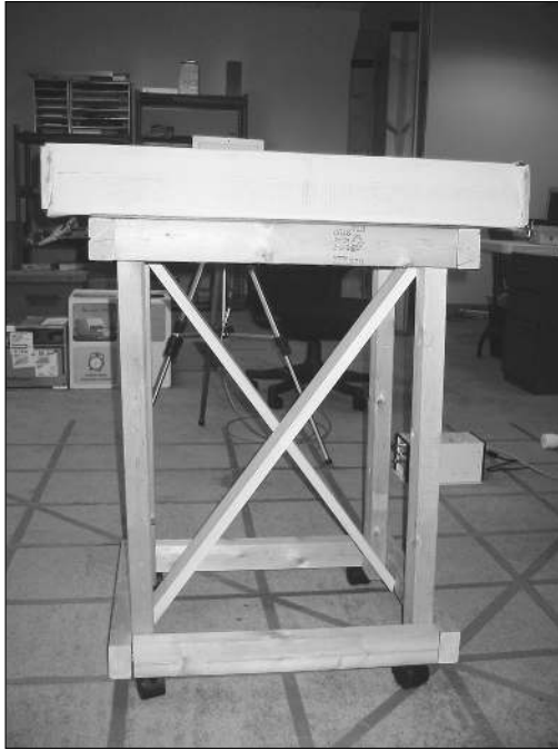
Figure 8-5: A SKU testing bench made of kiln-dried lumber.
