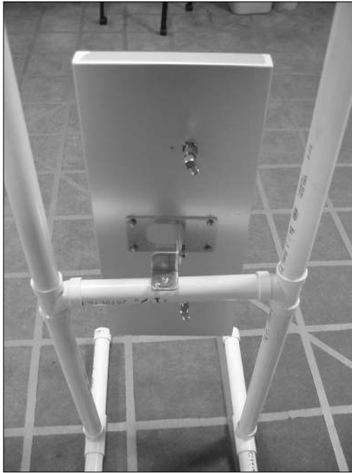
Figure 8-4: A home-made, freestanding PVC antenna rack.
