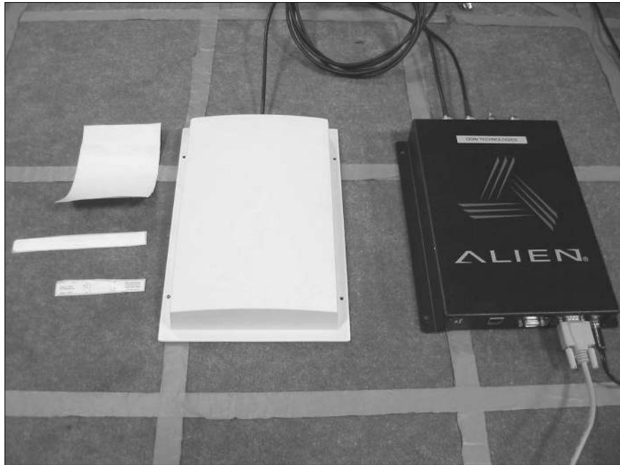
Figure 1-1: An Alien reader, a single antenna, and three types of Alien Class 1 tags.
