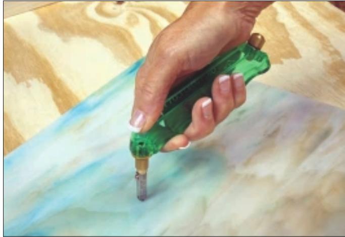
Figure 2-3: A pistol-grip cutter and the proper way to position it in your hand.
