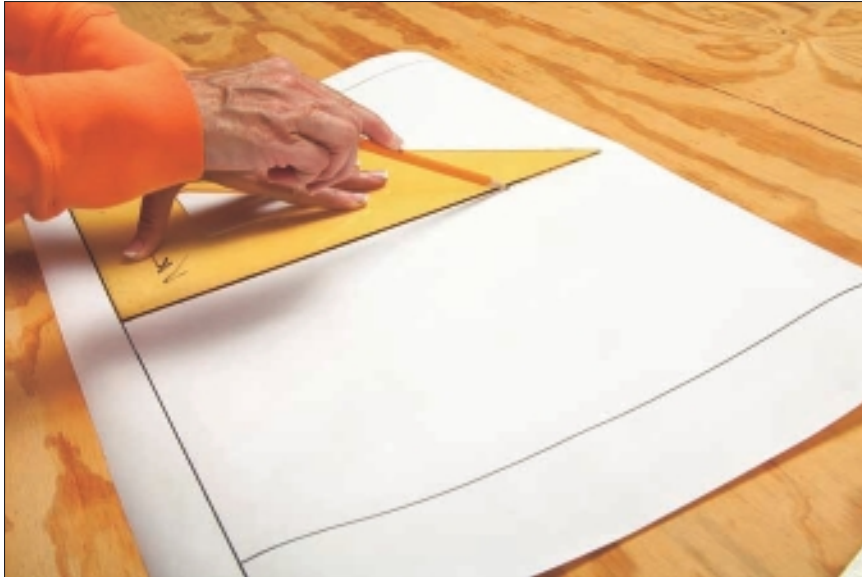
Figure 4-6: Establishing the middle design line.
