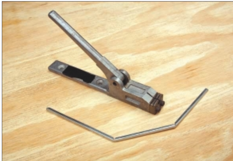
Figure 2-23: A notcher with examples of came cuts.
