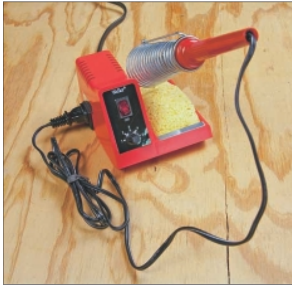
Figure 7-1: Setting up a rheostat- controlled iron for a copper-foil project.
