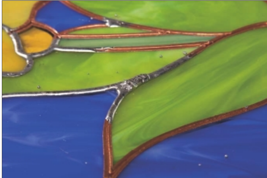
Figure 7-12: Common soldering imperfec- tions caused by popping flux.
