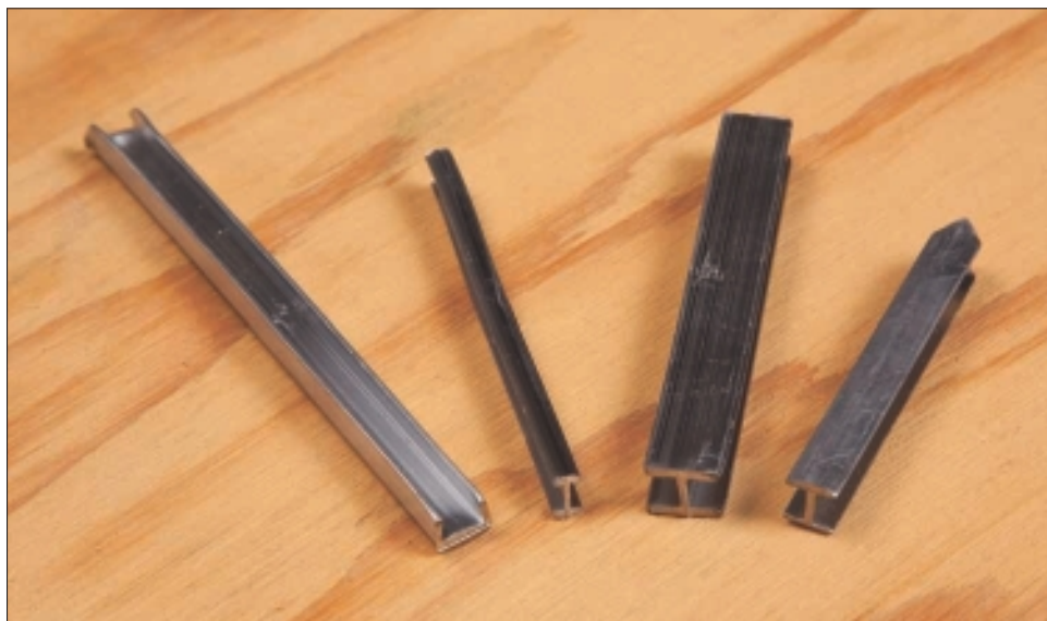
Figure 9-1: Different came profiles and sizes.
