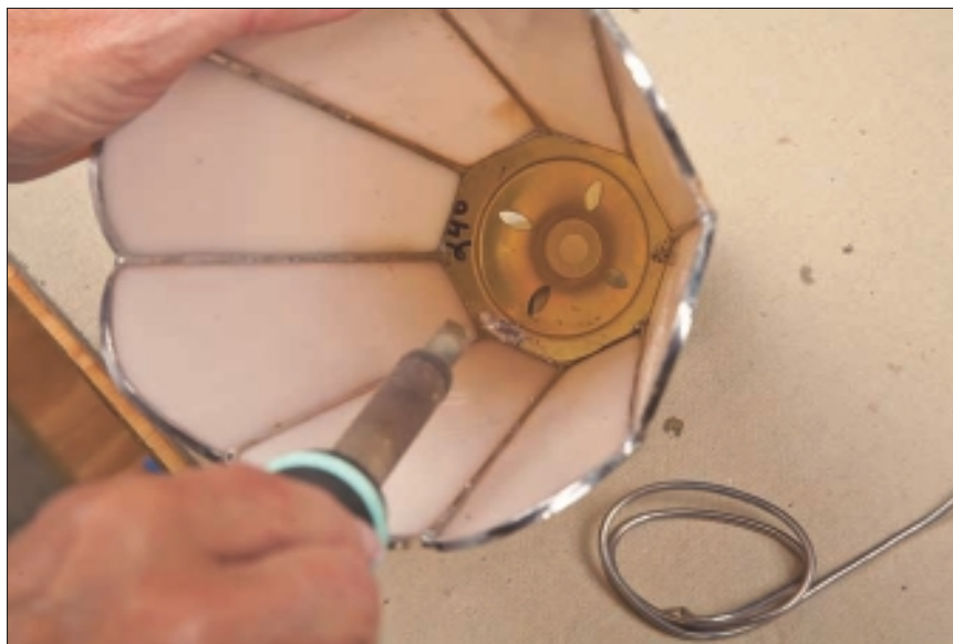
Figure 11-14: Tack soldering the cap to the top edge of the glass.
