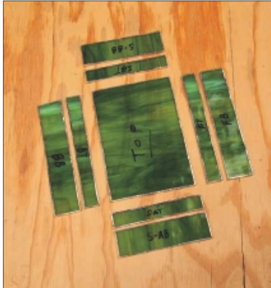
Figure 10-15: Foiled and tinned box pieces.
