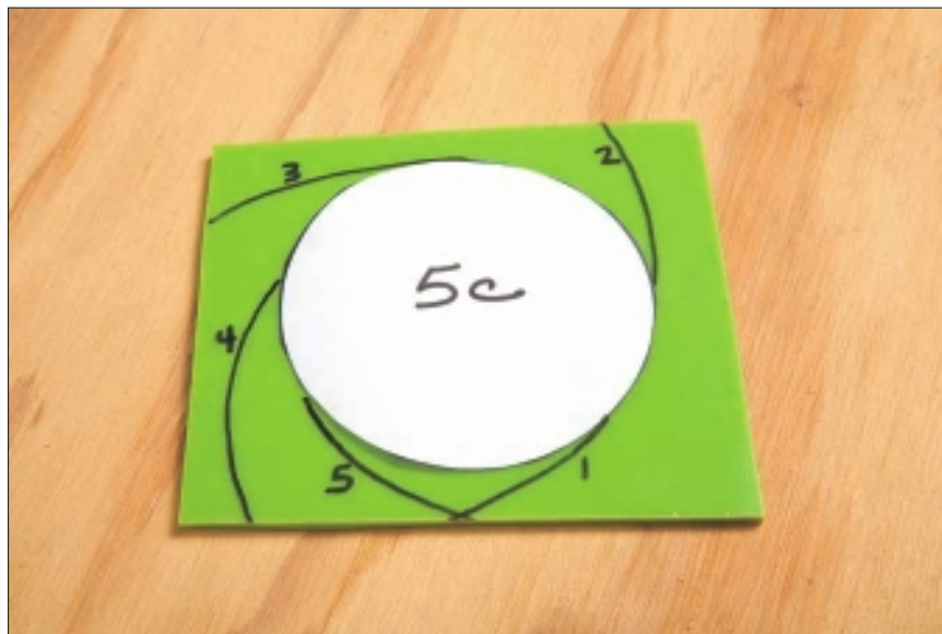
Figure 5-20: Making relief score lines around a circle pattern.
