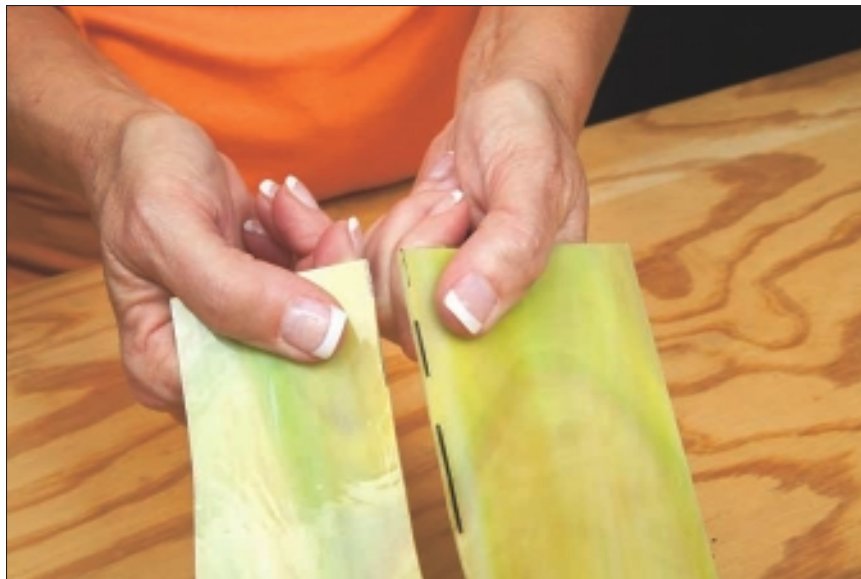
Figure 5-8: Rotating your hands to break the glass.
