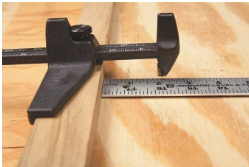
Figure 10-10: Setting the cutting wheel at 2 inches.
