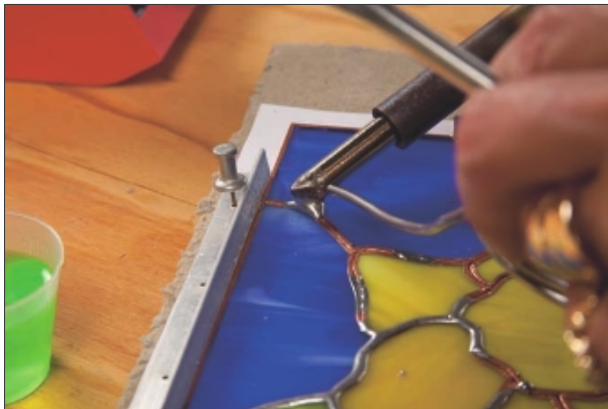
Figure 7-8: Molten solder ball under the soldering tip.
