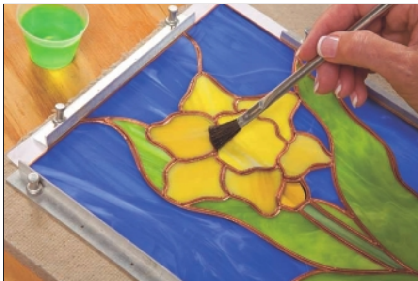
Figure 7-4: Applying flux to a copper-foil project.
