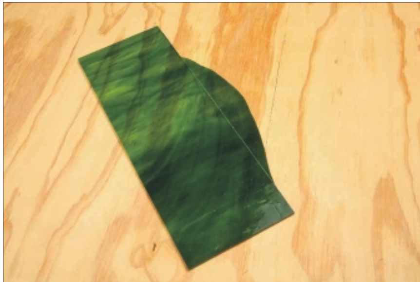
Figure 5-15: A bad break and run.
