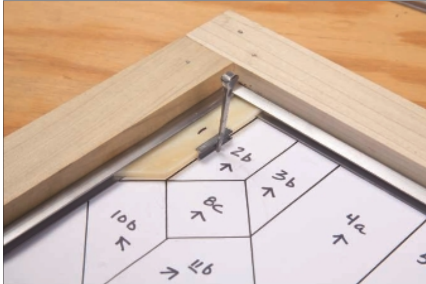
Figure 9-21: Securing the first glass piece in position with a spacer and a horseshoe nail.
