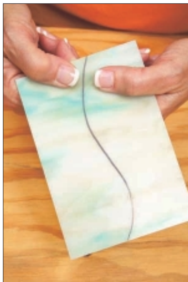
Figure 5-14: Breaking glass along a curved score line.
