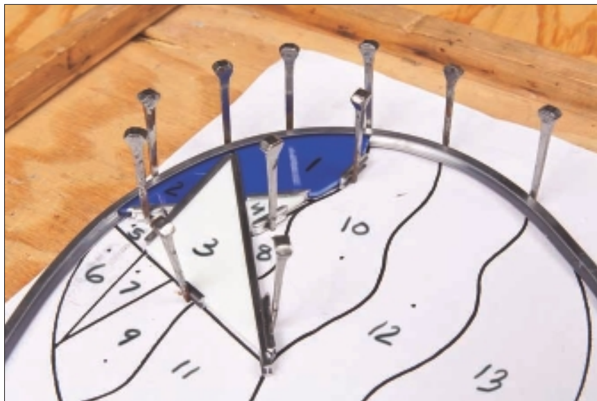
Figure 9-31: Partially leaded round panel.
