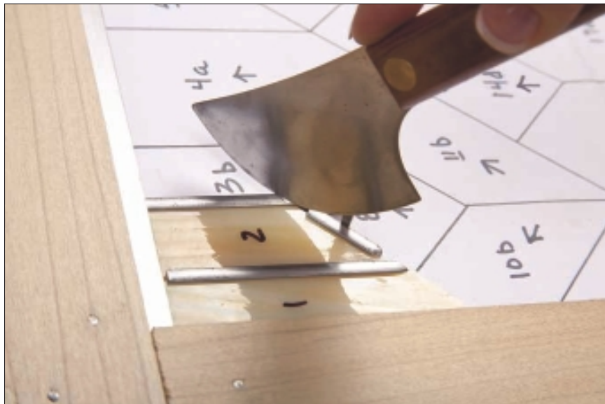
Figure 9-22: Using a lead knife to indicate where to trim the lead came and the angle of the cut.
