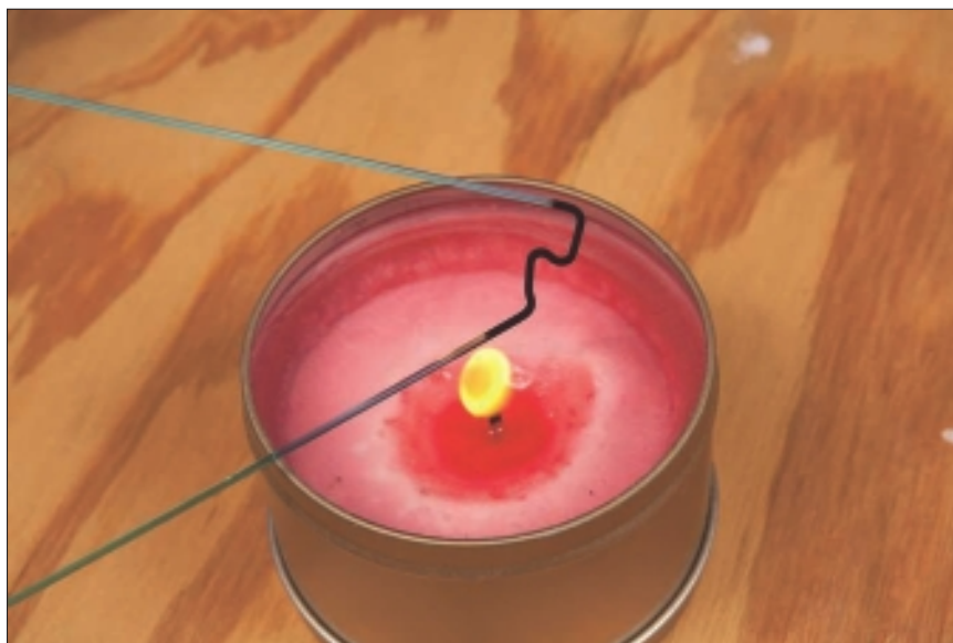
Figure 14-5: Bending a glass stringer over a candle flame.
