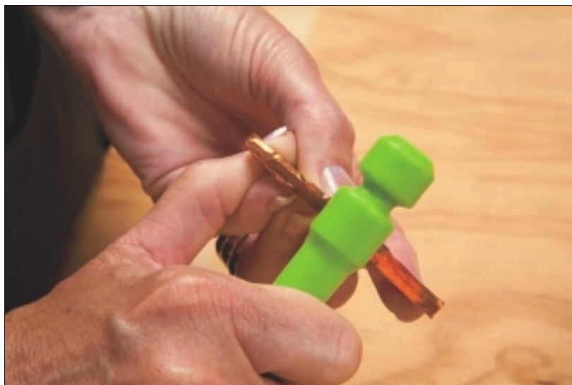
Figure 8-7: Burnishing the foil to the glass's edge.
