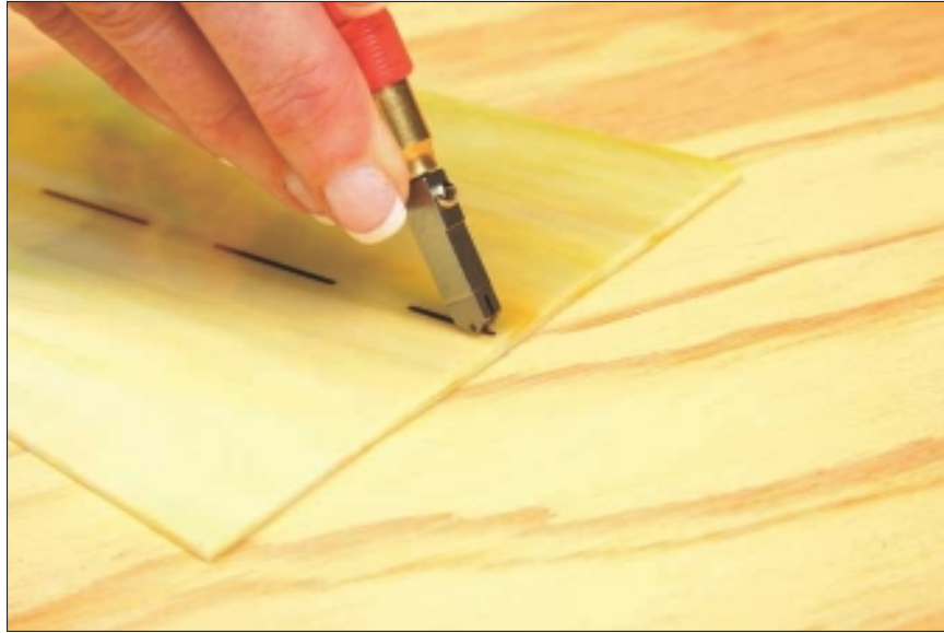
Figure 5-6: Ending the score before you come to the edge of the glass.
