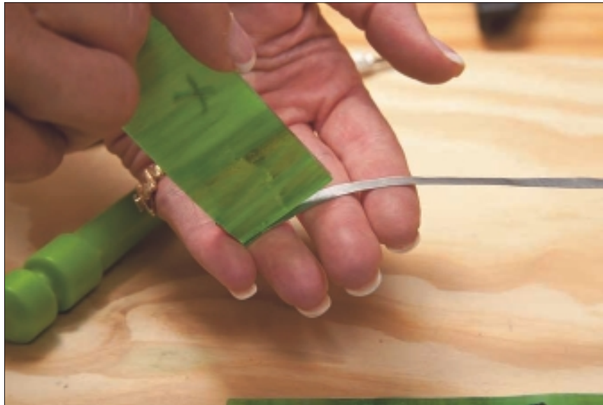
Figure 10-14: Applying copper foil.
