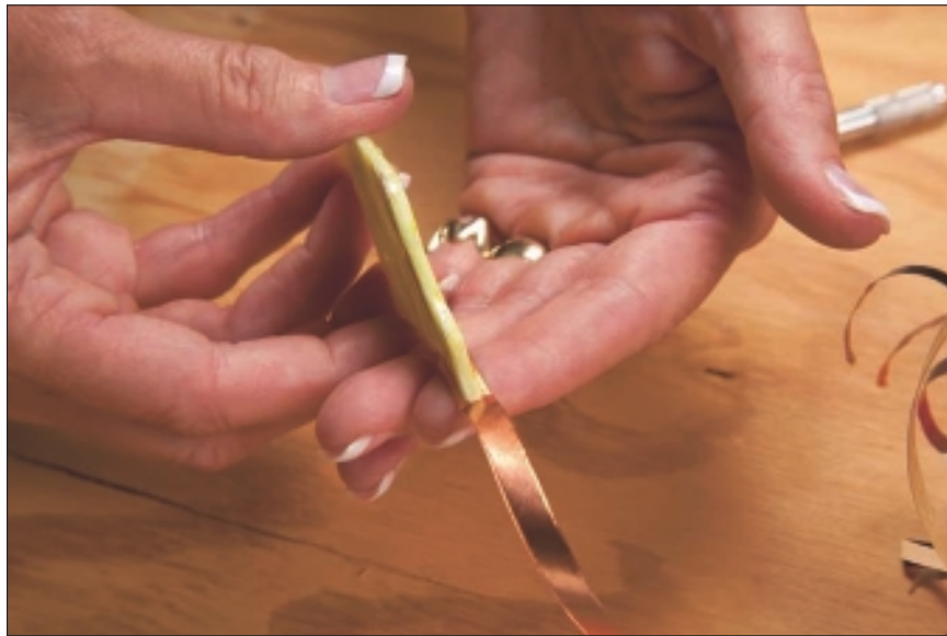
Figure 8-6: Centering a glass piece on the foil.
