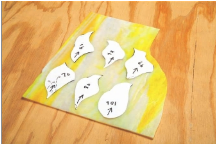
Figure 5-18: Laying out your pattern templates.
