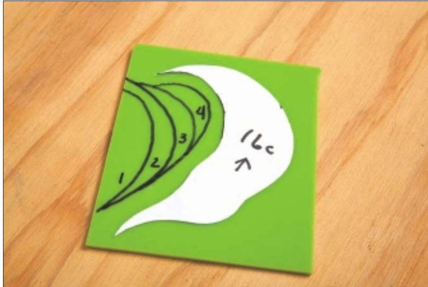
Figure 5-19: Making relief cuts when cutting curves.
