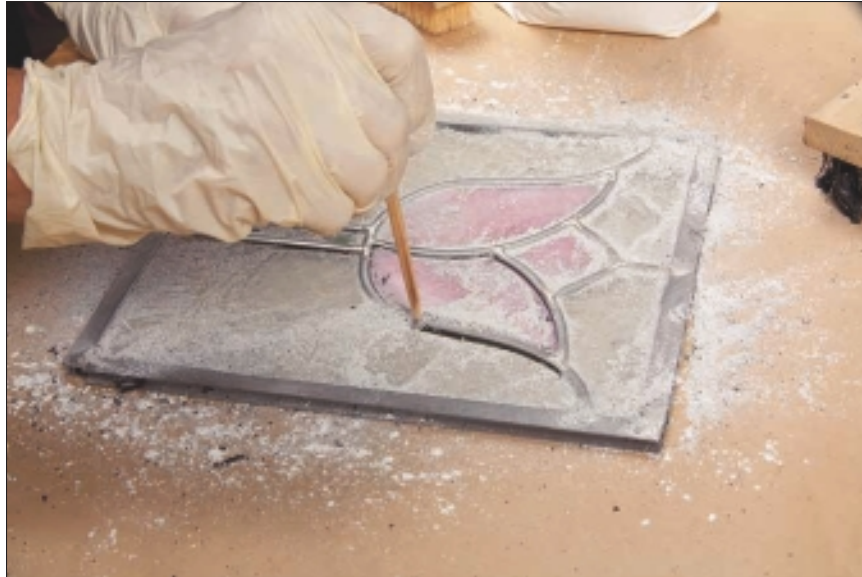
Figure 9-17: Removing any remain- ing cement with a craft stick.
