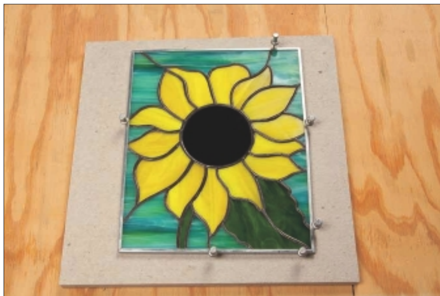
Figure 8-26: Panel with zinc frame ready for soldering.
