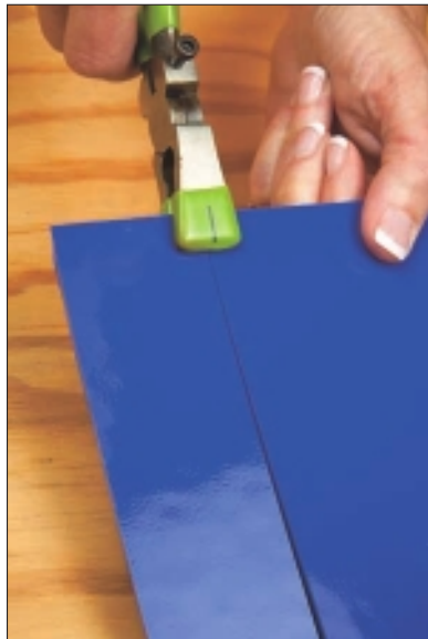
Figure 5-12: Completing the break with running pliers.
