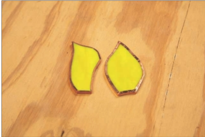
Figure 8-2: Comparing proper-sized foil (left) and too-large foil (right).
