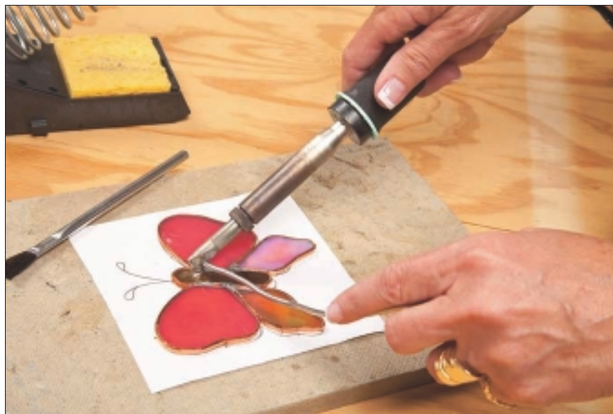
Figure 8-12: Correct way to hold your soldering iron.
