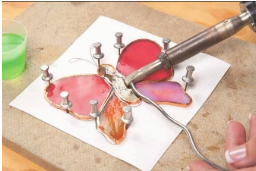
Figure 8-11: Position of solder and iron when tack soldering.
