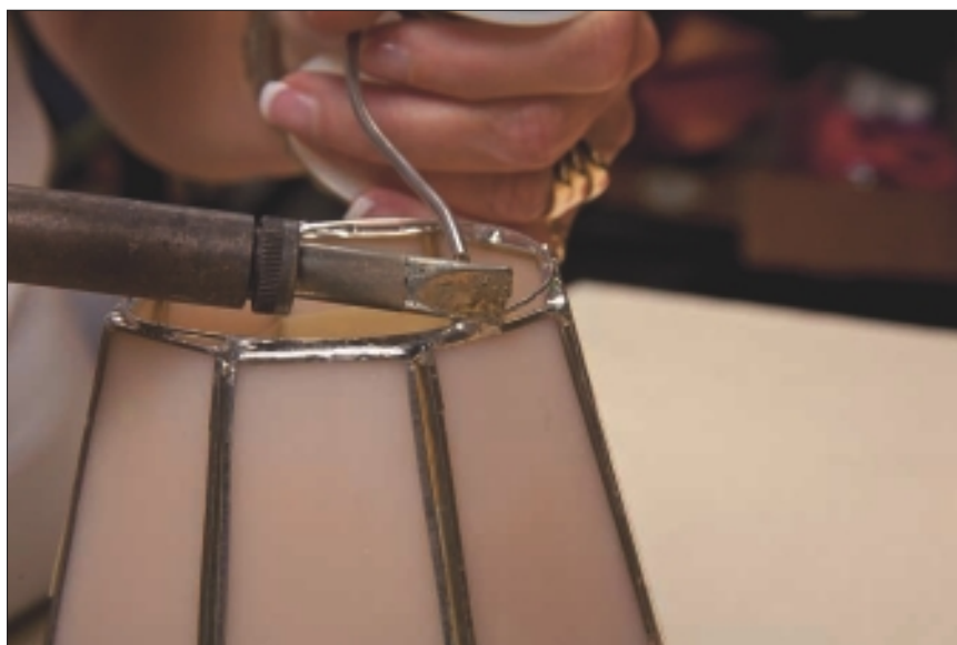
Figure 11-9: Covering the support wire with solder.
