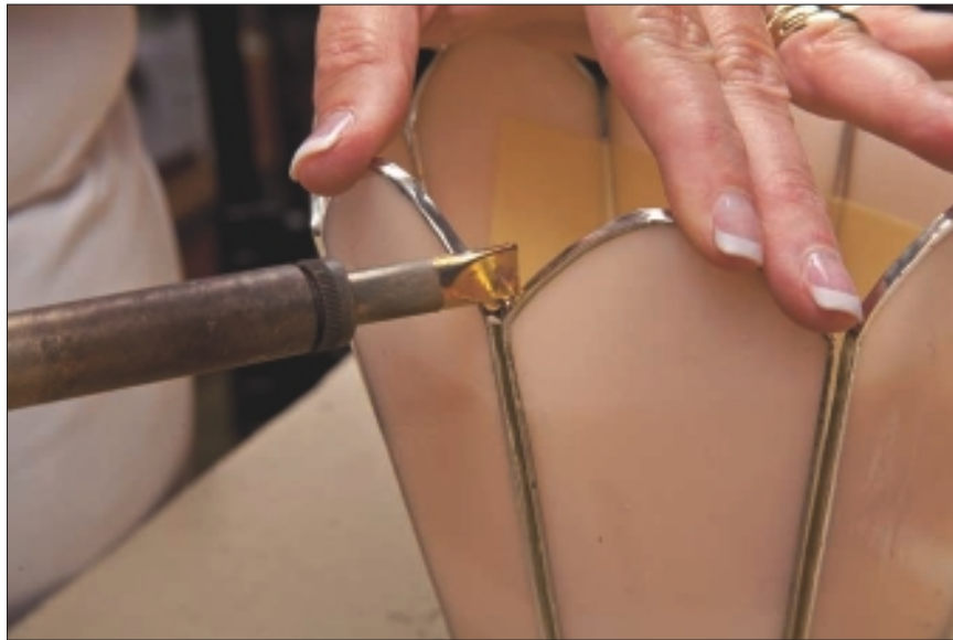
Figure 11-10: Tack soldering the bottom panel intersections together.
