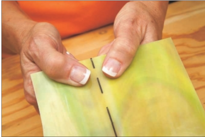
Figure 5-7: Getting your hands in the right position to break the glass.
