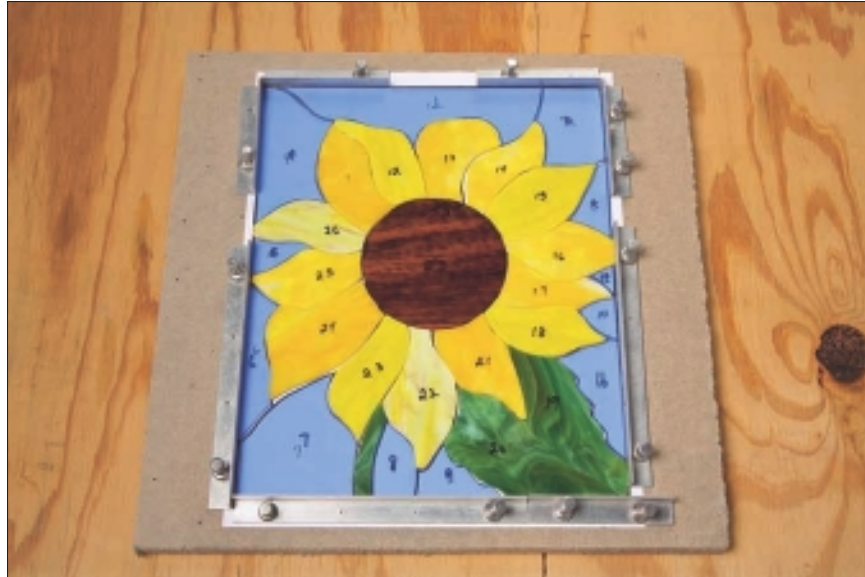
Figure 8-1: A copper-foil project that's fitted to the pattern and ready for foil.
