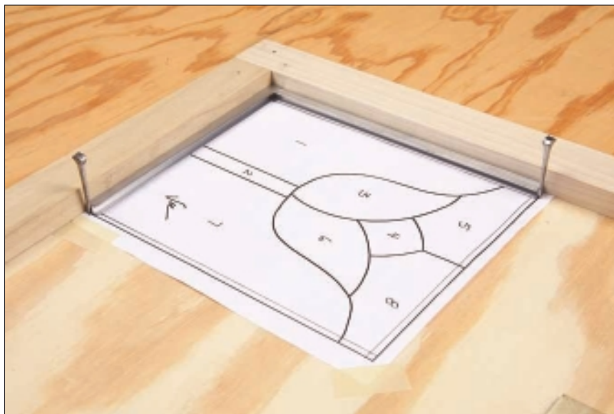
Figure 9-7: Securing lead comes around your pattern on the work board.
