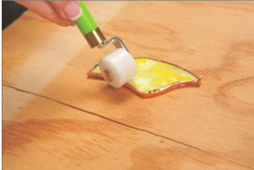
Figure 8-9: Burnishing the foil tightly to the glass's sides.
