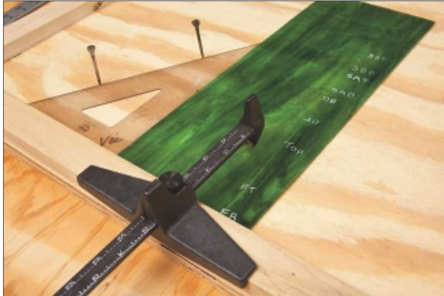
Figure 10-9: Glass set up and ready for stripping.
