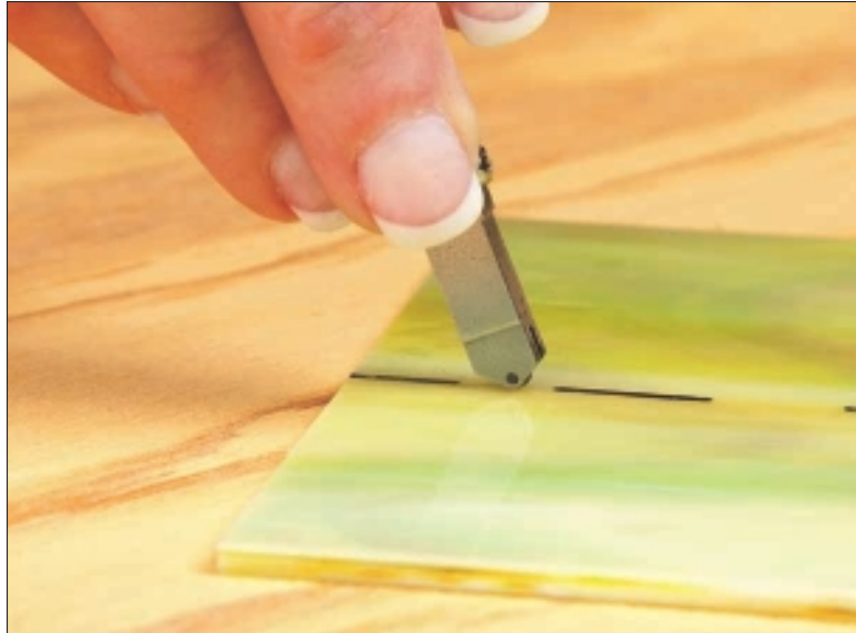
Figure 5-4: Positioning your glass cutter for the score.
