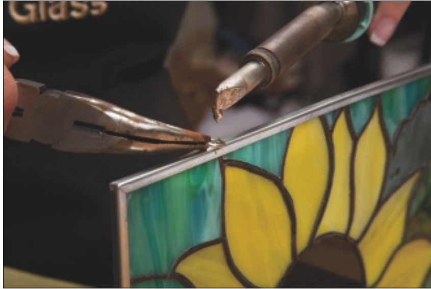
Figure 8-27: Attaching wire rings to the frame.
