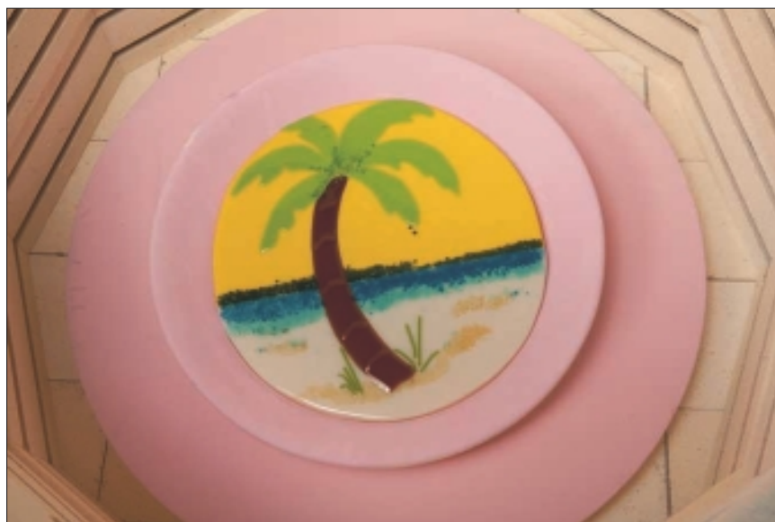
Figure 16-12: Getting the glass and mold ready for the second firing.
