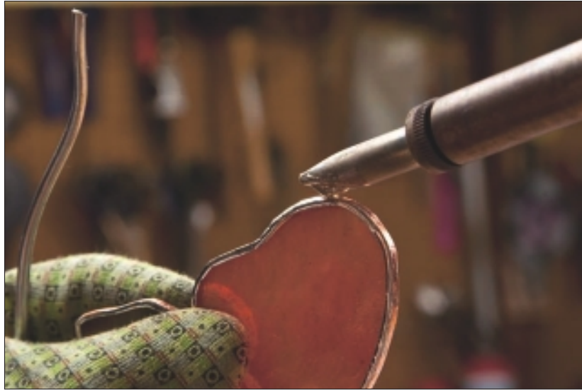
Figure 8-16: Holding the project while creating a frame with solder.
