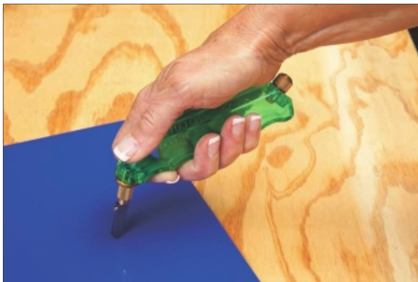
Figure 5-2: Holding a pistol-grip cutter.
