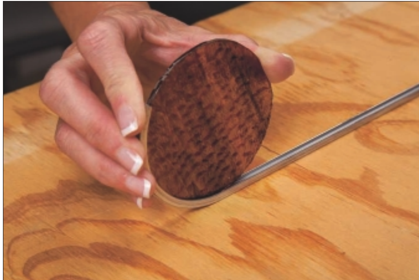
Figure 9-10: Wrapping a circle- shaped piece of glass in lead came.
