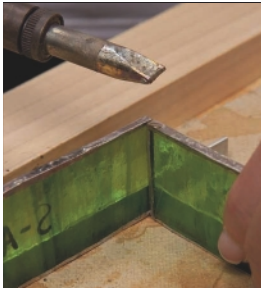
Figure 10-16: Tack soldering the box sides together.
