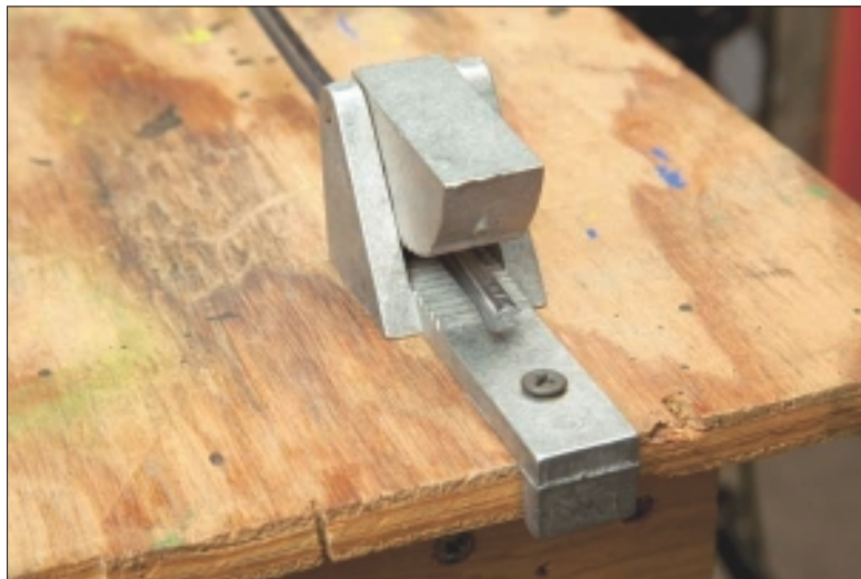
Figure 2-17: Lead vise mounted on a worktable.
