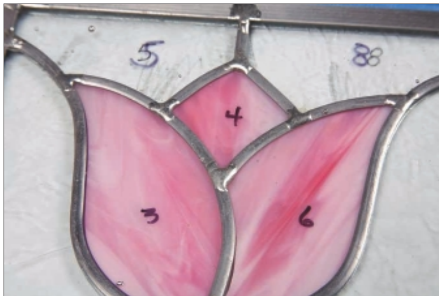
Figure 9-13: Examples of perfectly sized solder joints.
