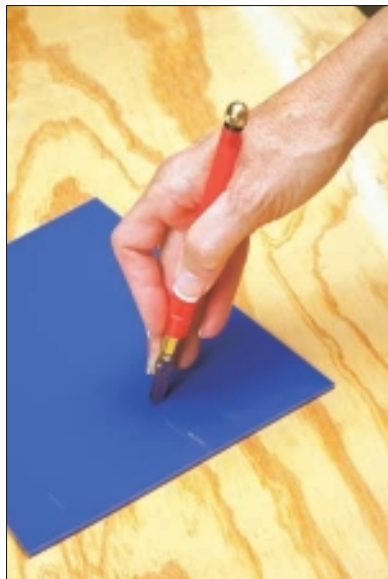
Figure 5-1: Holding a barrel cutter with extended fingers.
