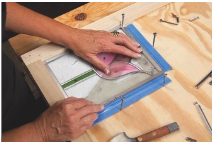
Figure 9-11: Checking a leaded panel for square corners.
