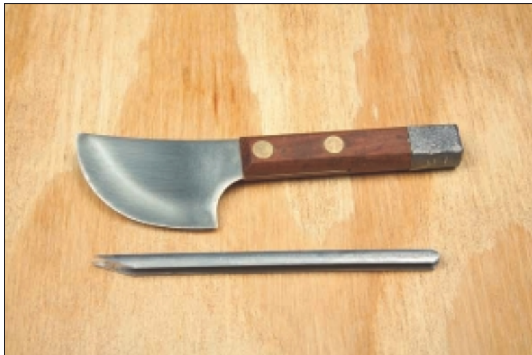
Figure 2-18: A lead knife and a cut came.
