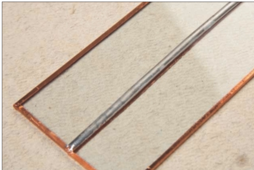
Figure 8-4: Cathedral glass foiled with copper- backed foil.
