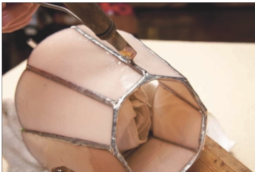
Figure 11-12: Soldering the seams on the out- side of your lamp.
