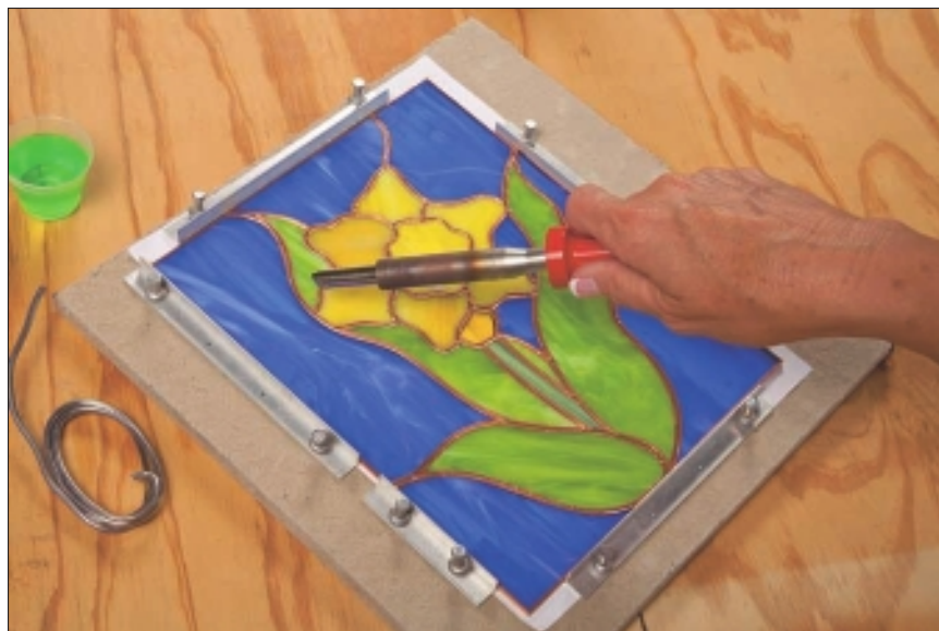
Figure 7-2: Holding your soldering iron the right way.
