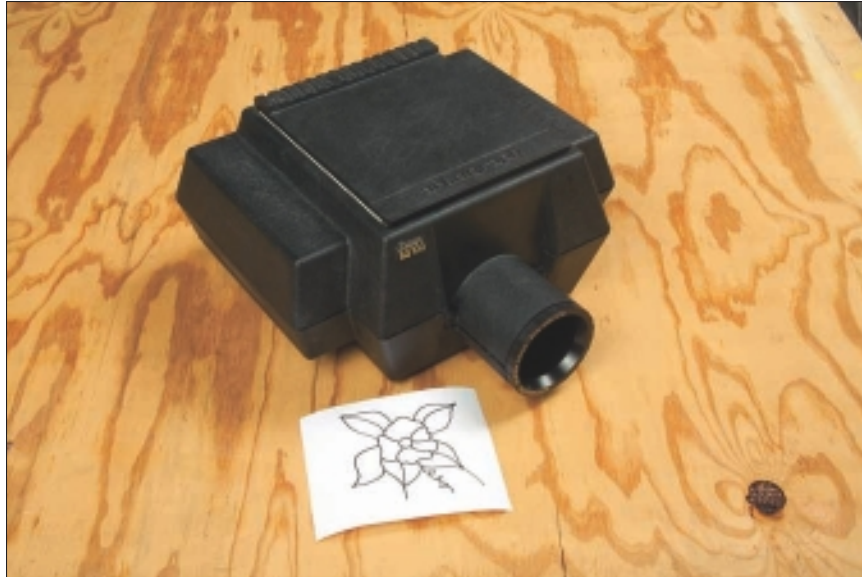
Figure 4-2: An opaque projector and design to be enlarged.
