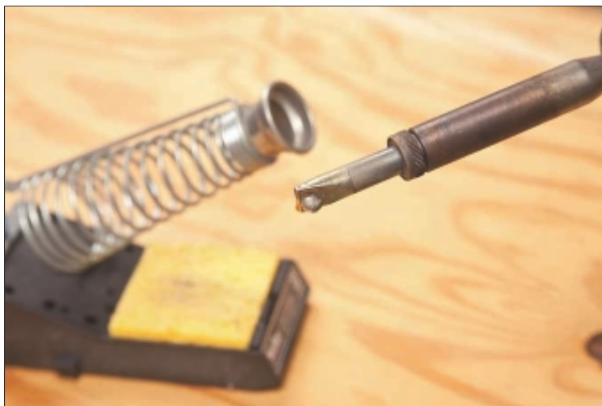
Figure 8-15: A drip of solder clinging to an iron tip that's too hot.
