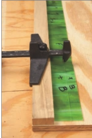
Figure 10-12: Glass strips laid out for separating the tops from the bottoms.
