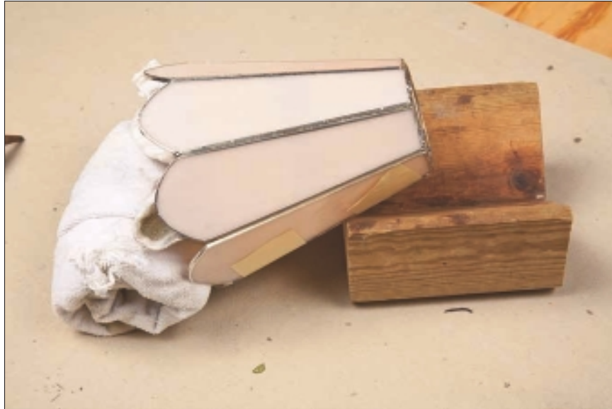
Figure 11-11: Supporting your shade's shape with wooden blocks and towels.
