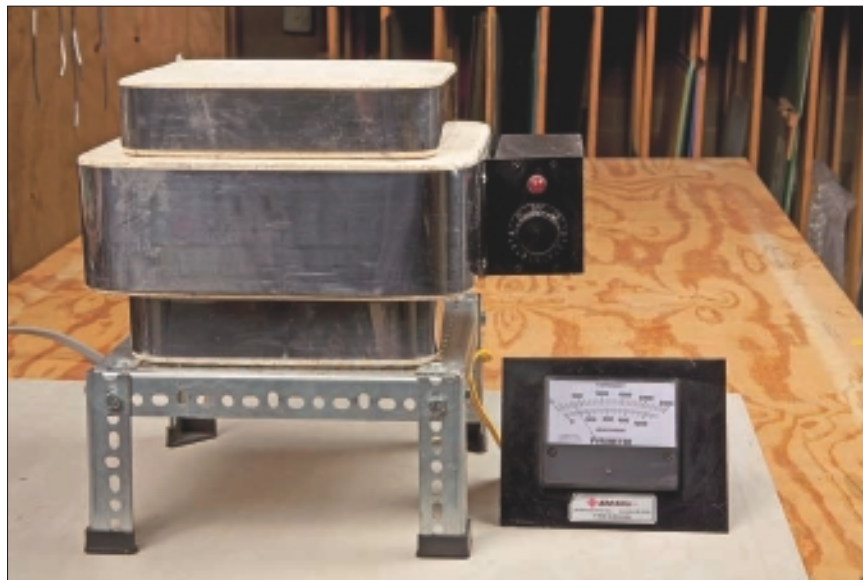
Figure 13-1: A temperature gauge mounted to the outside of a kiln.
