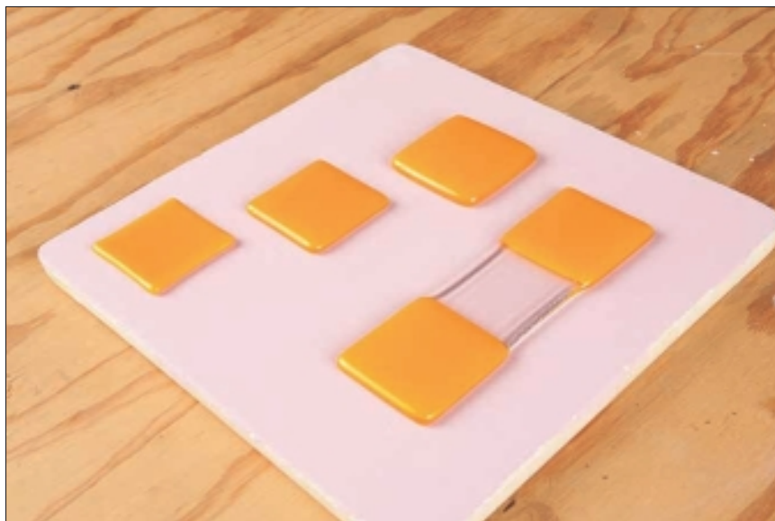
Figure 15-4: The results of test firing various layers of glass.
