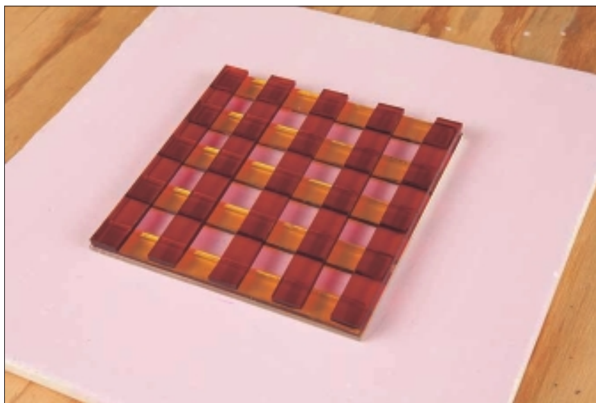
Figure 15-7: The perpen- dicular layer of glass creates the woven design.
