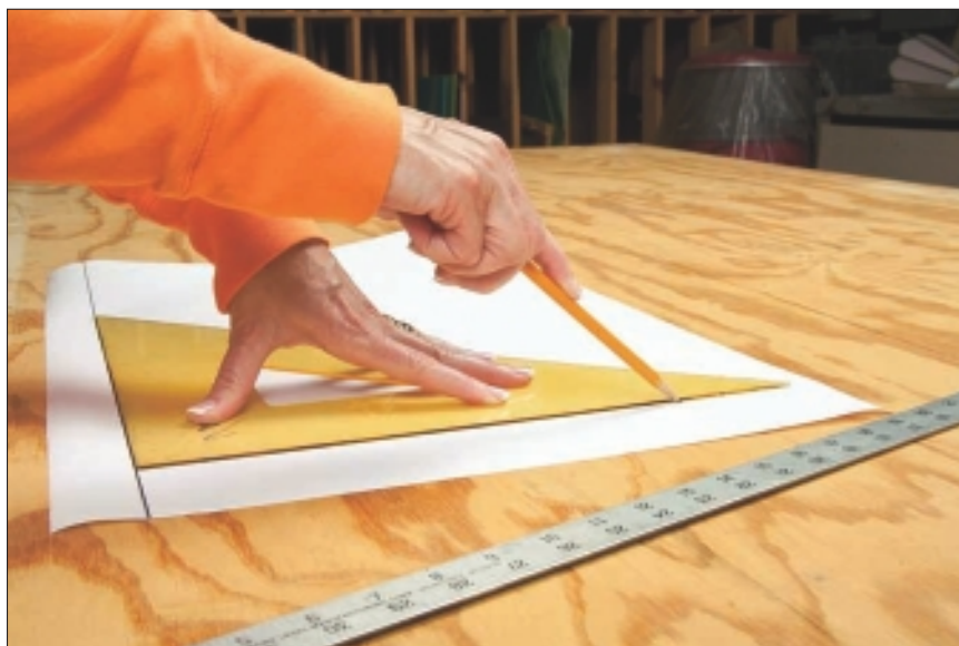
Figure 4-5: Establishing the bottom square corner of your design space.
