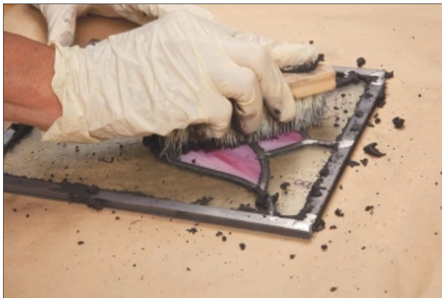
Figure 9-14: Using a natural brush to spread cement over the panel's surface.
