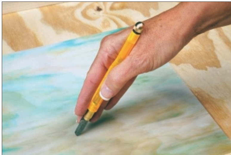
Figure 2-2: A barrel cutter and the proper way to position it in your hand.
