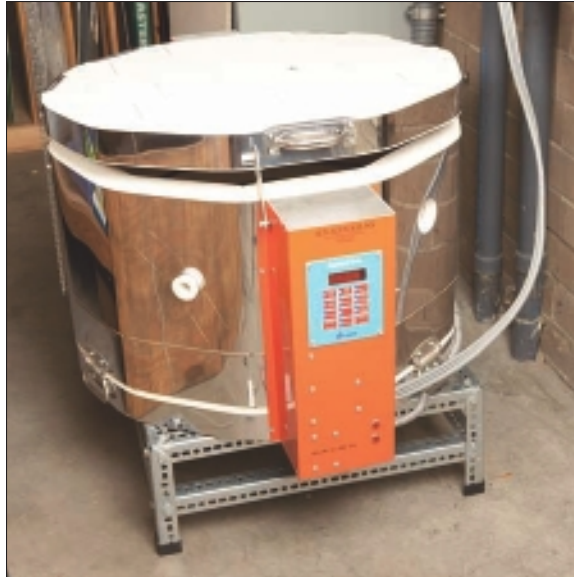
Figure 13-10: Test firing a new glass kiln.
