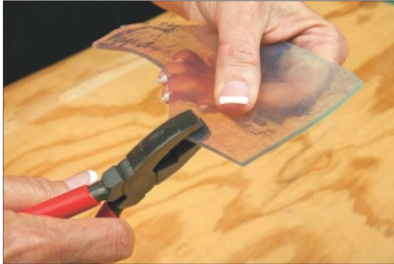
Figure 6-2: Grozing a piece of glass.
