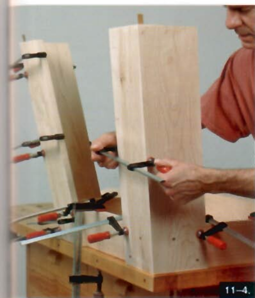
Clamping the legs (D) to the frame (A/B/C) holds them at the proper angle while you finish clamping their length.
