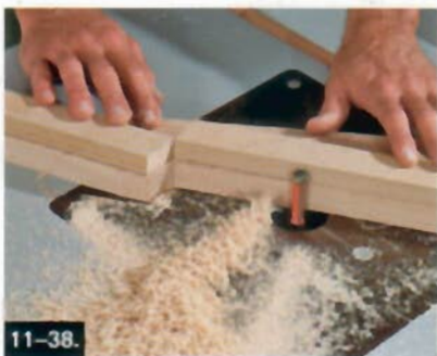
11-38. Use tape-adhered guide blocks and a flush-trim bit to rout the first leg to final shape. Then use it as your template.
