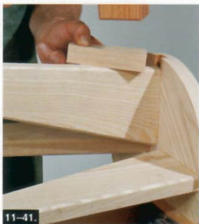
11-41. Two of the legs will have to be tapped in toward the center to make clearance for the foot ring, which installs from the top.
