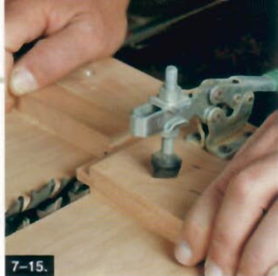
This shopmade tenoning jig features a hold-down toggle clamp. Make your own carriage-style jig, or use a miter gauge.
