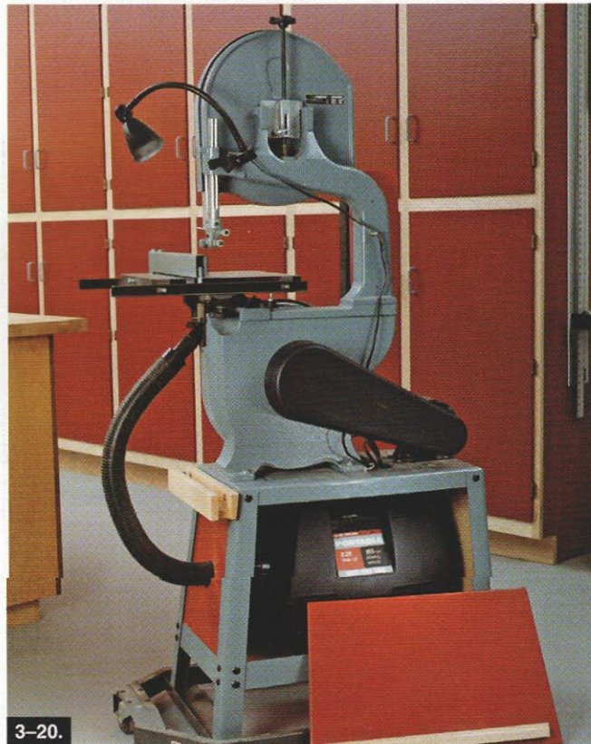
This bandsaw has a dust-collection outlet switch mounted to it and a three-outlet adapter connected to one end.
