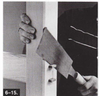
6-15. Tap the hardwood wedges into the notches. After the glue dries, trim the wedges flush with the legs.
