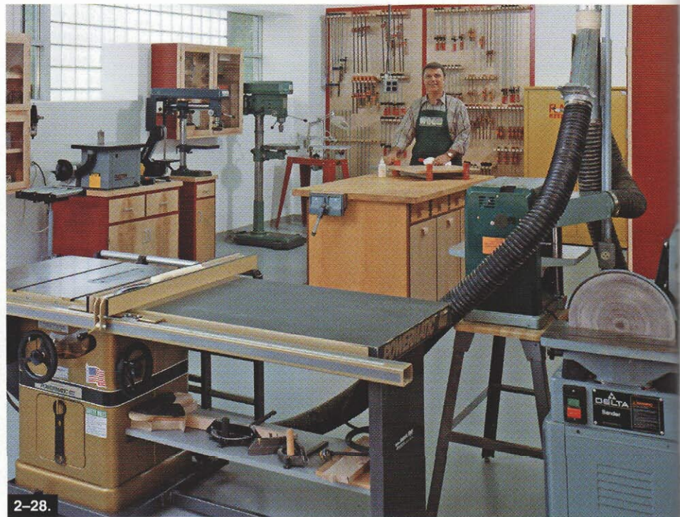
2-28. Chuck Hedlund, WOOD ® magazine's project builder, clamps an assembly together at one of the workbenches. This view looks north from the double entry doors. At right you can see the ducts and blast gates of the central dust-collection system.
