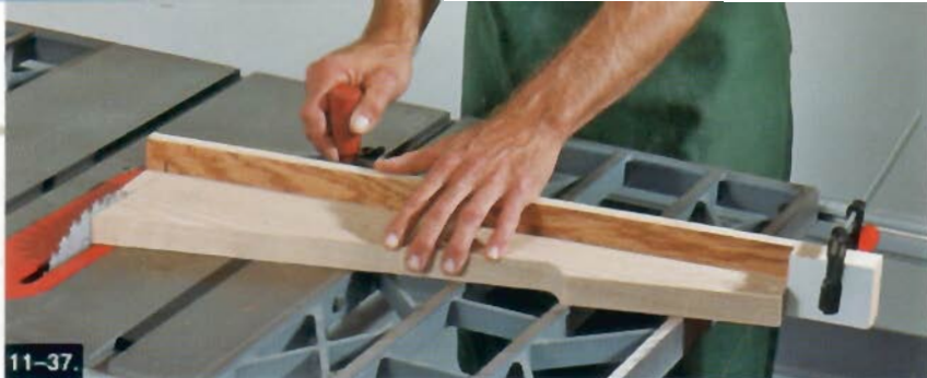
11-37. With your miter gauge set at a 6^\circ angle, trim the top of each leg. Then reset the miter gauge to 6^\circ the other direction, reset the stopblock, and cut the bottom ends.
