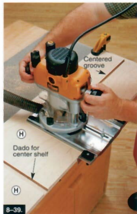
8-39. Adjust your router's edge guide to center the bit on the width of a side (H), and rout a groove from the bottom to the center shelf dado for the divider (K).
