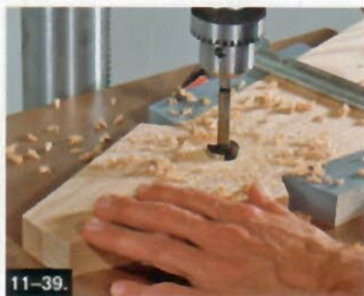
11-39. To make the half-round notches for the foot ring, clamp legs back-to-back and drill a 1" hole right on the centerline.
