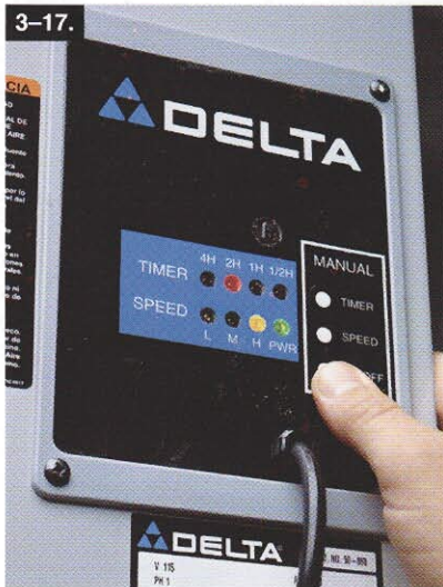
3-17. Touchpad controls are sealed from the outside to reduce dust penetrating to the switches.
