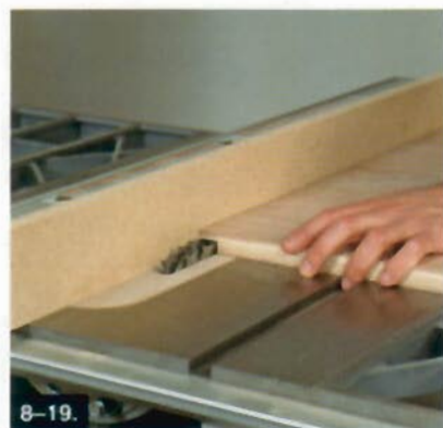
8-19. A wood auxiliary fence allows you to use the full width of the \frac{3}{4} " dado blade to cut rabbets in the plywood carcass panels.
