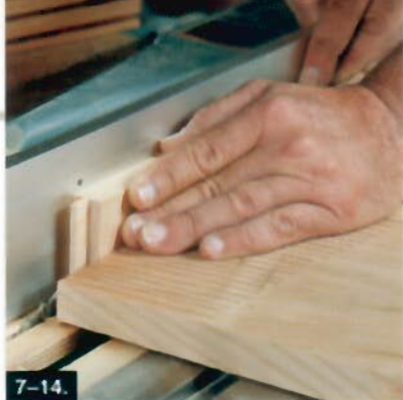
A feather board adds a lot to your accuracy when you're cutting grooves on the edges of the door rails and stiles.
