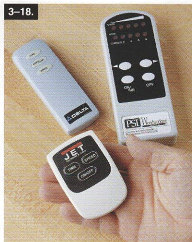
3-18. The remote control being held is easy to tuck into a pocket or misplaced. The one on the far right can be mounted to a wall, like a wireless switch.
