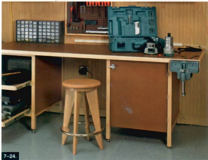
Fit two cabinets like this with a top (see Chapter 6) and, presto, you've got a sturdy workbench.
