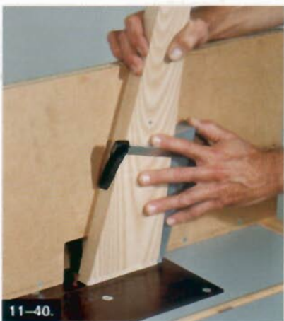
11-40. Make test cuts in scrap; then rout the dovetail tongue on the top end of each leg. A tall fence and follower block help.
