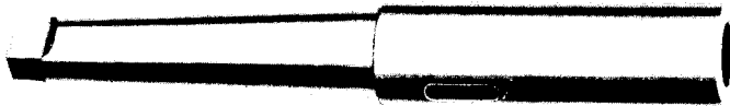
Figure 4-36 Steel socket used to hold twist drills with shanks too large to fit into either the drill press spindle or a sleeve.
