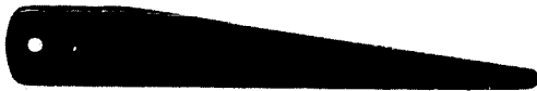
Figure 4-37 Drill drift used to remove twist drills, sleeves, and sockets from the drill press spindle. (Courtesy National Twist Drill and Tool Co.)
