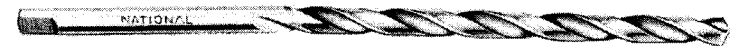
Figure 4-3 Taper-length, tanged, automotive series, straight-shank twist drill regularly furnished with tangs for use with split-sleeve drill drivers. (Courtesy National Drill and Tool Co.)
