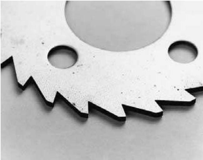
FIGURE 8.6 Ratchet wheel cut by a wire electric discharge machine (EDM).
