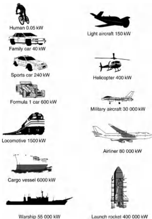
Figure 2.7 Comparative power outputs
