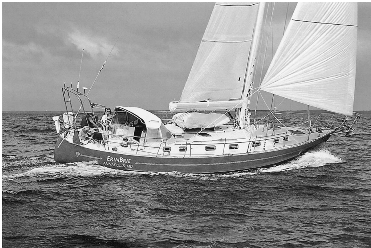
A Valiant 47 in Valiant 50 mode with tubular bowsprit. This boat has a Leisure Furl boom. I was never fond of the all-one-color topside paint jobs on these boats. To my eye a Valiant's lines are set off better with a white wale stripe above the rubrail.
