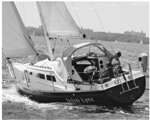
Another shot of Elisa and Mark's Islander 28, showing the boat's truncated stern and broad beam. The narrow cabin trunk and overall proportions still look great to me after 30 years.
