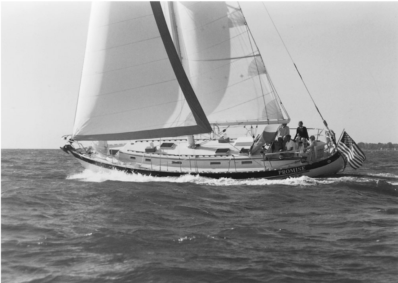
One of the later Valiant 40s, built just before we switched to the Valiant 42 model with the bowsprit. Note the boarding ladder obscuring my beautiful stern. This high-clewed genoa gives up too much sail area for my taste, but this is a good shot of a Valiant on a tight reach.
