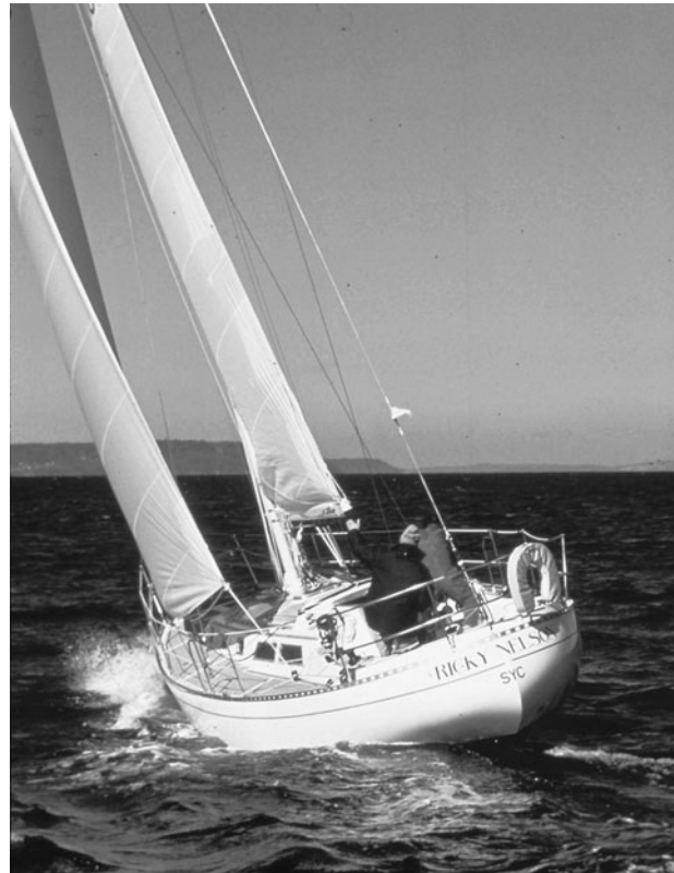
This is my Esprit, hull number 1. Hopefully I am indicating with my left arm to my crew that we need to do something about that baggy shape at the foot of the mainsail—perhaps “a little more main halyard, please.” (Roy Montgomery)
