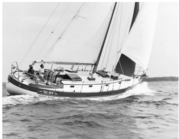
Ruby is the only custom, backyard-built Valiant. I moved Ruby's mast forward to help improve helm balance. Note the tiller steering.
