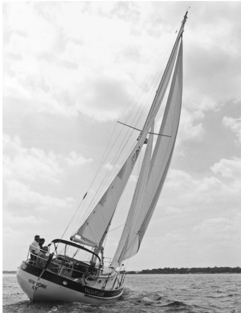
A Valiant 40 with the apparent wind at about 34 degrees and the mainsail oversheeted. An in-the-mast furling mainsail like this is hard to trim properly.
