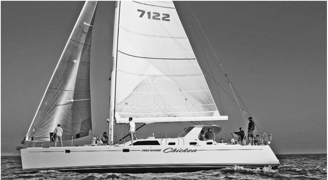
Free Range Chicken during her first day of sailing trials off Newport Beach, California. Note the small LP jib and the Leisure Furl boom.
