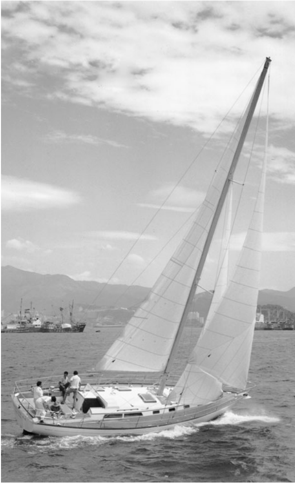
The CL 44 in cutter configuration, undergoing sailing trials in Hong Kong harbor.
