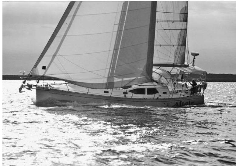
The Saga 48 Altair under sail. A plumb stem requires a bowsprit for anchor handling.
