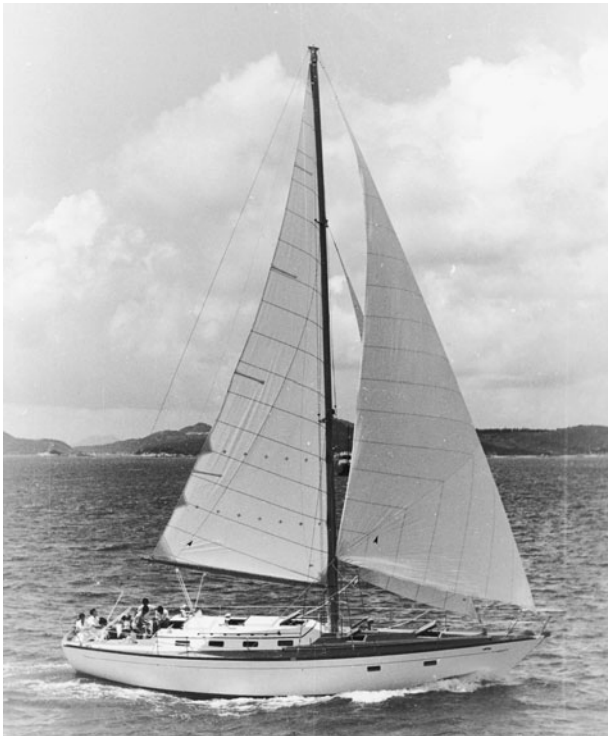
Hull number 1 of the CL 48s undergoing sailing trials in Hong Kong harbor. A vang would have helped the mainsail shape.
