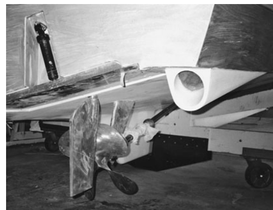
Figure 7-27. Exterior view of the Cape Dory's underwater exhaust system
