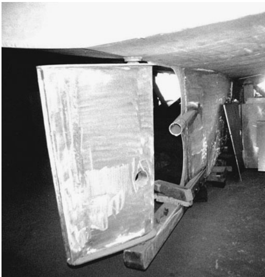
Figure 13-7. MacLear Thistle rudder with endplates
