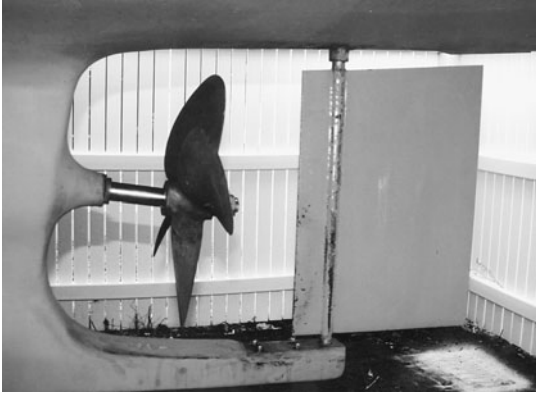
Figure 10-9. Basic flat-plate rudder
