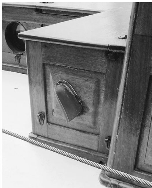
Figure 14-13. Clamshell vent on a locker
