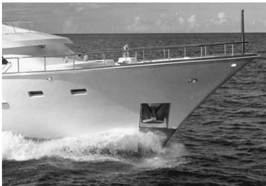
Figure 24-16. Anchors in hawsepipes (Courtesy Hargrave Custom Yachts)
