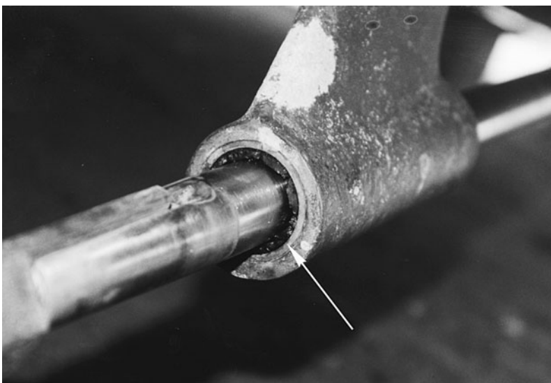
Figure 1-11. Worn Cutless bearing
