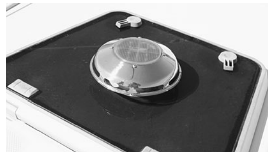
Figure 14-9. Solar mushroom vent (Courtesy Jack Hovnor)
