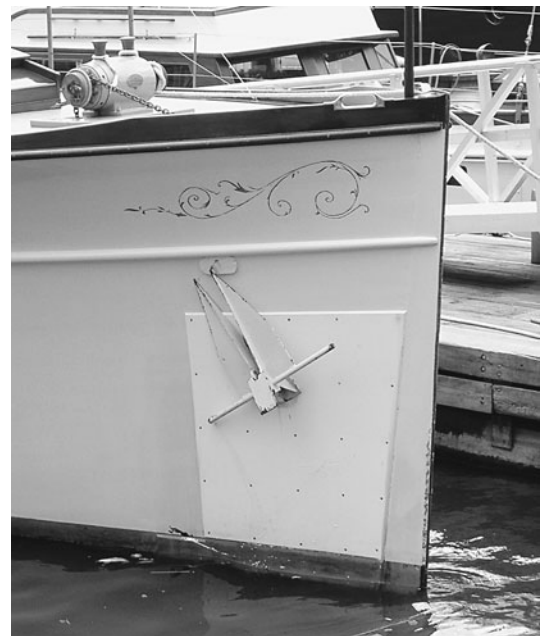
Figure 24-14. Danforth anchor in a hawsepipes. (This bow also has a plastic chafe pad)
