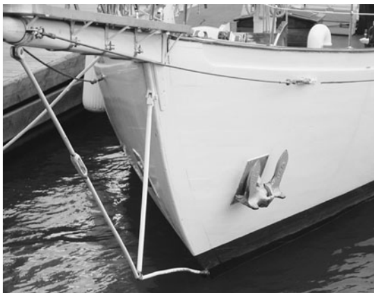
Figure 24-15. Bobstay damaged from anchor chain
