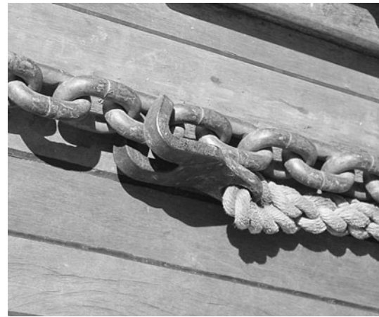
Figure 23-14. Devil's claw used as on-deck chain snubber
