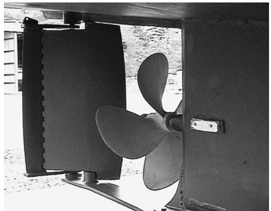
Figure 13-11. Deflector Rudder to starboard
