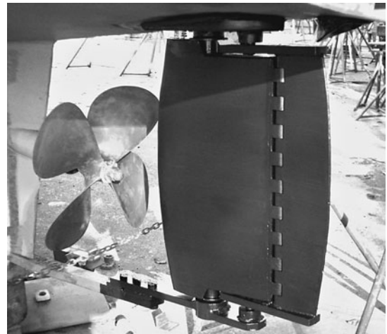
Figure 13-10. Deflector Rudder amidships
