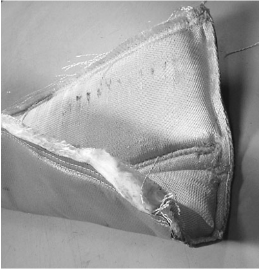
Figure 9-20. Fiberglass insulation cover (Courtesy Applegate Industrial Materials, Inc.)
