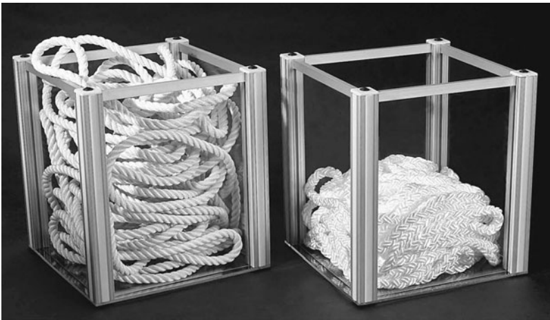
Figure 23-12. Yale Brait rope (right) versus three-strand nylon rope (Courtesy Yale Cordage)
