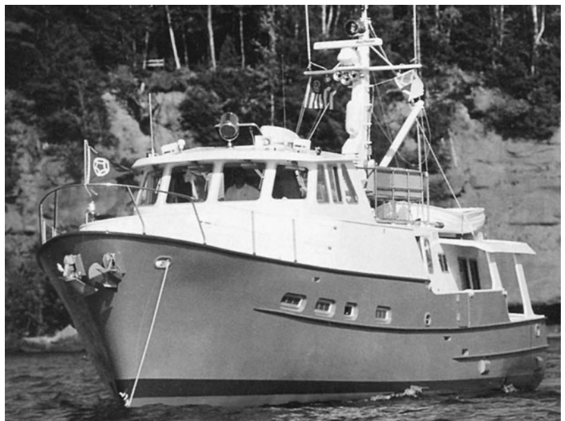
Figure 24-12. Bow-on view of Imagine 's double anchor rollers
