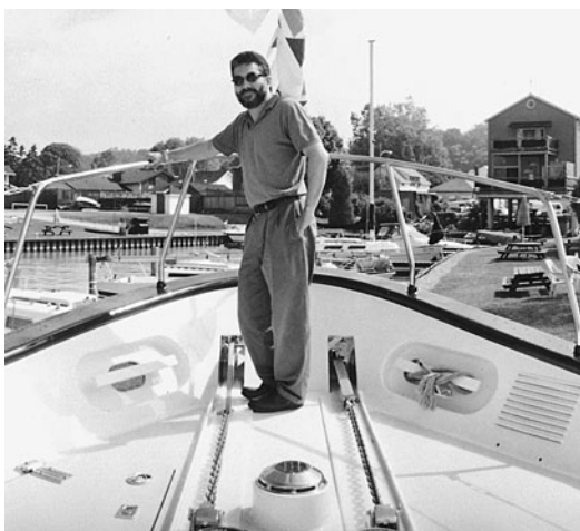
Figure 14-12. The author on the foredeck of Imagine . Note the solar vent amidships between the anchor chains. Note the louvre vent on the starboard bulwark.
