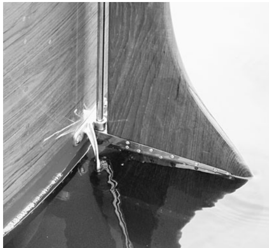
Figure 12-16. Bronze outboard rudder stop
