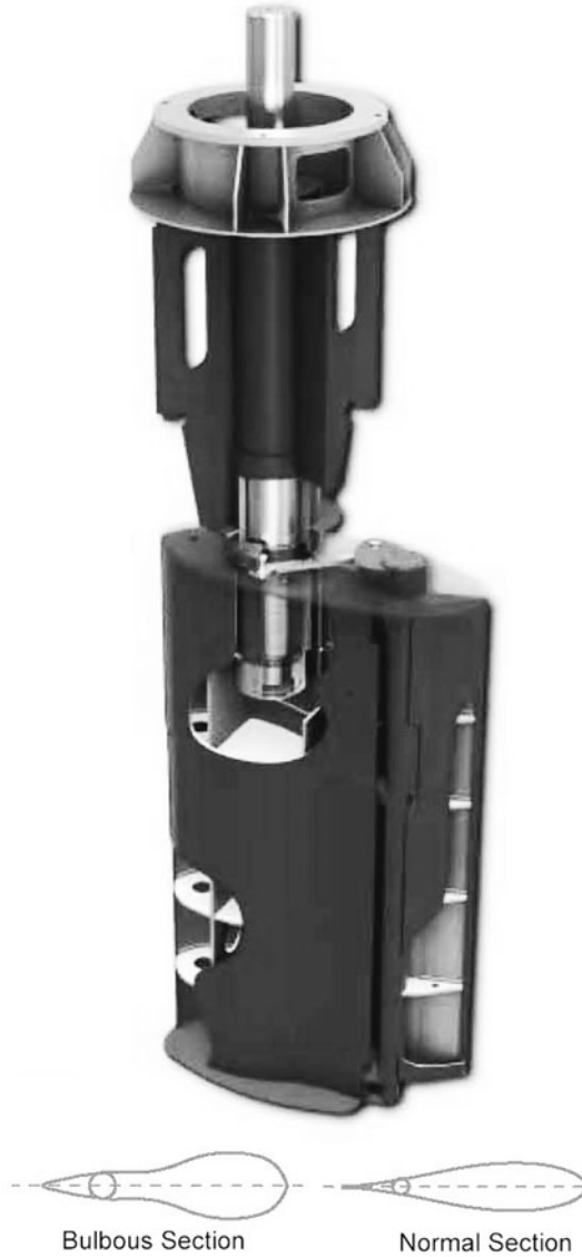
Figure 13-10. Deflector Rudder amidships
