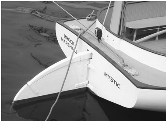
Figure 10-10. Barn-door rudder on a Marshall Catboat
