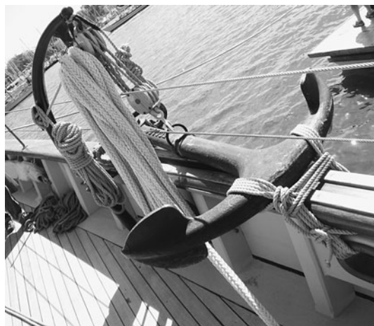
Figure 24-3. Admiralty-pattern anchor lashed to bulwark under the anchor davit
