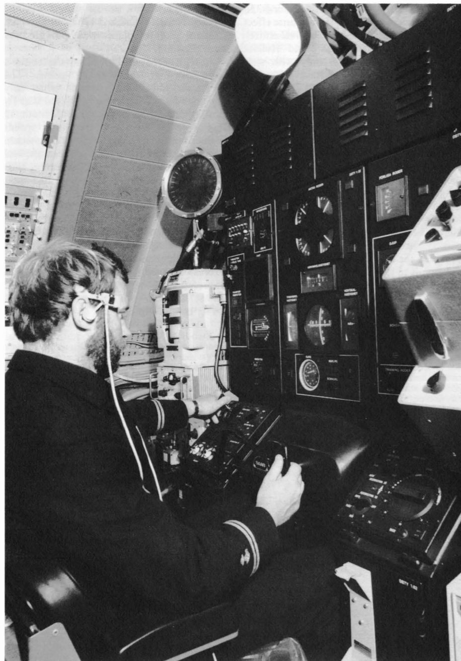
The Royal Swedish Navy now used integrated helm and plane controls (single operator control) as illustrated here aboard a Näcken -class submarine (6 December 1979). Kockums
