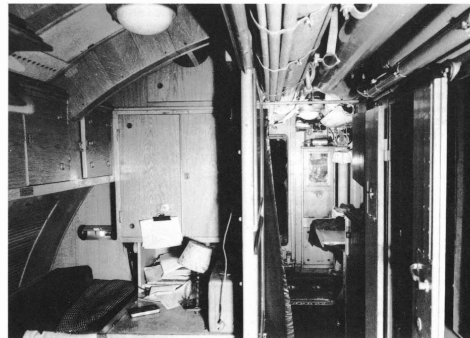
This may convey some impression of how crowded U-boats were. Even the Type IX was small by US standards. These are officers' quarters next to No 2 battery room. Most of the enlisted men had to 'hot bunk' (use the same bunks in rotation).
