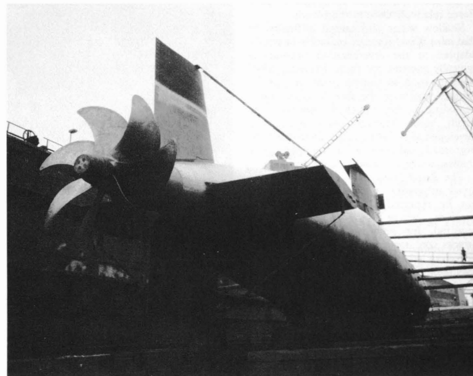
A modern scythe-form propeller is shown on an HDW submarine in drydock. Since 1962 German yards, principally HDW, have delivered or are delivering 97 submarines for 16 countries.
