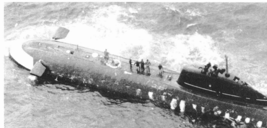
The Soviet Navy lagged behind the US Navy by about three years in introducing nuclear attack submarines; the 363ft 'November' class of 4500/5300 tons (15 built 1958-64), one of which is shown in distress off Cape Finisterre on 10 April 1970, was the first. The short sail and mast radome are Soviet characteristics. US Navy
