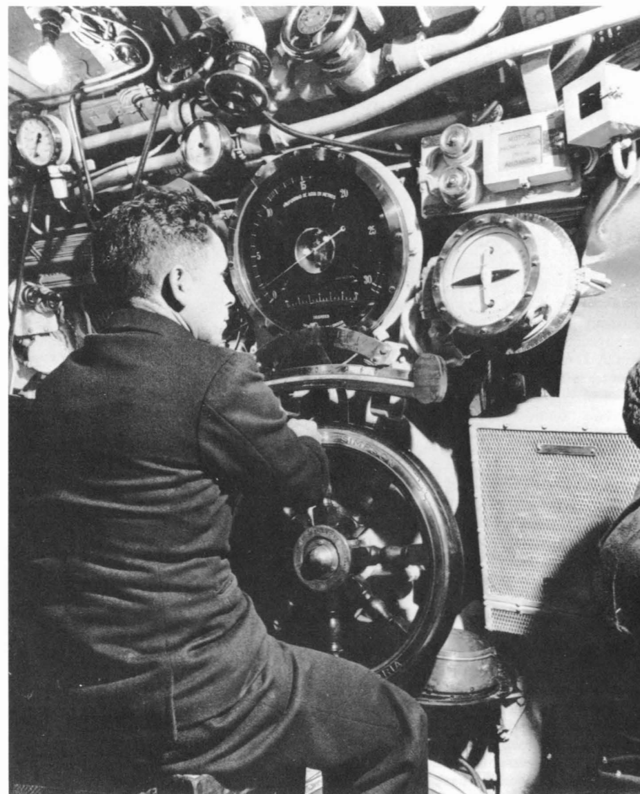
The planesman, controlling (probably) the stern planes, has a depth indicator (in metres) with a 'bubble' to show the inclination of the submarine. The dial to his right, which he is watching, displays diving plane angle.
