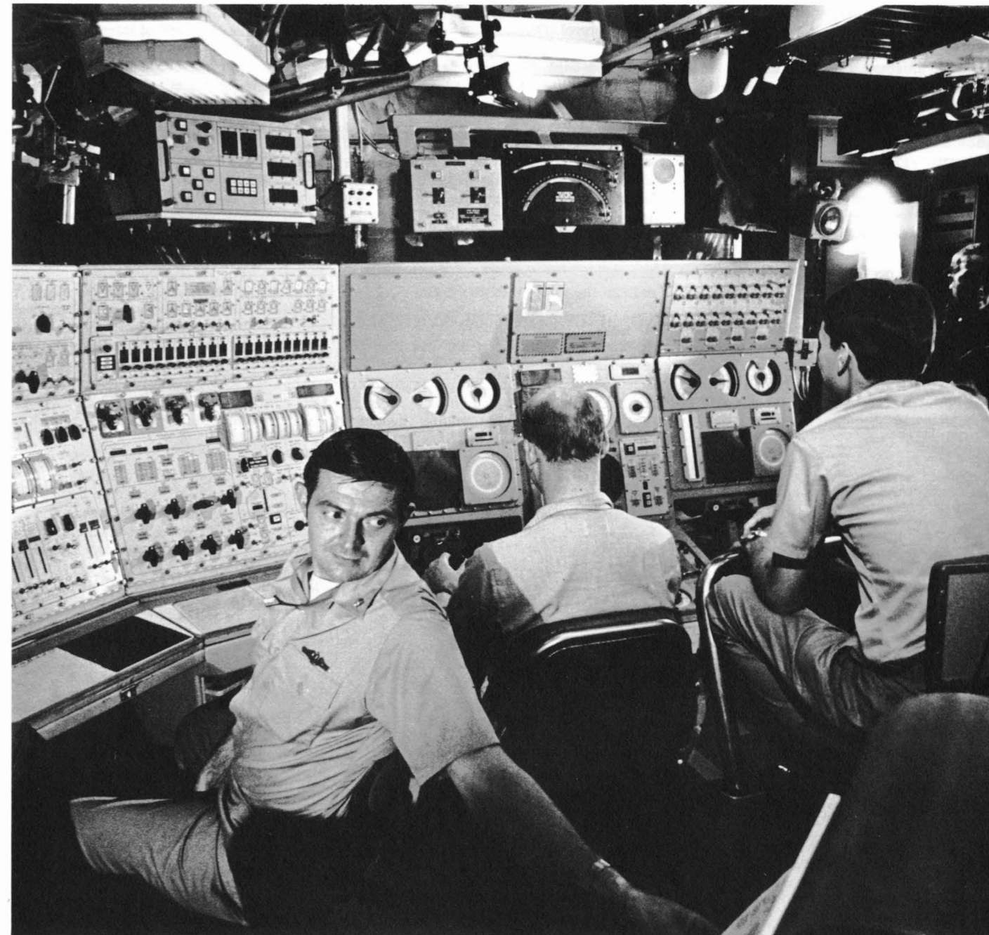
Modern US control room design is exemplified by the new ballistic missile submarine Ohio in October 1981. The diving control panel is at the left, with the planesman in the centre of this photograph, and the helmsman to his right, obscured by the diving officer who supervises both. The plane/helm control panels are identical, and are set up so that one man can operate both planes and helm as an integrated control system. However, two-man operation is standard US practice. Many foreign navies have gone much further with automation, and at times the US Navy is accused of over-manning, of excessive preference for men over automation. The standard reply is that, as long as automation can be avoided, human control is far more reliable. US Navy
