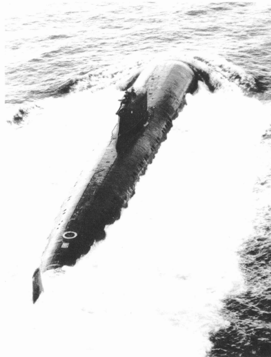
The nuclear-powered 'Charlie' cruise missile classes (12 'Is' built 1969-73 and 6 plus 'IIs' since 1973), an example of which is shown before 1975, were direct descendants of Soviet anti-ship attack submarines, missiles (SS-N-7) replacing their torpedoes. Eight external tubes occupy her bow section, forward of her diving planes (note the covered slot). MoD
