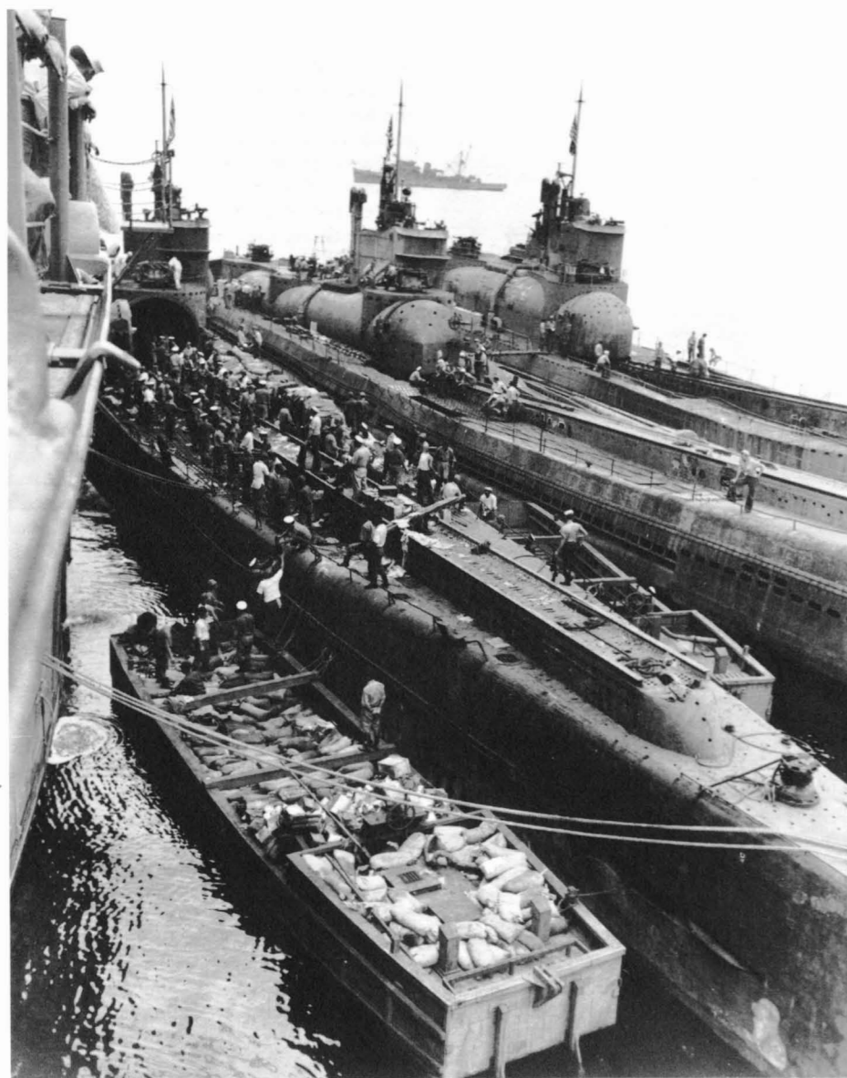
Japan followed a very distinctive course of submarine development, typified by the three I-401 class submarine aircraft carriers shown after their surrender in 1945. The catapult track of the nearest submarine is obscured by sailors unloading stores. Note the large hangars passing through the superstructures of all three, and the snorkels abaft their bridges. At 3530 tons and 400ft oa they were the largest submarines built until the advent of ballistic missile craft. US Navy
