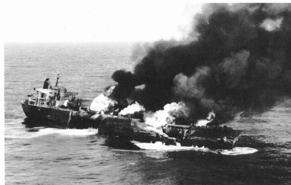
Torpedo lethality is often less than might be expected. These photographs show an attempt by a Japanese Maritime Self-Defence Agency submarine to sink the large derelict tanker Yuro Maru in the North Pacific during November 1964. Both show the tanker after one torpedo hit, in the fourth of four attacks. She had already been hit repeatedly by 5in shells, by 250lb bombs and 5in rockets from jet fighters, and by 500lb bombs and 5in rockets from Lockheed P3 Neptune maritime patrol aircraft, over a period of three days. Of three torpedoes fired, only one hit. Another failed to run, and a second ran deep. Even after all of this damage the tanker remained afloat for another three days. A second submarine attack was, therefore, cancelled. Japanese Maritime Self-Defence Agency
