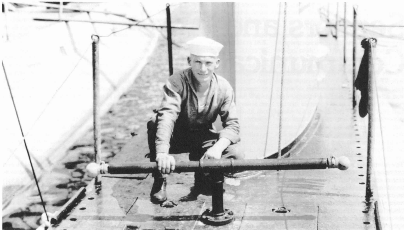
The simpler alternative to electronic rotation was physical rotation of a directional hydrophone: this is a C-tube, aboard the US submarine H-5 , at San Pedro about 1919. Each bulb enclosed a microphone attached to a headphone, and the operator turned the device until the sound level was equal in both his ears. This device operated at relatively low frequency, and therefore its 5ft baseline gave it only poor directionality. During the interwar period both the US and Royal Navies turned to 'supersonics', ie to much higher frequencies, for both active and passive sonars, to achieve better directionality with devices of similar size. Ultimately they had to return to lower frequencies for their passive systems, because water absorbs higher-frequency sound too well. US Navy
