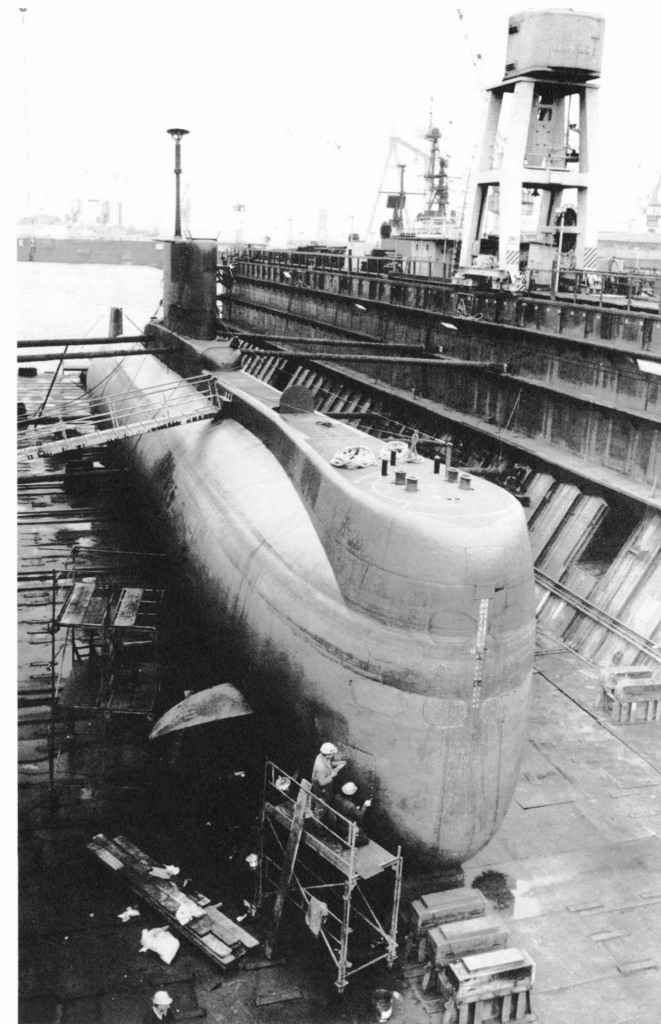
An HDW-built Type 209 in drydock shows several characteristic features: the nest of eight bow tubes, the extended (curved) bow plane and the single-hull configuration. HDW
