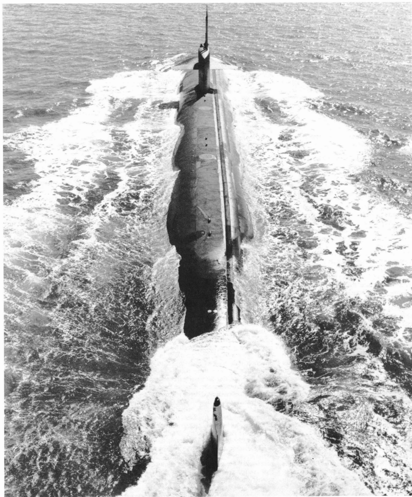
USS San Francisco (SSN 711), a Los Angeles class attack submarine, stows her towed tactical array passive sonar in the fairing running aft along most of her 360ft hull, and visible in this 15 March 1981 photograph of her in the James River during sea trials, (just prior to completion by Newport News Shipbuilding of Virginia). There is too little space in her ballast tanks to stow more than the associated winch and cable; the array is deployed from one of her tail fins, so as not to foul her propeller. In theory, a thinner array might be stowed inside her hull, and so could be made substantially longer, for better directivity. US Navy
