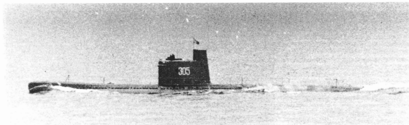
At 183ft and 400/540 tons the smallest of the three Soviet submarine classes begun just after 1945. 'Quebec' (seen here on 5 January 1961) was the only one with a closed-cycle (Kreislauf) powerplant; 30 were built (1954-57), only being operated in the Baltic and Black Sea. The projection at the rear of the sail housed the snorkel. US Navy
