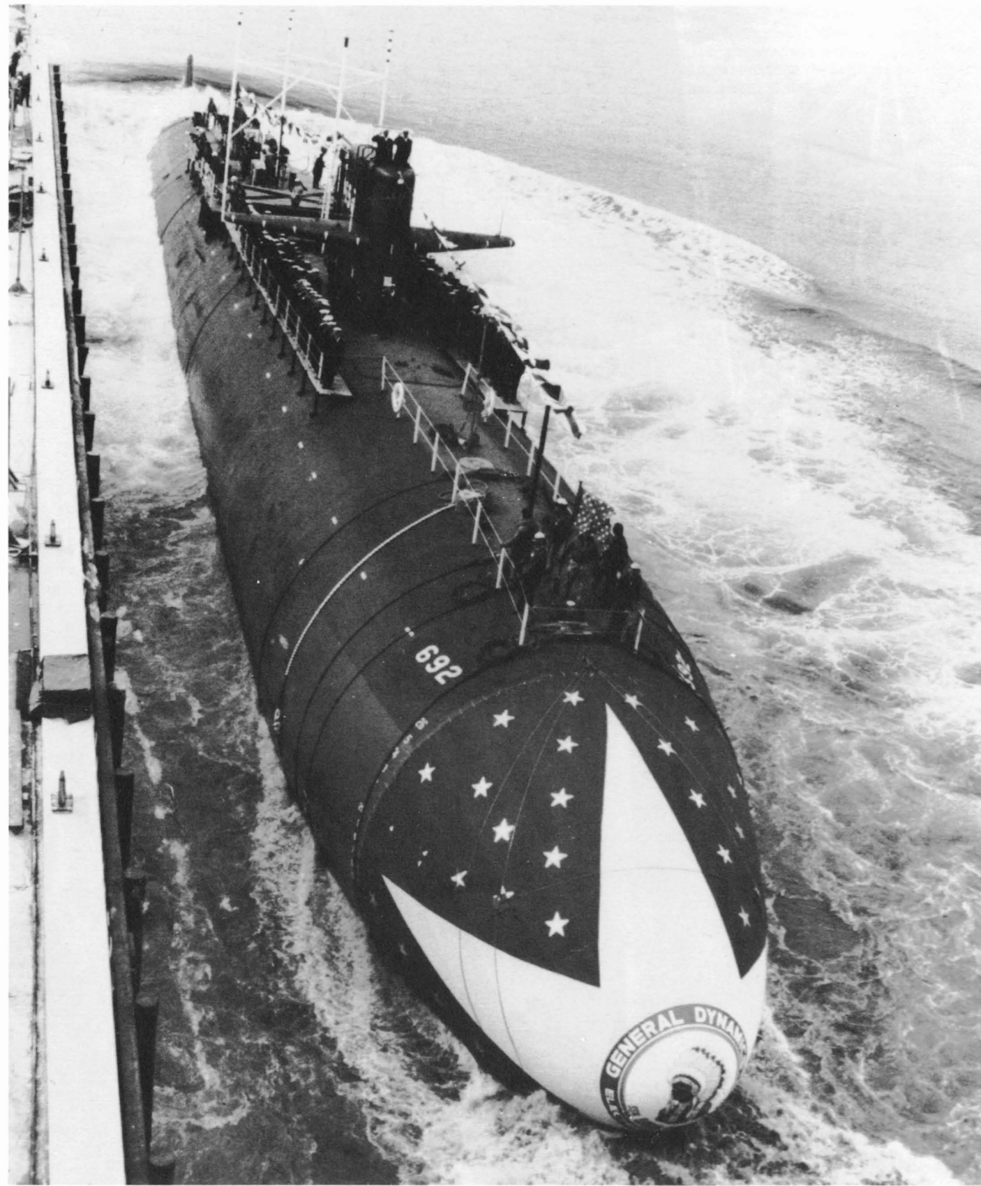
Although a continuously curved hull form is best, it is almost as efficient to use a cylindrical middle body, which is much easier to build. This is the Los Angeles class nuclear attack submarine Omaha (SSN 672) launched on 21 February 1976 at Groton, Connecticut. Note her relatively small sail, its size minimised to reduce resistance in a submarine built for very high speed. As a result, the planes cannot be rotated to the vertical position, and thus the Los Angeles class cannot break through ice. From units built under the FY83 Program onwards, Los Angeles class submarines will have their forward diving planes relocated to their hulls, primarily for under-ice operation. US Navy
