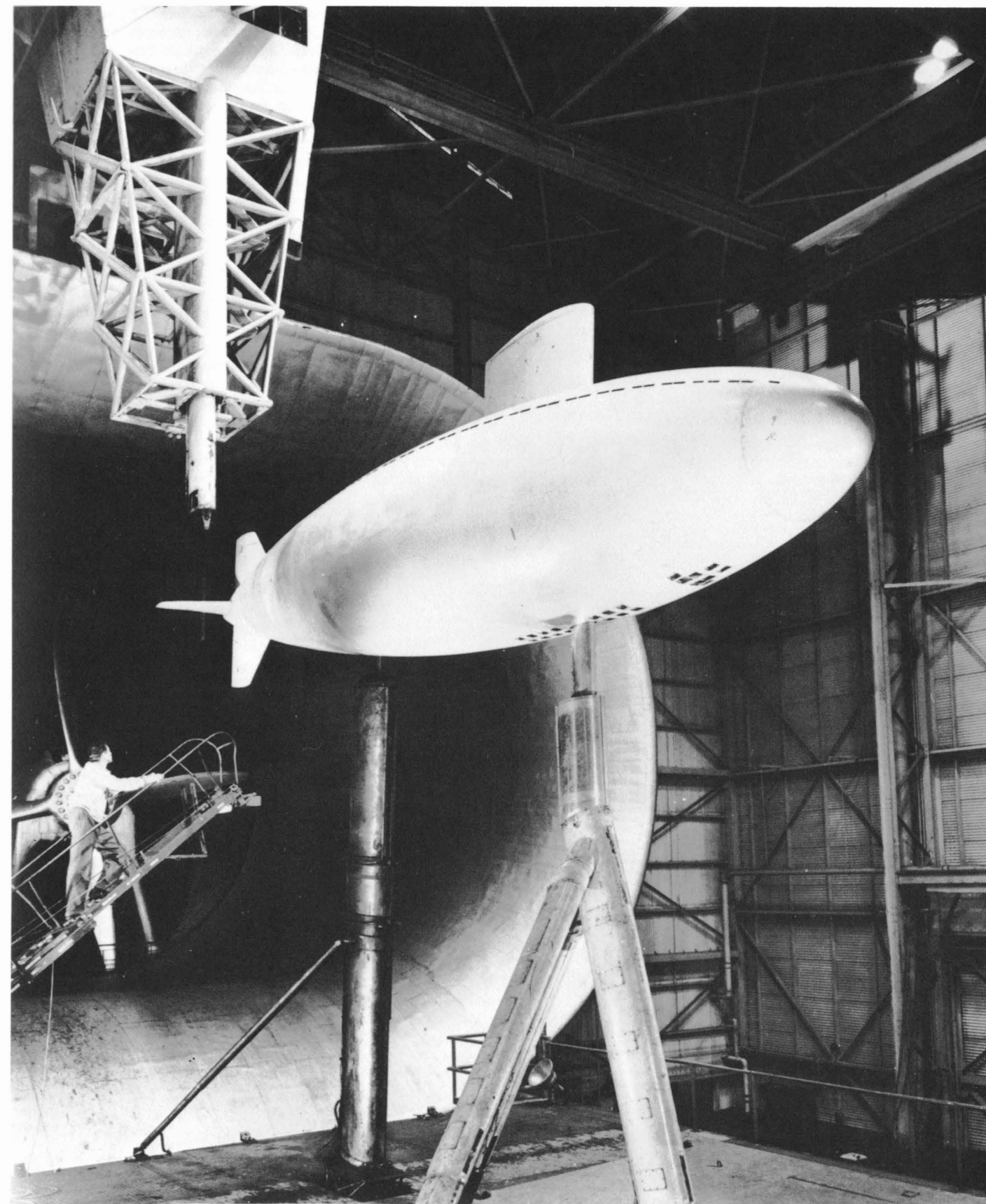
The diesel-powered experimental 210ft USS Albacore (AGSS 569) transformed postwar submarine design when built in 1953. Once the possibility of very high underwater speed (a reported 33 knots in final form) had been demonstrated, the submarine community demanded it in operational craft: the Skipjacks were the result. This wind tunnel model clearly shows the relatively fat Albacore hull form developed on the basis of airship practice. Note the numerous vents and limber holes and the total absence of bow planes. US Navy
