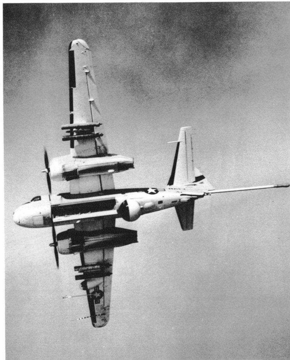
Aircraft may be the most potent ASW weapon, at least in the open ocean. This Grumman S2F Tracker (over the Atlantic near Long Island on 30 December 1960) shows both its bomb bay and main sensors: a snorkel-detection radar in a retractable radome, sonobuoy dispensers (at the rear ends of its nacelles) and MAD in the tail 'stinger' or boom. The latter is essential for precise placement of weapons but has so short a range that its user must fly very low, subject, perhaps, to future submarine launched anti-aircraft weapons. Note also the searchlight (in the starboard wing) used to illuminate submarines surprised on the surface and the inboard rocket pods for attack flanked by homing torpedoes. Such aircraft also carry two other detection devices: ESM, the direct descendant of World War II HF/DF and 'sniffers' capable of detecting snorkel emissions. Submarine designers counter 'sniffers' by emitting exhaust underwater, and infra-red detectors by artificially cooling the exhaust.
