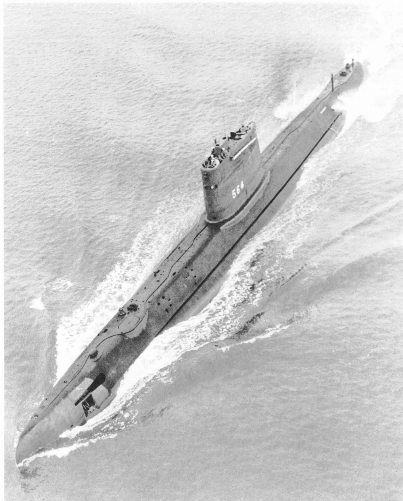
The Tang class attack boat Trigger (SS 564, seen in May 1967) typified the US equivalent of Type XXI. Note the slot for her retractable bow plane, and the absence of deck fittings; her safety lines retracted into the slots visible on deck. The small sonar dome probably housed an underwater telephone. US Navy
