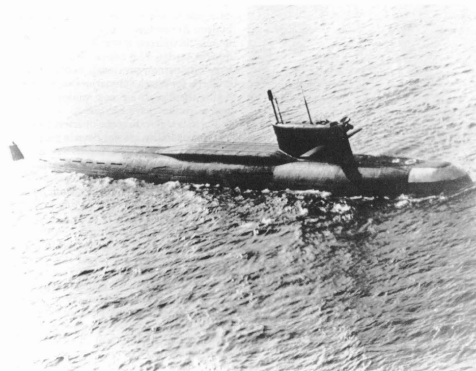
Soviet SSBNs are a remarkable demonstration of the effect of industrial inertia. There is considerable evidence that the original 'Yankee' was developed very rapidly (34 built 1967-74); its pressure hull diameter was just less than the 33ft length of the SS-N-6 missile. 'Delta', in its three versions (36 built since 1972), consists of a 'Yankee' hull, suitably lengthened with a hump raised sufficiently to take SS-N-8 and then SS-N-18 missiles. Presumably the process could not be continued with the Typhoon's SS-N-20 because the holes for the new much larger (49ft) missile would have weakened the pressure hull too badly. The existing hull may also have lacked sufficient volume for the fire control system associated with the MIRVed SS-N-20. 'Yankee' class ballistic missile submarine (426ft oa and 8000/9600 tons) in or before August 1976. One of her sail mast hatches is opened.
