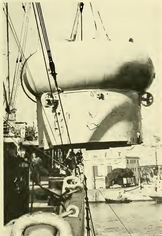
Fig 3.34 This 55-ton hyperbaric section of PHOENIX 66 will be encapsulated into a 70-ft-long submersible for oil field work to 1,200 feet with a crew of seven (Sub Sea Oil Services, Milan)
