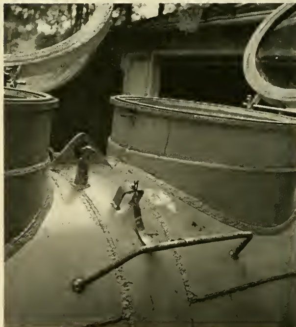
Fig 14 19 A scuba bottle valve attached to a thru-hull penetration provides air from a scuba tank to blow main ballast in the All Ocean Industries vehicles. The rack in the foreground holds the scuba bottle.
