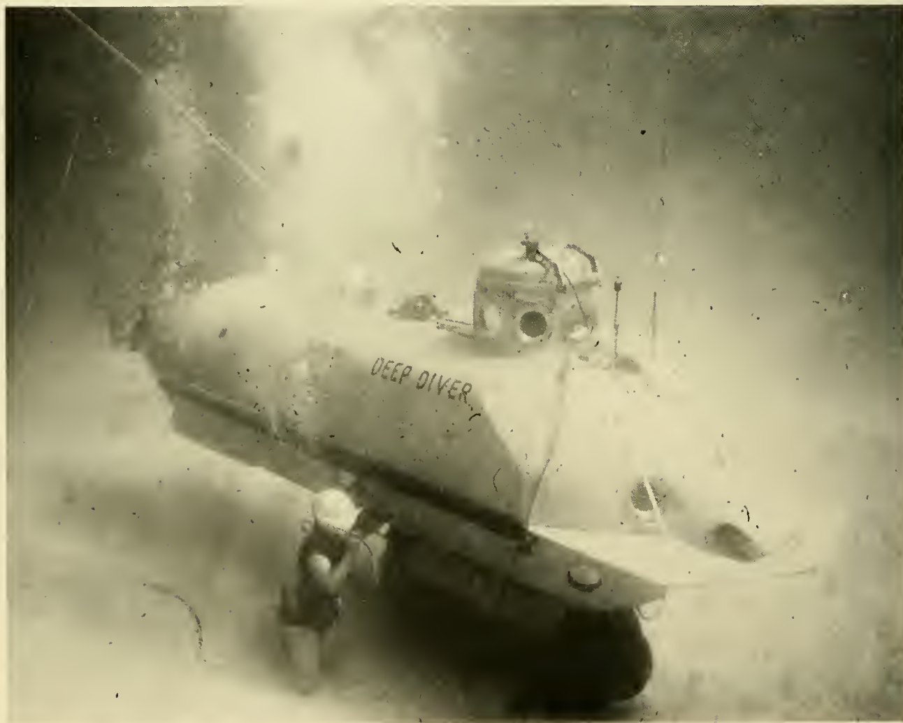
Fig. 3.23 The Perry-Link DEEP DIVER was the first modern submersible to incorporate a diver lock-out feature. (Ocean Systems Inc.)
