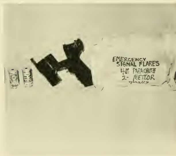
Fig 14 11 Distress rockets (left) and hermetically sealed parachute flares (right) may be fired from the launcher (center) carried aboard DEEPSTAR 2000 .
