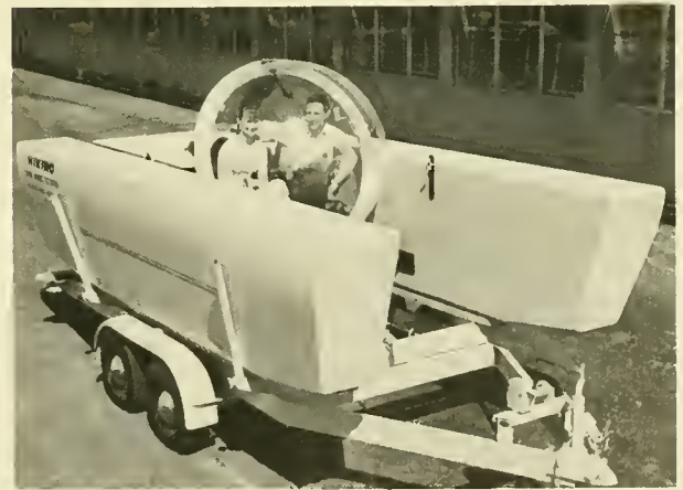
Fig. 3.22 The plastic-hulled HIKINO set an early precedent for submersibles of the seventies. (U.S. Navy)
