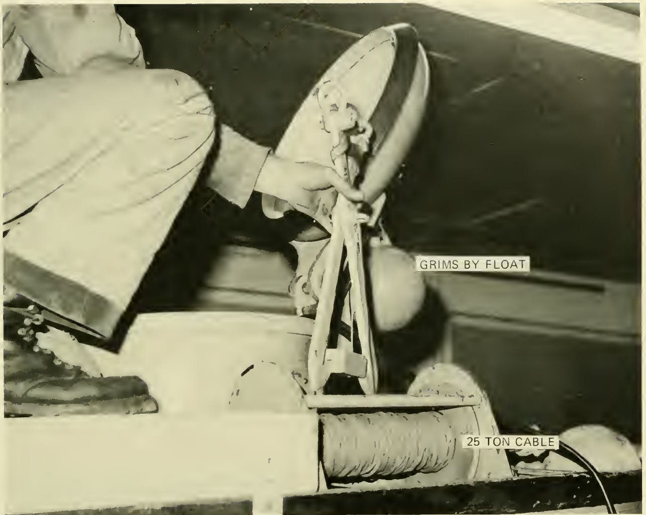
Fig. 14.17 SEA OTTER's marker buoy (Grmsby Float) is released by rotating a handle in the hatch cover which pulls out a restraining pin. As the float ascends it reels out the \frac{1}{4} -inch line which is spooled around and attached to a 25-ton-capacity cable shackled to the hull. The ice tong-like device is slid down the line which is fair-led through a hole in the block holding the tongs open. Reaching the cable, the block is knocked out and the tongs close on the cable. A lift line attached to the tongs is then employed to retrieve the vehicle.
