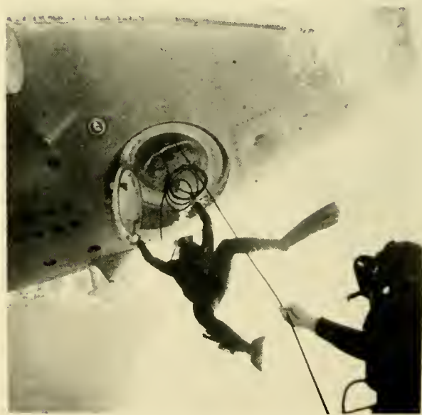
Fig. 14.5 Divers approaching the lock-out hatch of BEAVER . Air pressure in the aft sphere is equal to water pressure and prohibits entrance of seawater. (North American Rockwell)
