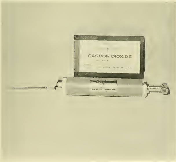
Fig. 9.16 A Kitagawa \text{CO}_2 detection kit used as a backup system aboard DS-2000
