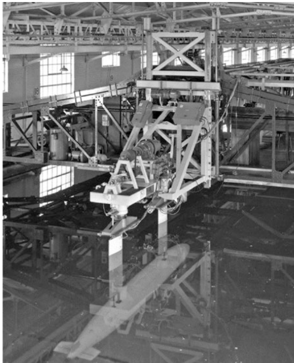
Fig. 3.8 Typical set up for captive model tests using a VPMM (courtesy of QinetiQ Limited, © Copyright QinetiQ Limited 2014)
