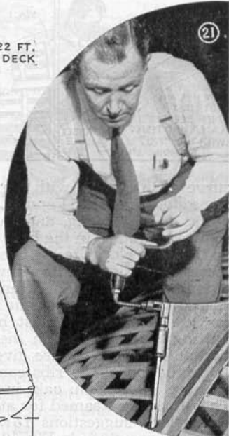
Fig. 21 shows how to bore the rudder-post hole, using the after skag as a guide
