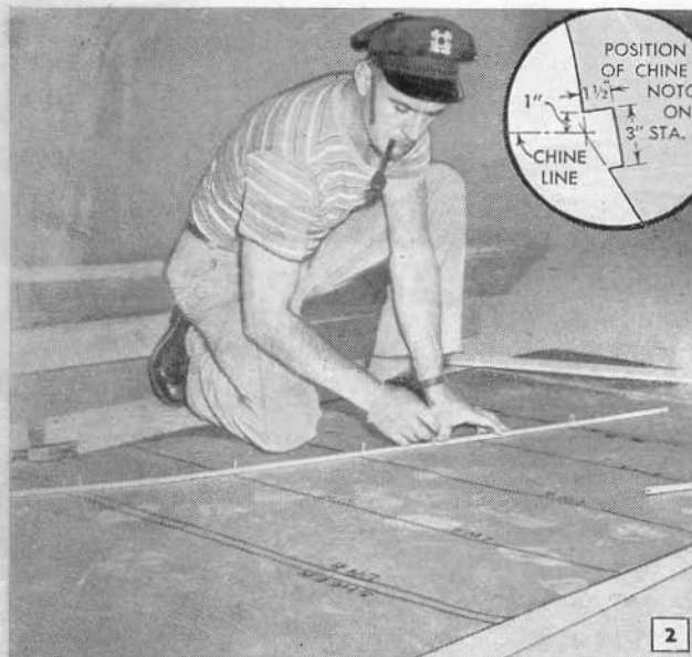
Above, full-size half pattern of each station is drawn on heavy paper. Left, the natural curve of a wooden batten is used to mark curved line connecting half-breadth dimensions
