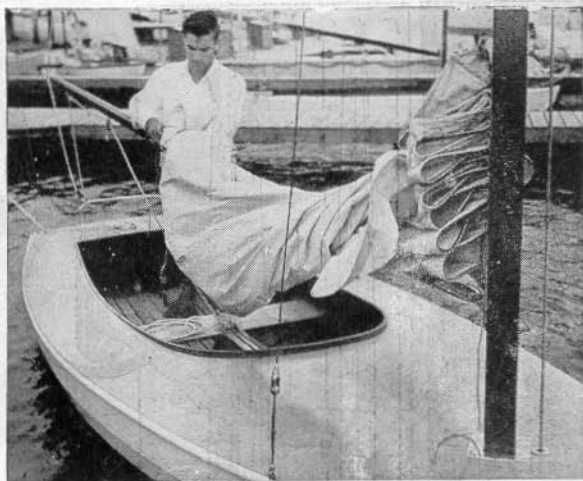
Top photo shows the foot of the sail being tracked on the boom in readiness to be hauled aloft, while the lower photo, a stern view of Zephyr, shows the fast, trim lines of its hull and roominess of the cockpit
