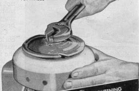
② TIGHTENING THE CONDENSER
