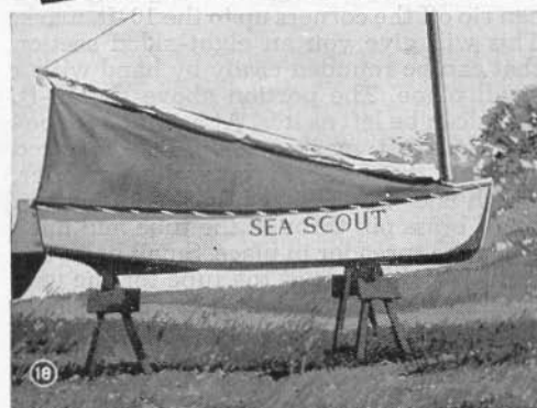
A tent cover, Figs. 18 and 19, is quite simple to make and is a protection to the boat and occupants when making cruises. The edges of the tent are held down by screw eyes spaced 8 in. apart below the boat's molding
