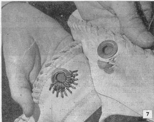
7 The herringbone stitch also is used to repair tears around grommets. In making the repair, one loop of each stitch passes around the grommet ring as shown
