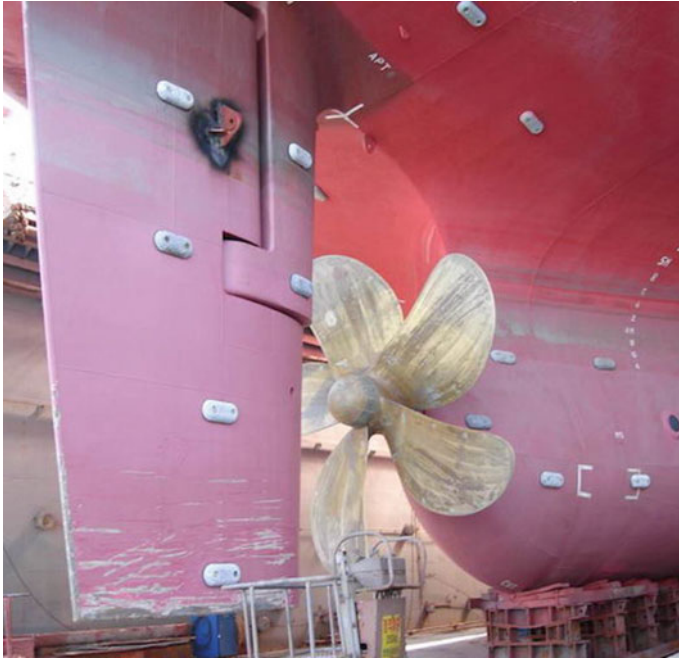
Fig. 6.17 A typical spade rudder with intermediate support
