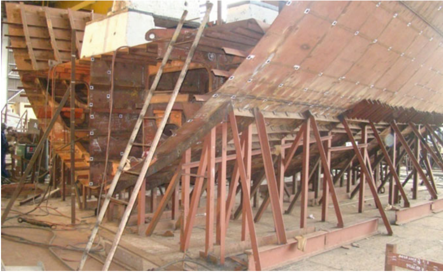
Fig. 17.17 A hull unit in a skid fitted with longitudinal and transverses
