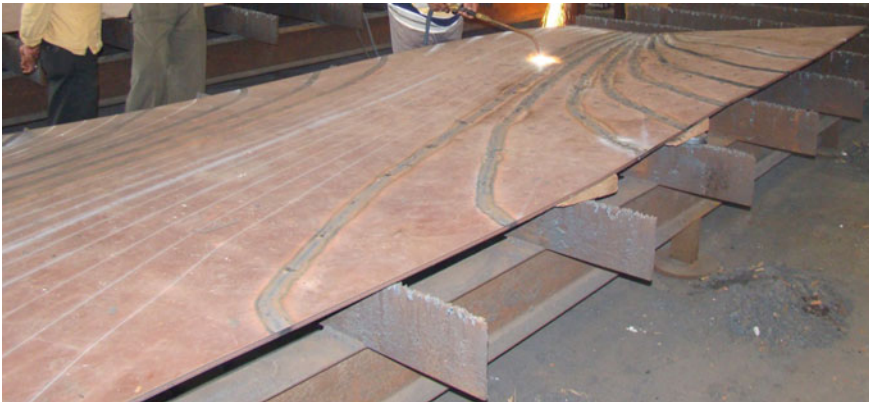
Fig. 12.9 Manual line heating with oxy-acetylene gas flame
