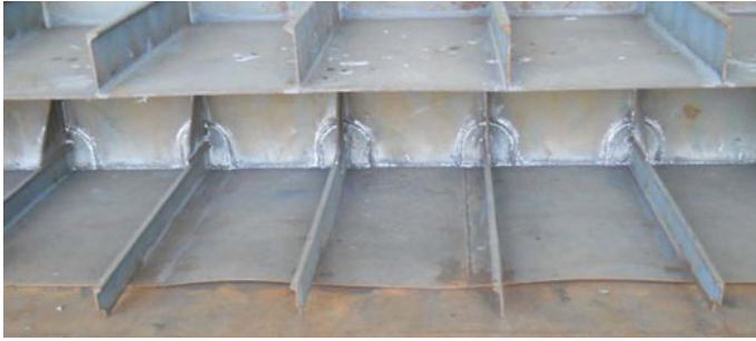
Fig. 17.3 May lead to poor fitup
