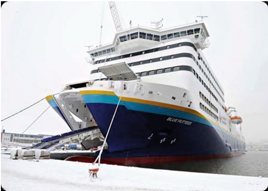
Fig. 1.8 A typical RO-RO ship with bow ramp
