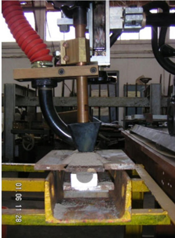
Fig. 15.18 Single side submerged arc welding with flux filled aluminum backing bar
