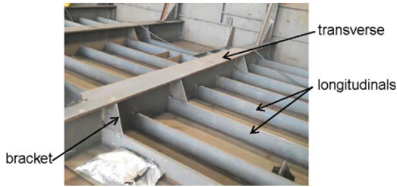
Fig. 4.3 Longitudinal framing system—longitudinals supported by the transverses
