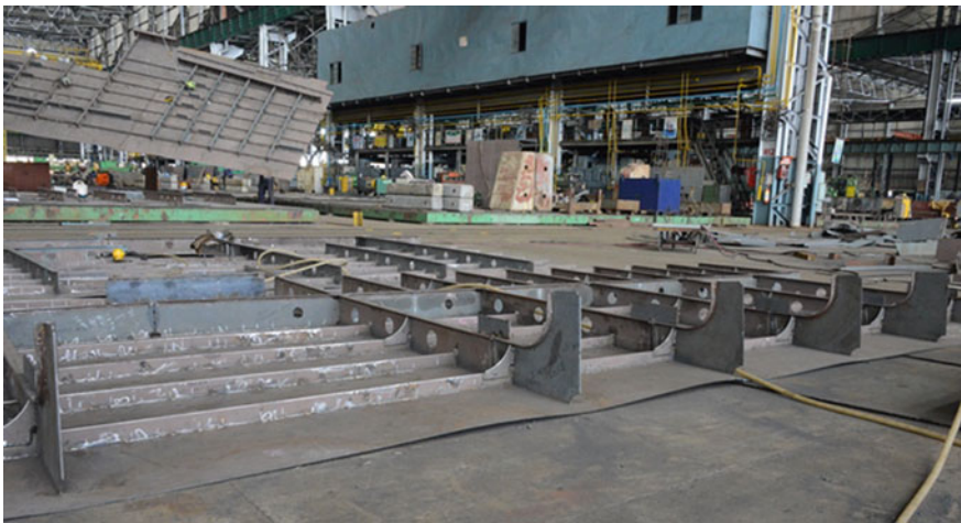
Fig. 3.11 Typical longitudinally framed stiffened panels
