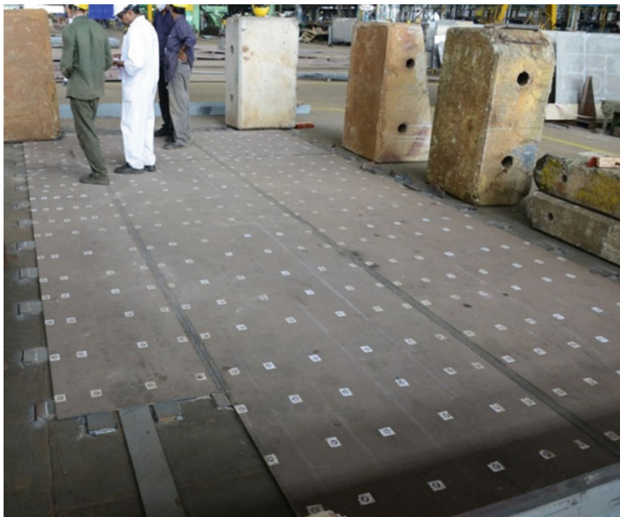
Fig. 18.9 The plate panel with lugs fitted all around
