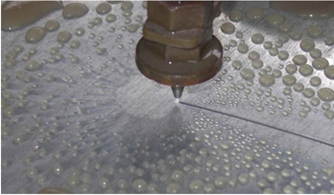
Fig. 11.4 Waterjet cutting of steel plate
