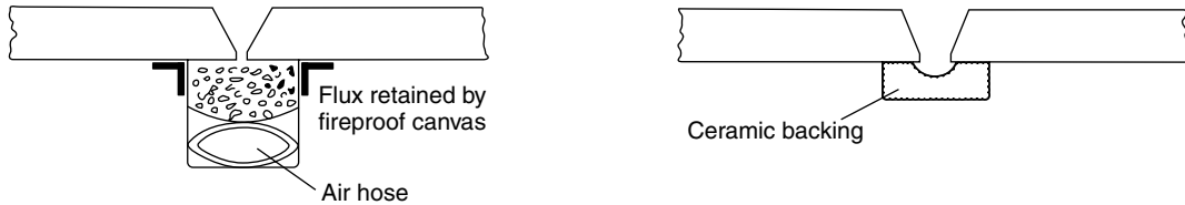
FIGURE 9.4 Automatic arc welding
