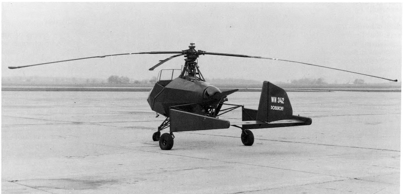
Fig 7.2 The Doblhoff WNF 342 V4 jet helicopter.
