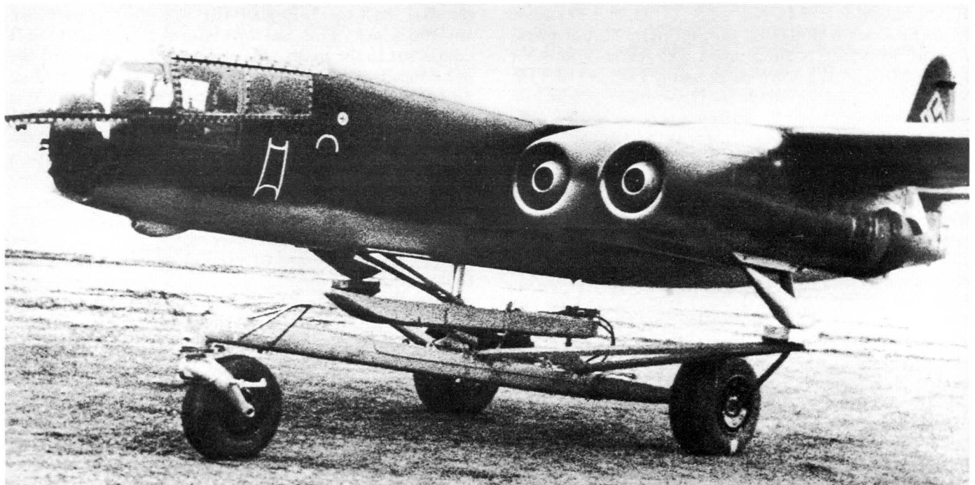
Fig 2.82 The Arado Ar 234 V8 prototype was fitted with four BMW 109-003 A-0 turbojet engines as part of the trials to ascertain the best arrangement of engines for the more powerful Ar 234 C. (Phillip Jarrett)
