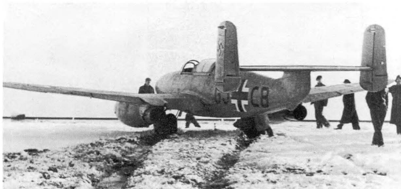
Fig 2.10 Heinkel He 280 V3 (GJ+CB). ABOVE LEFT: With engines uncowed owing to early fuel leaks. ABOVE: Later, following a landing skid.
