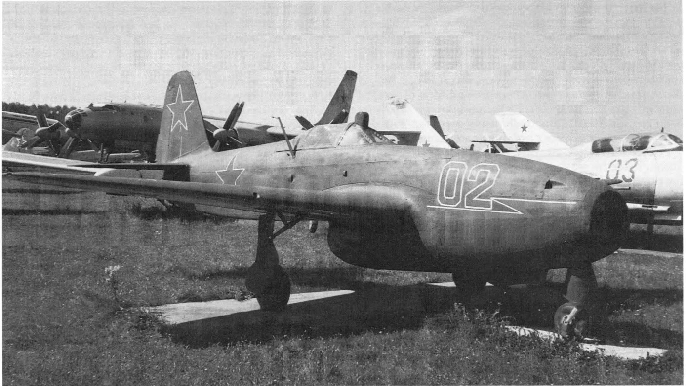
Fig 2.73 An example of post-war utilisation of Junkers turbojets is this Soviet Yak-17 fighter with an RD-10A turbojet (109-004). The similarly powered Yak-15 had entered service on 24 April 1946 and the Yak-17 entered service in 1948. Both were capable of about 500 mph at 3,000 m (9,840 ft). (Author)
