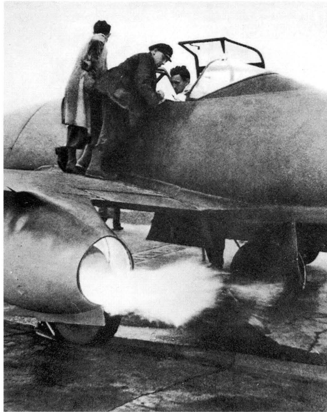
Fig 2.40 A pre-production Messerschmitt Me 262 A-0 as a test pilot lights up the port Junkers 109–004 B-1 turbojet. Bad velocity distribution of the combustion gases was in the process of being cured with this version of the engine.
