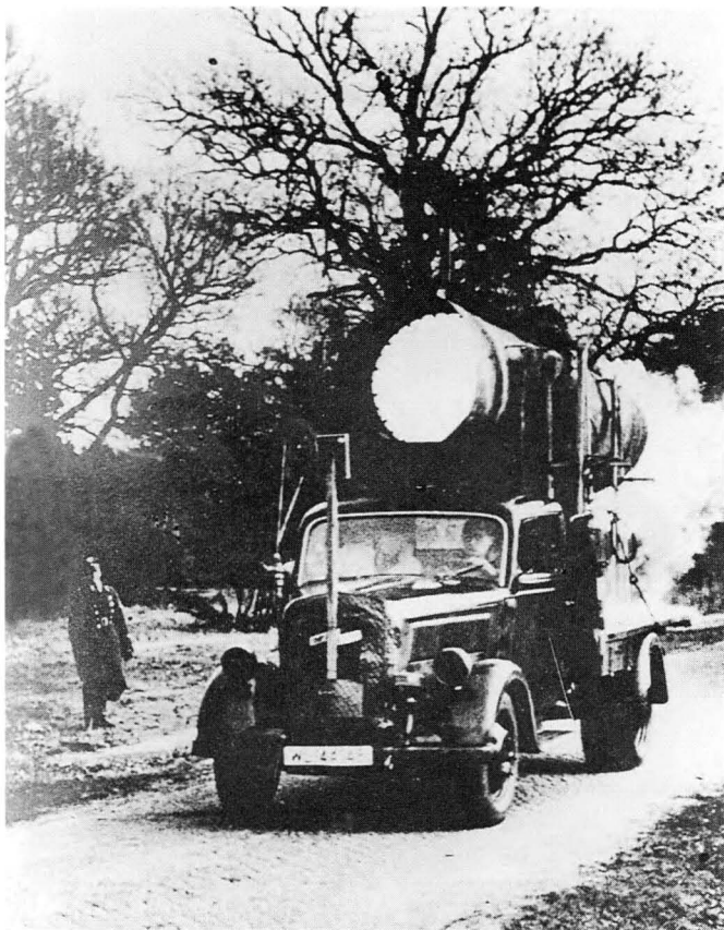
Fig 9.12 An 800 mm tube, mounted on an Opel-Blitz truck, used to conduct ramjet combustion tests in October 1941.
