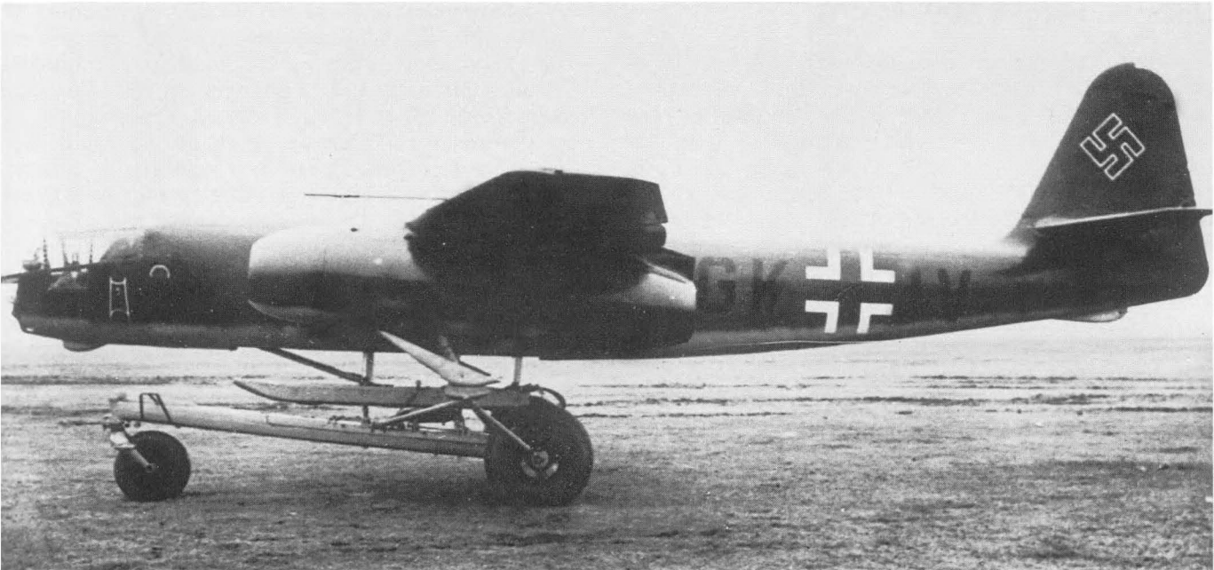
Fig 2.61A Arado Ar 234 V5 (GK+IV) powered by two Junkers 109-004 B-0s and showing the type of take-off trolley used prior to the development of a retractable undercarriage.
