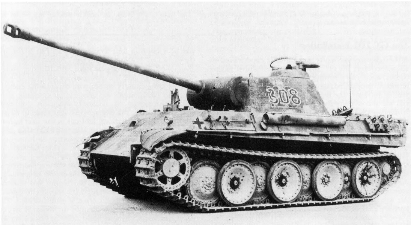
Fig 3.4 Panzerkampfwagen V G Panther (Sd.Kfz. 171) tank. In September 1944, this version of the Panther was chosen to be powered by a gas turbine unit to increase its power-to-weight ratio. With its standard piston engine, the Panther had already proved to be a formidable weapon. (Royal Armoured Corps Centre, Bovington)
