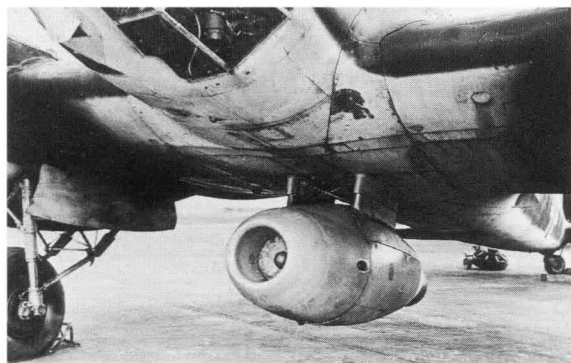
Fig 2.10 Heinkel He 280 V3 (GJ+CB). ABOVE LEFT: With engines uncowed owing to early fuel leaks. ABOVE: Later, following a landing skid.
