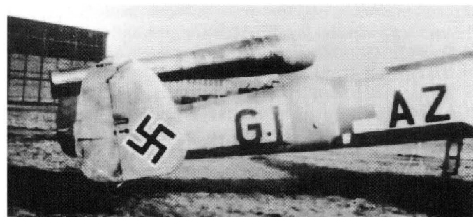
Fig 8.7 An Argus pulsejet fitted above a Messerschmitt Bf 110 (GI+AZ) flying test-bed, probably at E-Stelle Rechlin. Twin-finned aircraft such as this, the Ju 88 and the Do 217, were useful in this role.
