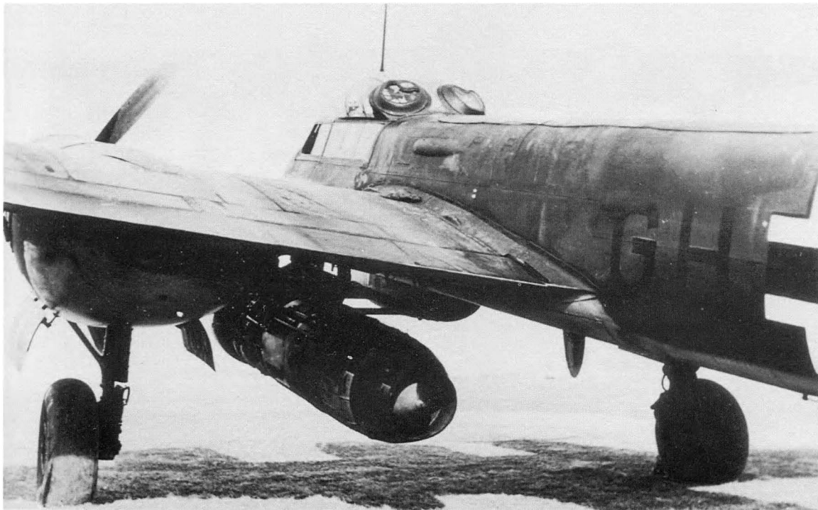
Fig 2.59 A Junkers Ju 88 A-5 (GH+--) with underslung Junkers 109-004 turbojet to perform flight tests. The engine is mounted at a hard point normally used to carry bombs.
