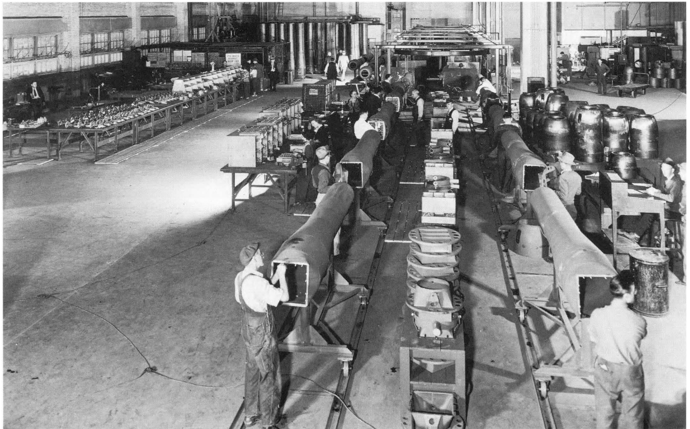
Fig 8.24 Late war production of PJ-31-1 pulsejets, based closely on the Argus model, by Ford in the USA. Most of the assembly stages are shown, including the arc welding of the tubes in the bays at the top centre of the picture. (Ford Motor Company)
