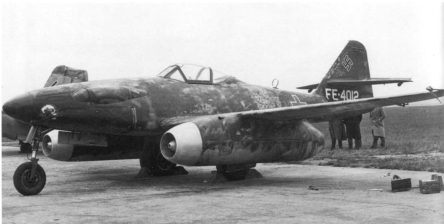
Fig 2.62 Messerschmitt Me 262 A-1a/U3, the photo reconnaissance version of the jet fighter, showing the nose bulge made to accommodate two vertical cameras. It was captured by the Americans and given the Foreign Evaluation number FE4012. A Junkers Ju 88 is behind. (US Air Force photograph taken on 30 September 1945)
