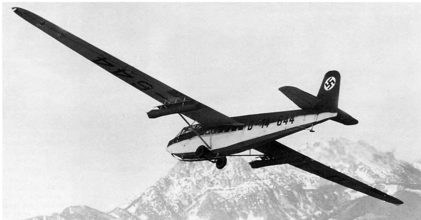
Fig 8.19 The DFS 230 glider (D-14-644) used to flight-test a pair of Argus 300 mm pulsejets. As a test bed, this assault glider had plenty of room for test equipment and various fuel system installations.
