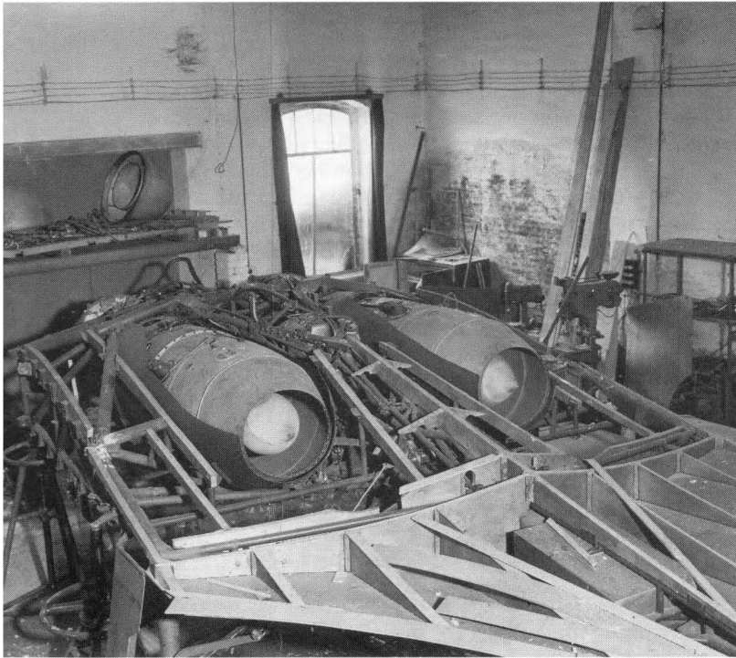
Fig. 2.67 A Gotha Go 229 all-wing fighter with two Junkers 109-004 C turbojets under construction. This plant, at Friedrichsrode, was captured by troops of the VIII Corps of the US Third Army on 14 April 1945. (US Army photograph)
