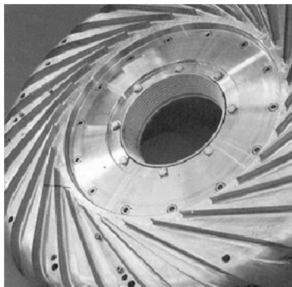
Figure 7.13 Nuovo Pignone vaned diffuser (courtesy of GE Power Systems).
