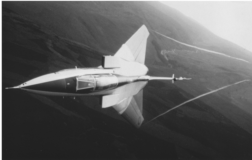
Figure 14.4. A photograph of a Tornado in a high-g turn with the trailing vortices made visible by condensation of water vapour. (Reproduced by permission of British Aerospace Defence Ltd, Military Aircraft Division)
