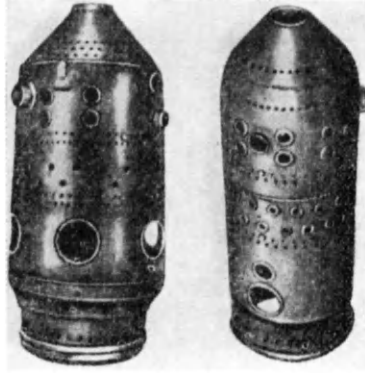
FIG. 81. Flame tubes of combustions chambers.
