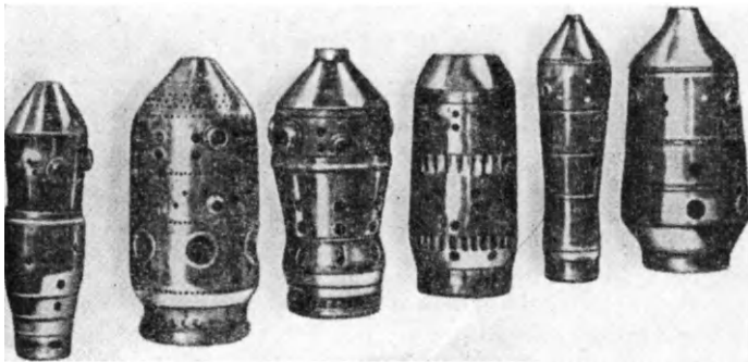
FIG. 82. Flame tubes of combustion chambers.
