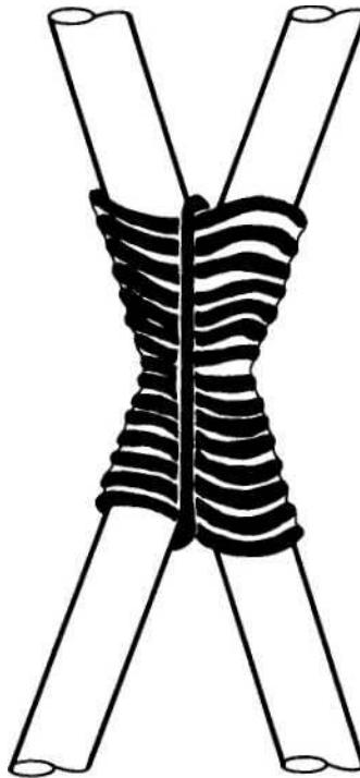
Figure 35. Tying and soldering
