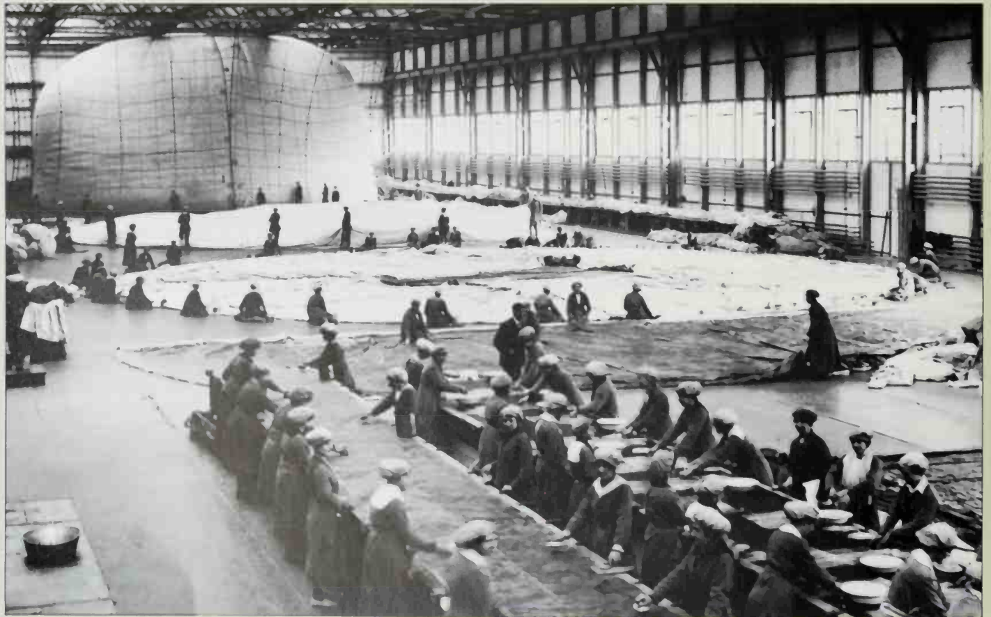
In the cavernous factory, the women at tables stick goldbeater's skins together (right) and glue them to a linen panel (left).
