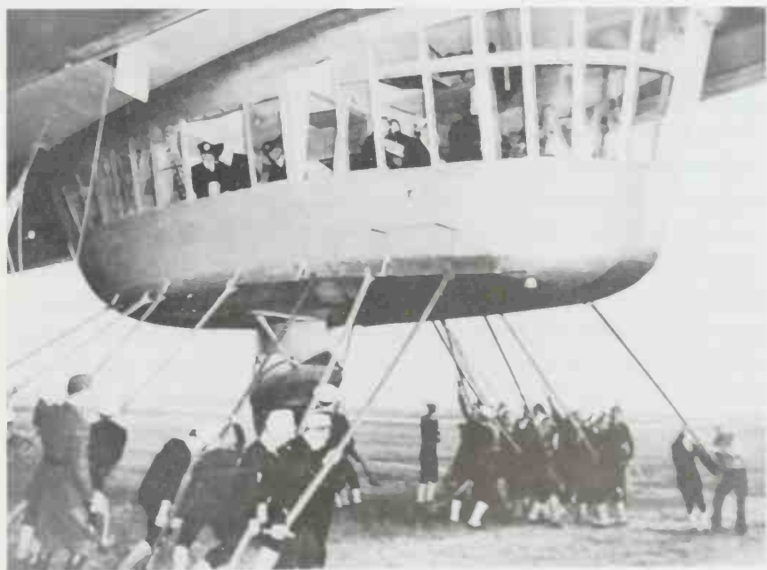
Bracing their poles, called crutches, against rails on the control car, Navy crewmen help position the Hindenburg for mooring to a mobile mast at Lakehurst. Low-pressure tires on shock-absorbing mountings protected the control car and lower fin from contact with the ground.
