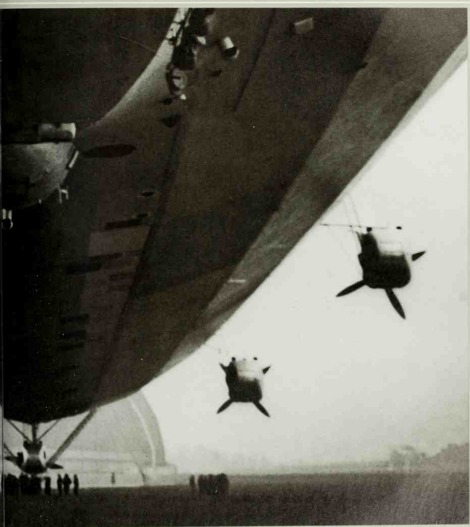
Ohio, in 1933. This view, looking astern, shows the after portion of the Graf's passenger gondola and all five of its externally mounted engines.
