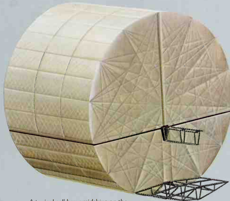
A typical cell bay amidships on the Graf held two separate cells with a narrow walkway running through them. The upper cell contained hydrogen; the lower one contained gaseous engine fuel.
