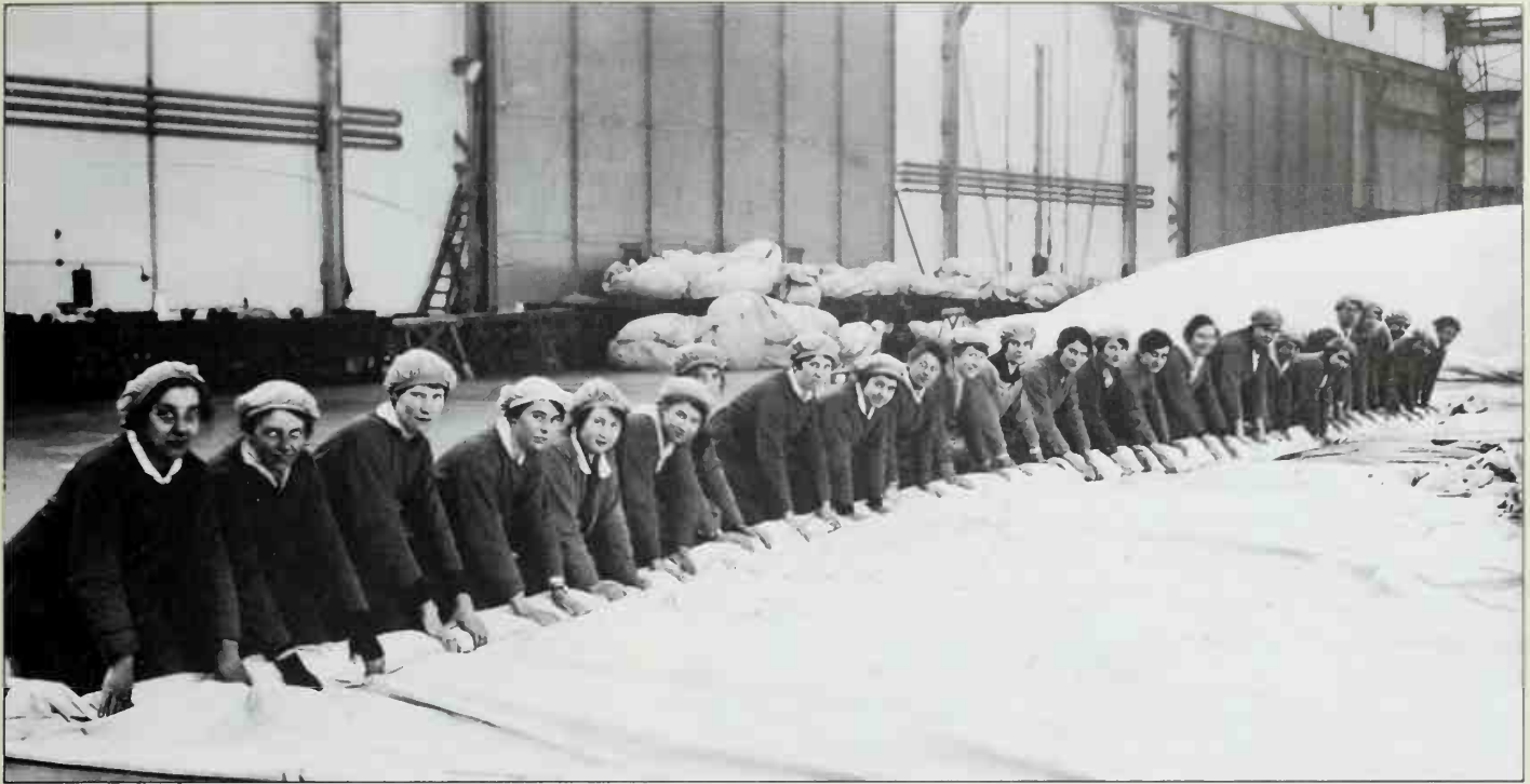
Once all the panels have been stitched together, two dozen workers roll up the finished cell to await testing.
