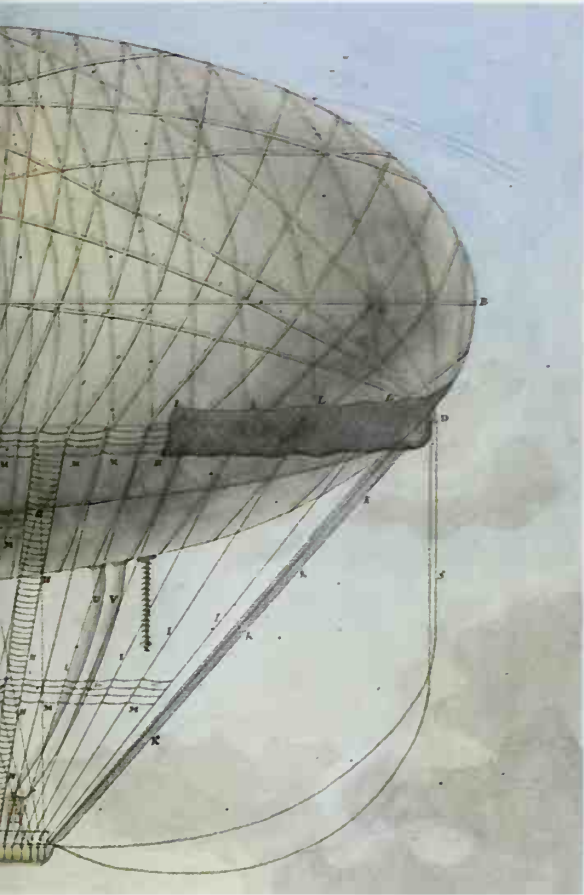
These 1785 watercolors by French soldier-engineer Jean-Baptiste-Marie Meusnier detail his revolutionary—and still-valid—concept of an ellipsoidal dirigible (above), streamlined to reduce air resistance, and a peak-roofed hangar (left) to house it.
