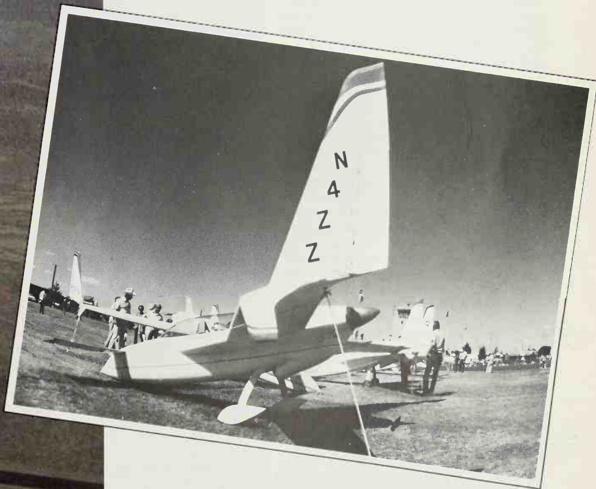
Above : The Rutan Vari-Eze is another variant on the canard theme, in this instance tailored to high performance.
