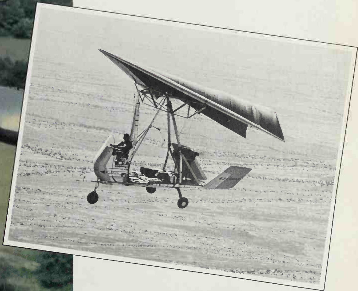
Above: Another approach to the pack-away aircraft is seen in the Ryan XV-8A Fleep, which has an ultra-light fuselage surmounted by a foldable hang-glider wing.
