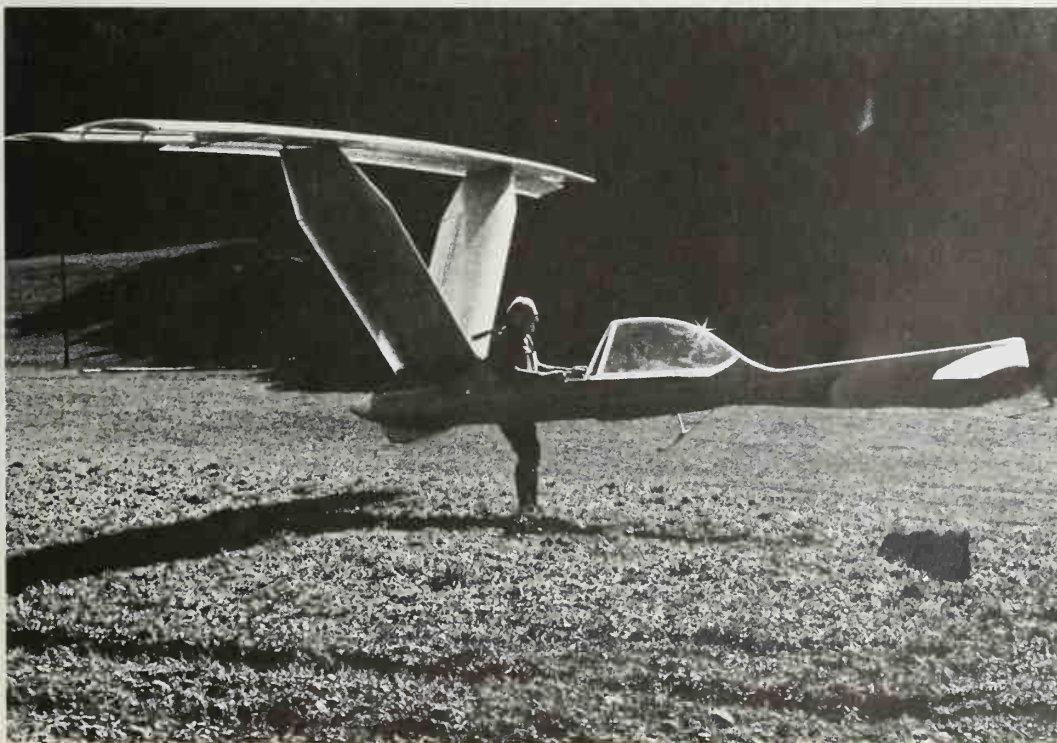
Left : At the other extreme of size, weight, complexity and performance is the Aviafiber Canard-2 FL ultra-light sailplane of Swiss origin. This interesting design has its rear wing set in parasol fashion on top of the large V tail, and has an advanced structure of great strength but low weight. The first example flew in September 1977.
