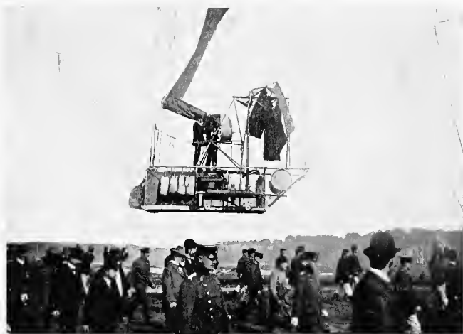
THE CAR OF THE "PARSEVAL" AIRSHIP (Note the collapsible blades of the propeller, and the air pump for filling the ballonet)
