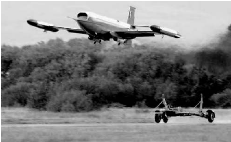
Figure 9.10 Aircraft Jindivik releases landing gear after take-off. Reproduced from permission of http://www.militaryimages.net
