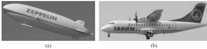
Figure 3.8 Lighter-than-air craft versus heavier-than-air craft: (a) Zeppelin NT; (b) ATR-42. Part (b) reproduced from permission of Anne Deus.
