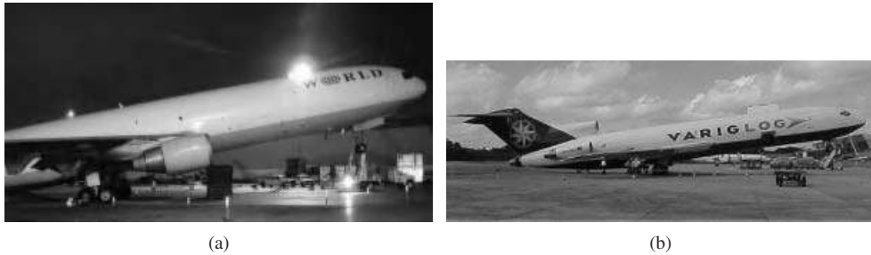
Figure 11.1 Too much load beyond the allowed aft cg creates an accident. (a) A McDonnell Douglas MD-11 nose up due to the cg aft of main gear; (b) A Boeing 727 nose up due to loading error in Brazil, June 9, 2001. Reproduced from permission of (a) Randy Crew; (b) Orlando J. Junior
