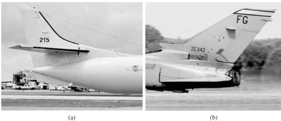
Figure 6.18 An adjustable tail and an all-moving tail: (a) adjustable horizontal tail in Fairchild C-26A Metro III; (b) all-moving tail in Panavia Tornado. Reproduced from permission of (a) Luis David Sanchez; (b) Antony Osborne.
