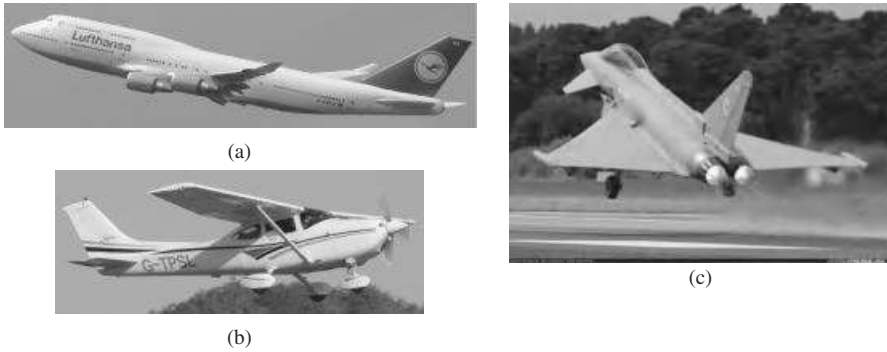
Figure 3.7 (a) Civil transport Boeing 747; (b) general aviation Cessna 182; (c) military aircraft, Eurofighter Typhoon. Reproduced from permission of (a) Anne Deus; (b) Jenny Coffey; (c) Antony Osborne.
