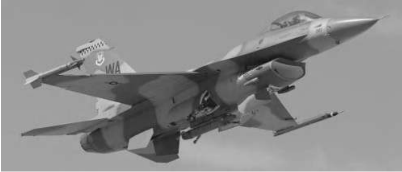
Figure 4.6 F-16 Falcon with an empty weight-to-take-off weight ratio of 0.69. Reproduced from permission of Antony Osborne
