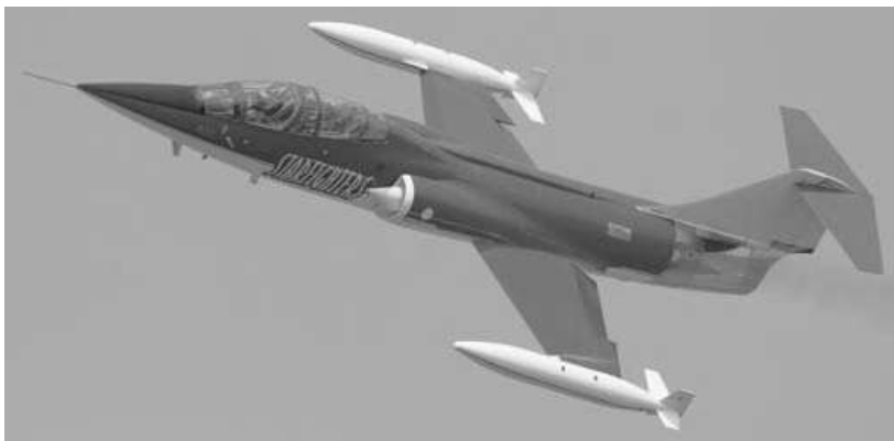
Figure 7.25 Lockheed CF-104D Starfighter with wing-tip fuel tanks. Reproduced from permission of Antony Osborne
