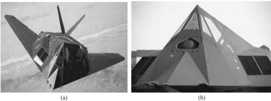
Figure 7.34 F-117 Night Hawk fuselage is designed to satisfy stealth requirements. (a) Fuselage, engine, and tail design for stealth, and (b) Sharp edges of fuselage (US Air Force)
