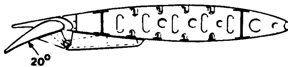
Figure 4.77 Single Slotted Flap Installation FR T-46
