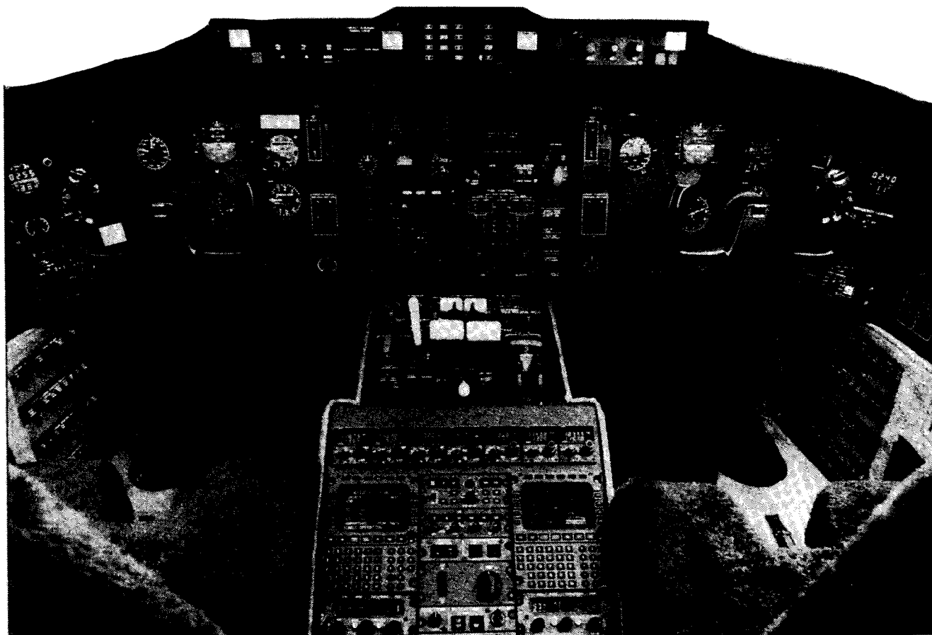
Canadair's Challenger 601-3A cockpit utilizes quiet/dark design principles.
