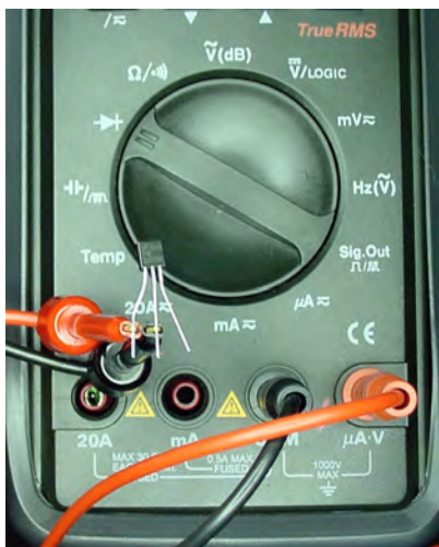
Figure 16-4. Setting up a multimeter for testing a transistor with the diode test function
