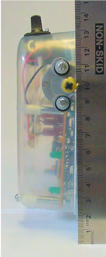
Figure 19-11. A ruler measuring the distance from the front of the robot to the center of the motor shaft
