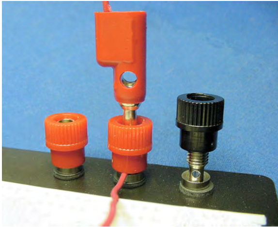
Figure 12-11. Three binding posts: Middle post has banana plug and wire
