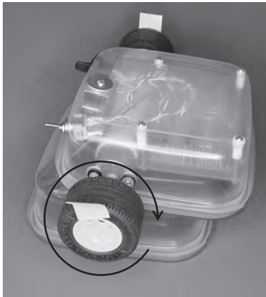
Figure 25-2. The robot's right motor spins clockwise
