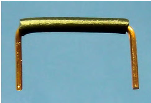
Figure 12-22. Completed homemade flat jumper wire
