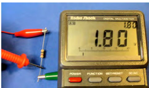
Figure 11-5. Red probe detecting the voltage at the point after the resistor
