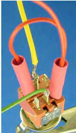
Figure 22-23. Diagonal side terminals covered in heat-shrink tubing and connected to left motor
