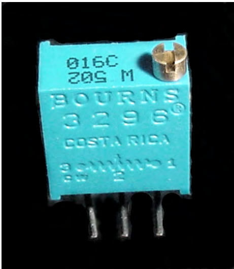
Figure 14-4. A breadboard-compatible multiturn trimpot
