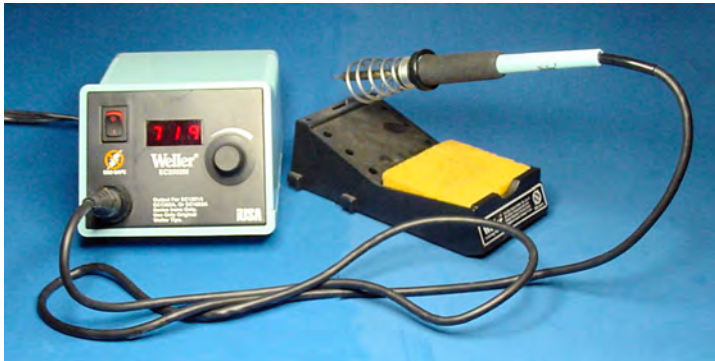
Figure 21-4. Temperature-adjustable soldering iron with sponge and stand
