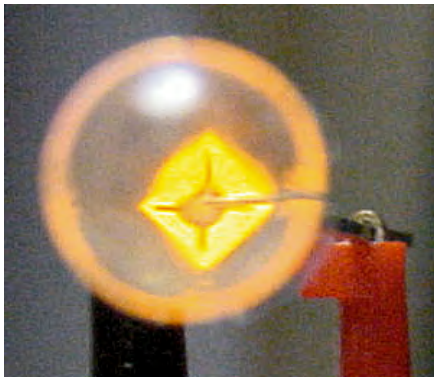
Figure 10-10. Glowing die with a view of the bonding wire and bonding site
