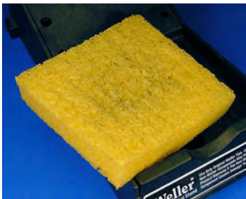
Figure 21-7. Moistened sponge for cleaning a soldering iron's tip
