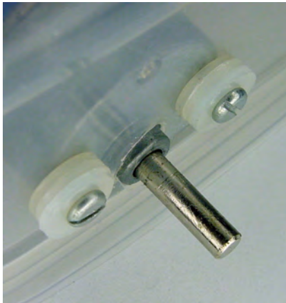
Figure 24-12. Test fit of motor with screws and washers
