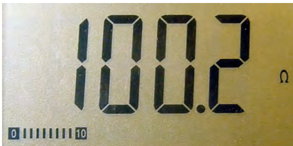
Figure 9-7. Meter displaying resistance of approximately 100 \Omega
