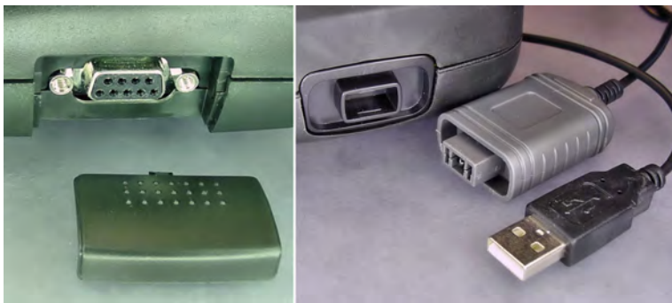
Figure 4-11. Connecting a multimeter to a personal computer with RS-232 DB9 (left) or optical USB (right)
