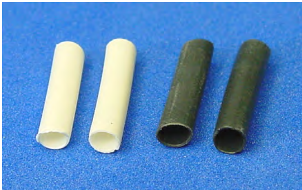
Figure 22-8. White and black \frac{3}{32} -inch diameter heat-shrink tubing cut to 1.5 cm lengths
