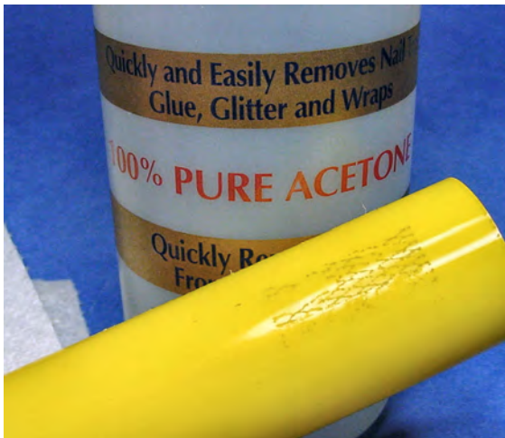
Figure 24-16. Removing sticker adhesive residue with acetone
