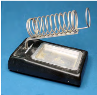
Figure 21-6. Soldering stand with metal coils to safely hold a hot soldering iron
