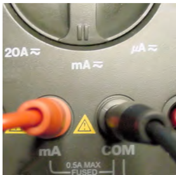
Figure 11-8. Multimeter setup for mA current flow
