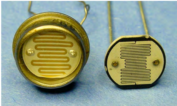
Figure 14-12. Encapsulated and exposed ceramic cadmium-sulfide photoresistors
