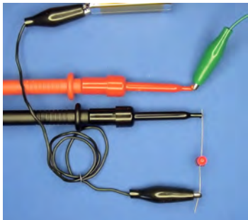
Figure 11-12. Counting current between the green clip and the LED
