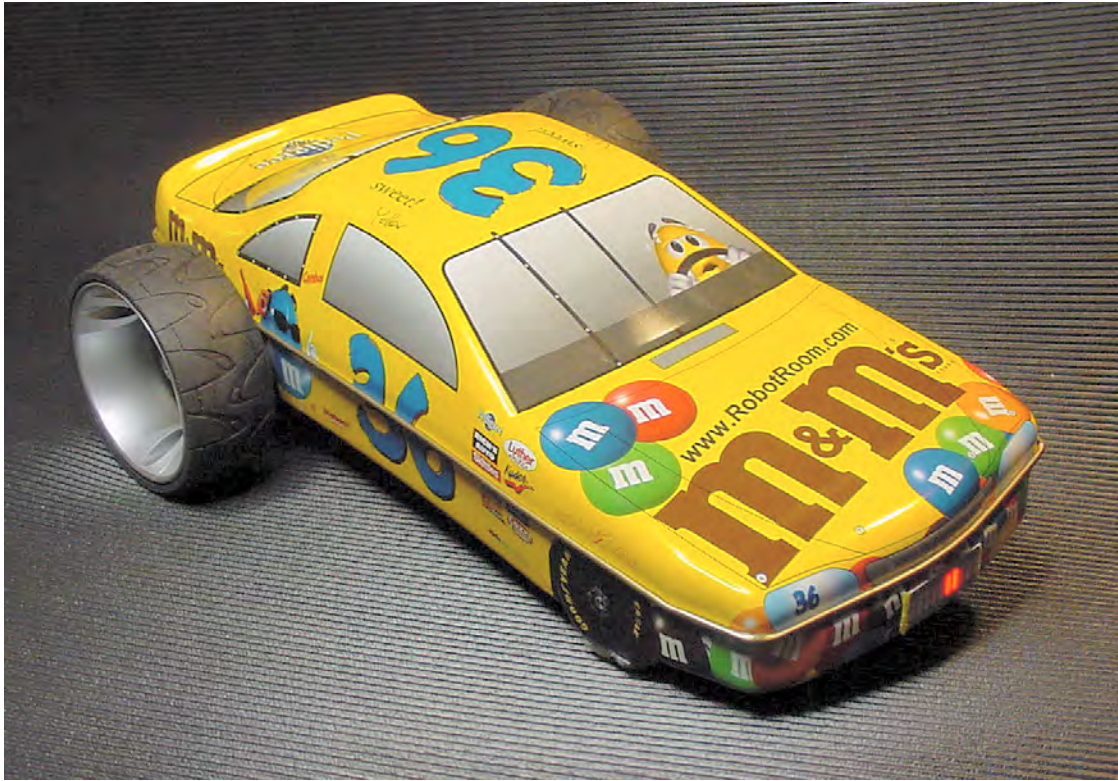
Figure 1-12. Line-following robot made from a candy container
