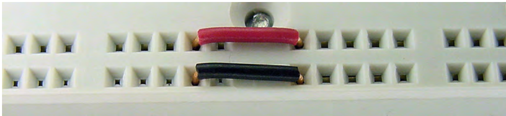
Figure 12-10. Extending buses by connecting with wire
