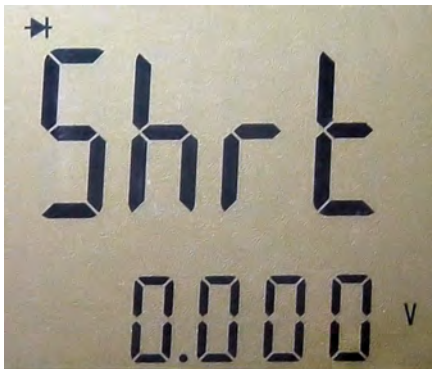
Figure 10-16. Short circuit or zero volts indicate a test error or damaged LED.
