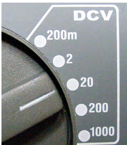
Figure 7-3. Dialing a DC voltage range above 9
