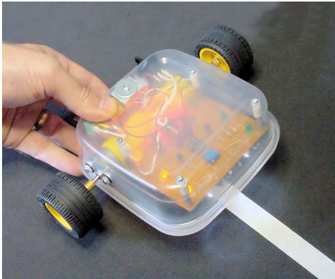
Figure 6-12. Placing the robot with sensors centered on the line
