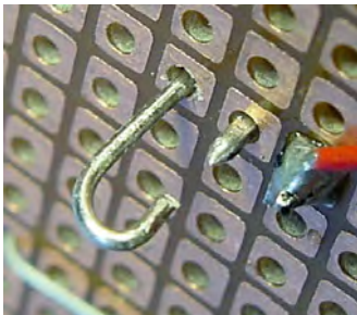
Figure 23-11. Bare wire shaped to connect to underside of Molex KK connector
