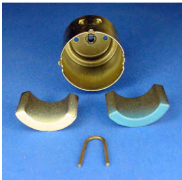
Figure 17-3. A pair of permanent magnets removed from the metal can. The clip in the foreground keeps the magnets from sliding together.
