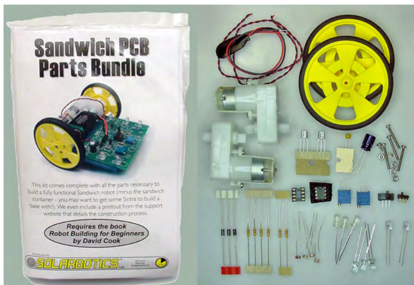
Figure 6-21. The Sandwich PCB Parts Bundle includes motors, wheels, printed circuit board, and electronics.
