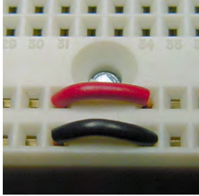
Figure 13-10. Jumper wires connecting the left side to the right side of the breadboard
