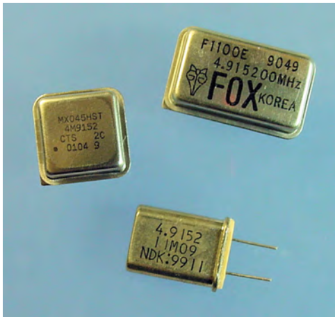
Figure 26-16. Half-can oscillator (middle left), full-can oscillator (top right), and crystal (bottom)
