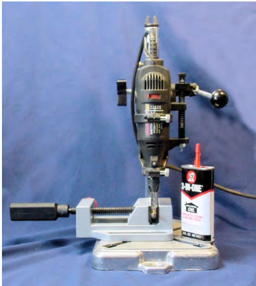
Figure 20-19. Dremel rotary tool installed on a Dremel drill press. Optional oil and drill-press vise also pictured.
