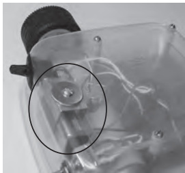
Figure 7-17. Battery mounted near rear axle
