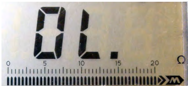
Figure 9-8. The resistor value is above the selected range on the multimeter
