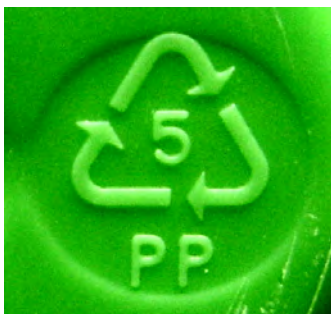
Figure 24-17. Recycling symbol indicates tube is polypropylene
