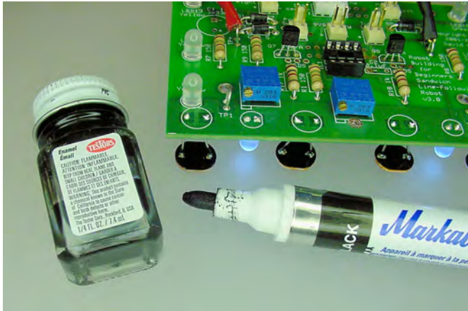
Figure 23-15. Black paint (left and bottom) and photoresistors raised 12 mm from circuit board surface (top right)
