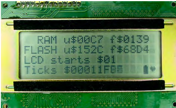
Figure 26-23. Standard 14-pin 20-character by 4-line LCD
