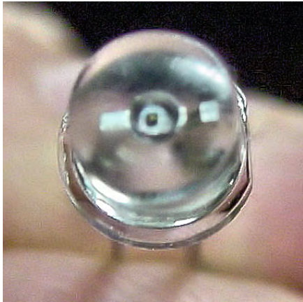
Figure 10-9. View of a reflector cup and die
