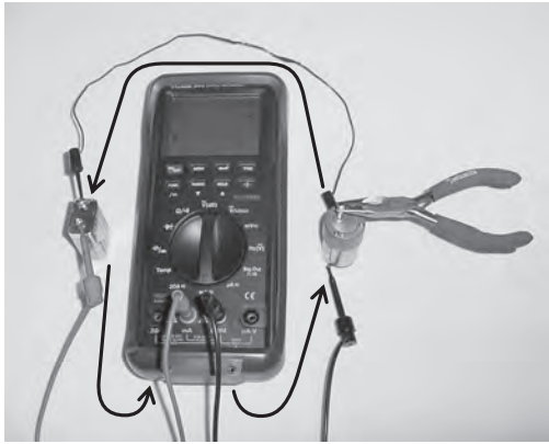
Figure 18-4. Testing motor current with a multimeter and pliers
