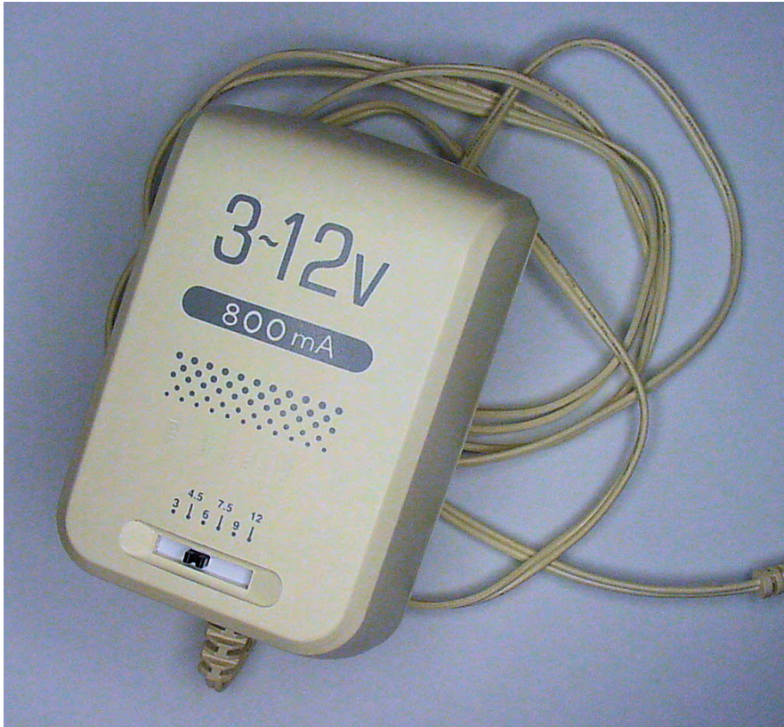
Figure 3-6. An AC-to-DC transformer with adjustable voltages from 3 volts to 12 volts
