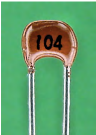
Figure 5-6. Not much room for a label (104 represents 100000 pF)
