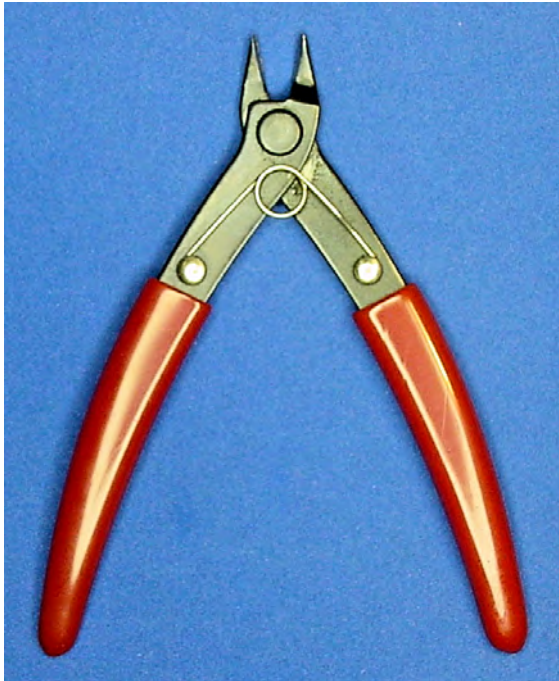
Figure 9-5. Flush wire cutter or nippy cutter
