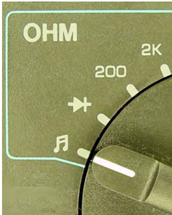
Figure 8-5. Multimeter dial set to continuity
