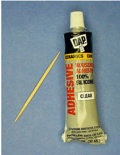
Figure 23-8. DAP clear silicone adhesive with a toothpick for applying
