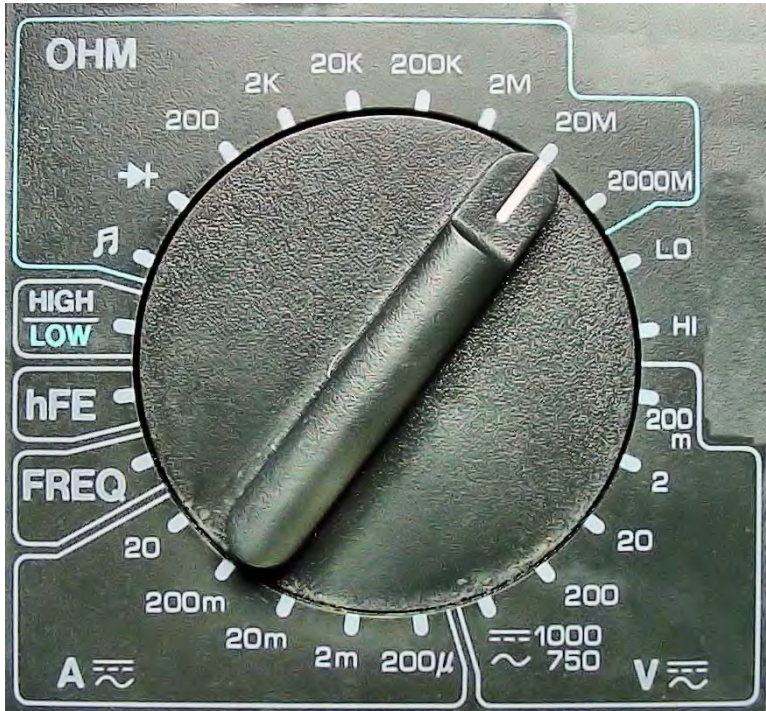
Figure 4-7. Dial with groups of manual range settings
