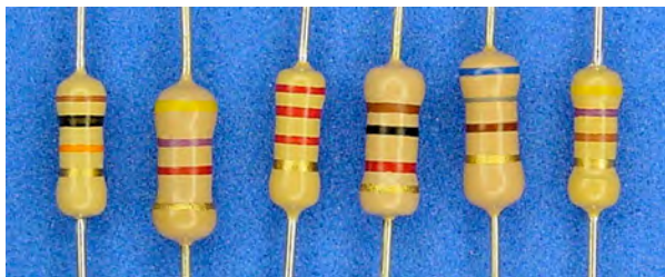
Figure 11-11. Resistor values for experimenting: from 10,000 \Omega down to 470 \Omega
