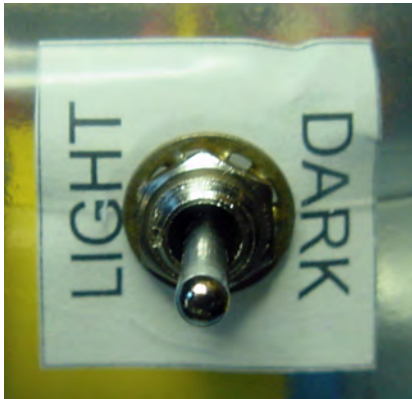
Figure 25-3. A printed piece of paper inserted inside the container for labeling the line-following switch
