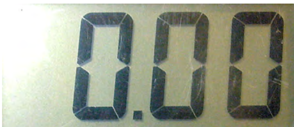
Figure 7-4. Meter displays no voltage
