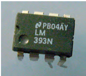
Figure 27-3. A destroyed LM393N comparator
