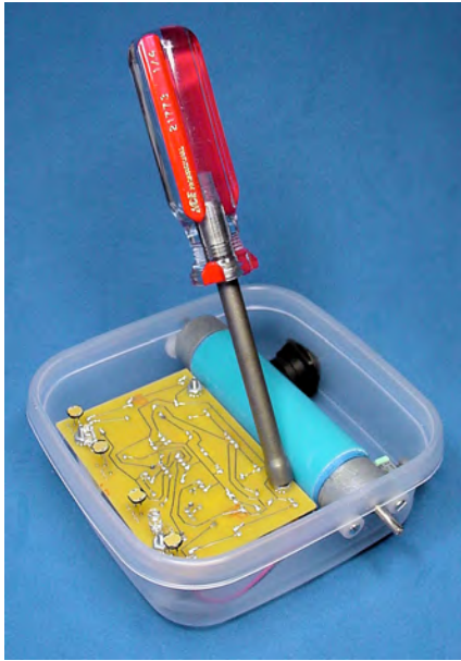
Figure 24-28. Nutdriver tightening nuts onto standoff screws
