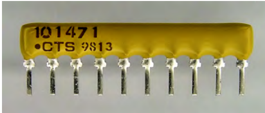
Figure 26-7. Resistor network consisting of nine 470 \Omega resistors in one package
