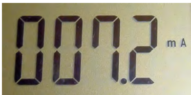
Figure 11-10. Multimeter displaying 7.2 mA of current flowing through circuit
