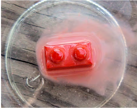
Figure 24-18. Acetone destroying a standard LEGO brick
