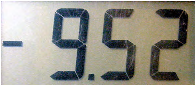
Figure 7-6. A negative number indicates a mixed-up connection
