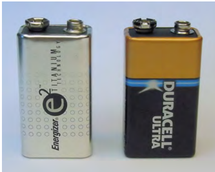
Figure 7-15. Tweaked alkaline 9 V batteries
