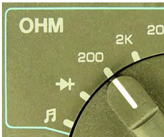
Figure 8-6. Multimeter dial set to lowest ohm range
