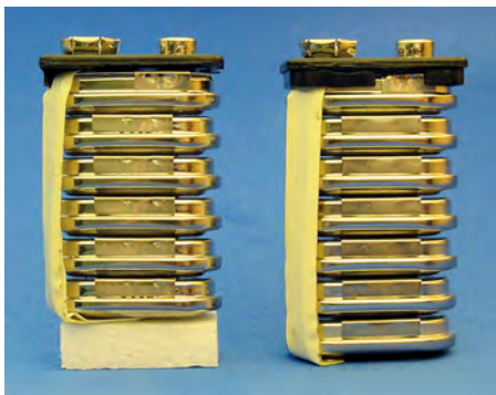
Figure 7-16. Polystyrene foam filler in a less-powerful battery
