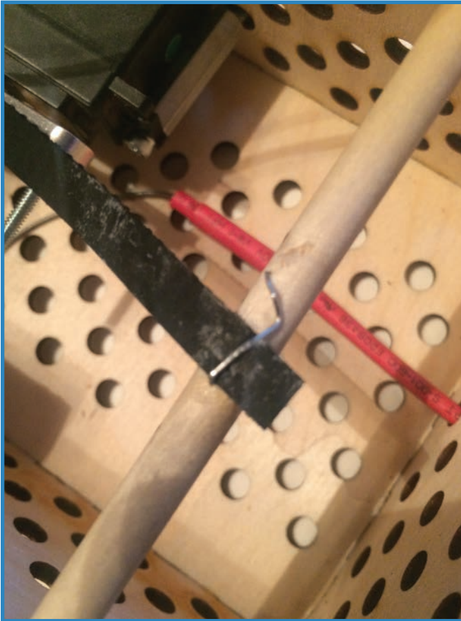
FIGURE 7.16 Staple and glue the timing belt to the wooden dowel and then wrap it around.
