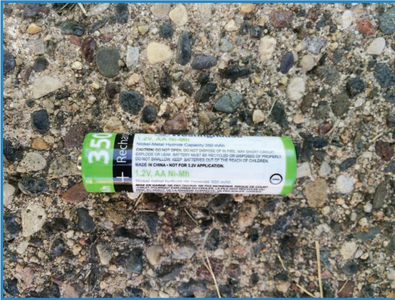
FIGURE 10.2 NiMH batteries are a popular choice for drones.
