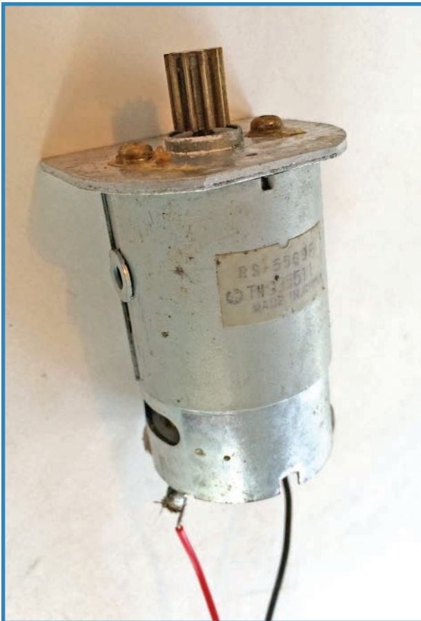
FIGURE 6.3 A brushed motor, identifiable by its two leads.
