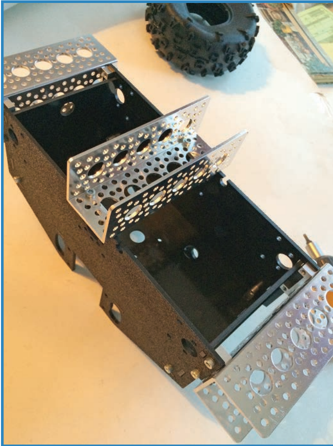
FIGURE 13.11 These channels will eventually hold sensors.
