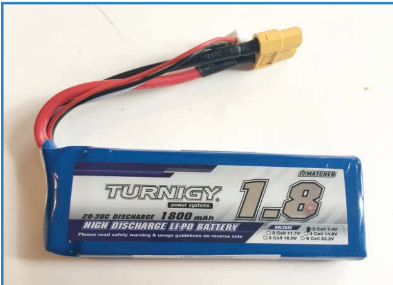
FIGURE 10.3 LiPo batteries are the go-to power solution for most drones.
