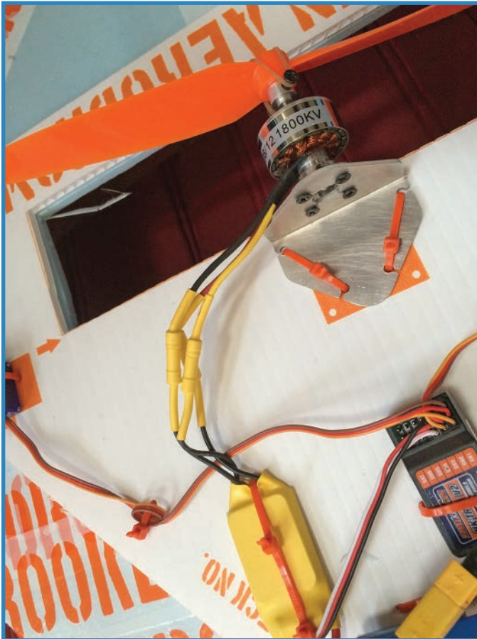
FIGURE 6.4 An AC motor with the matching speed controller.
