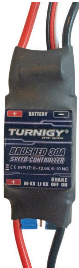
FIGURE 8.4 This 30A ESC is designed for brushed DC motors.
