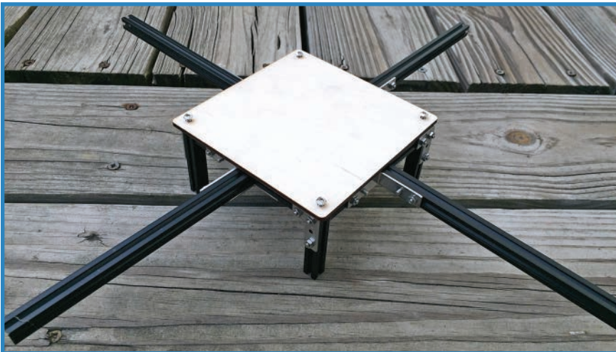
FIGURE 4.15 Attach the wooden platform to the tops of the legs.
