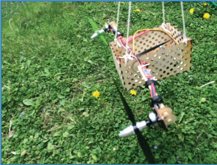
FIGURE 7.5 The blimp drone uses balloons to hoist itself into the air.
