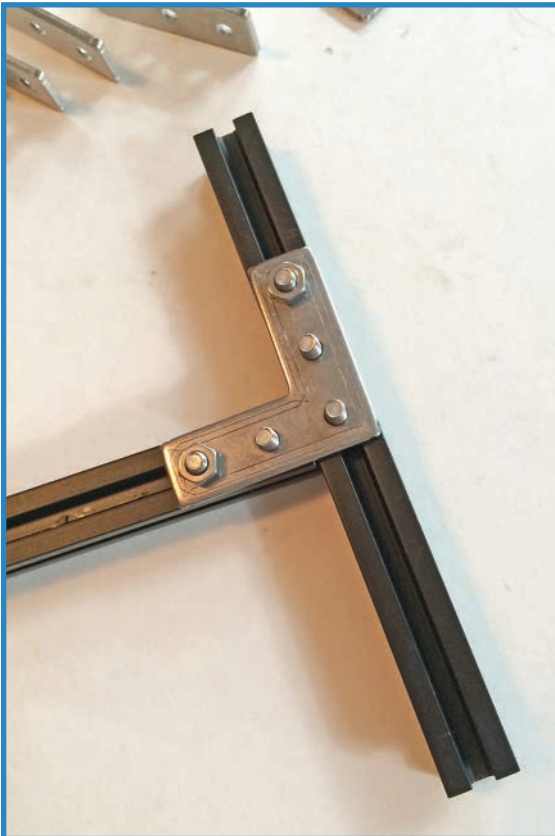
FIGURE 4.10 Make a “T” with the two beams and secure with a bracket.
