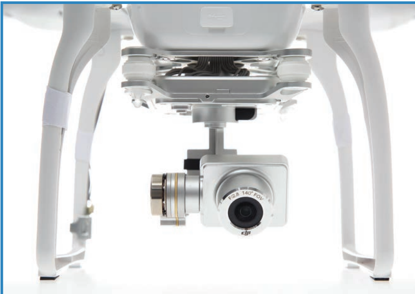
FIGURE 3.5 The Vision+, true to its name, has a gimbal-mounted camera that comes with it (credit: DJI).
