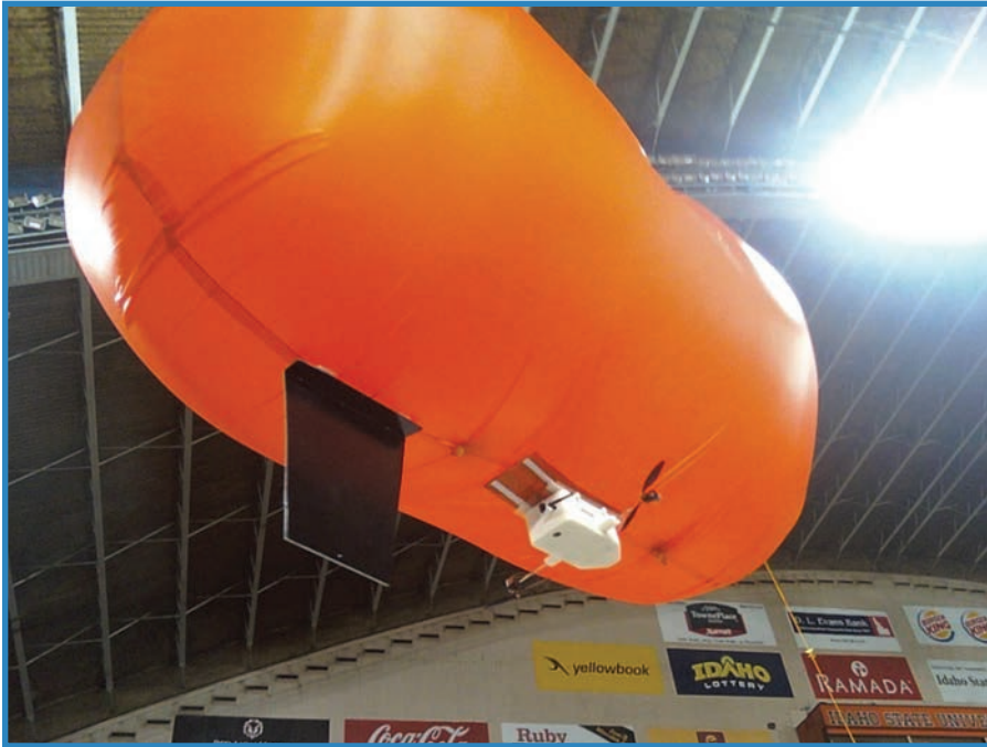
FIGURE 2.5 This blimp features a 3D-printed cabin (credit: Geran Call).
