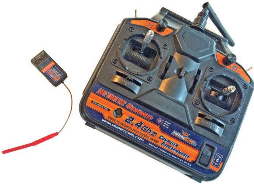
FIGURE 8.7 The HobbyKing receiver I used in this book is fairly typical for a six-channel receiver.
