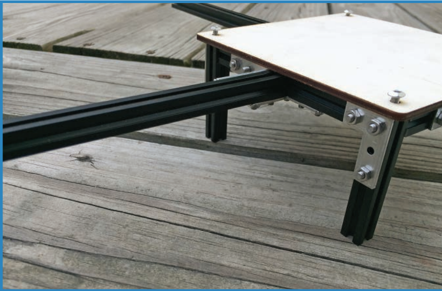
FIGURE 4.6 The MakerBeam chassis serves as a light and flexible platform upon which to build your quadcopter.
