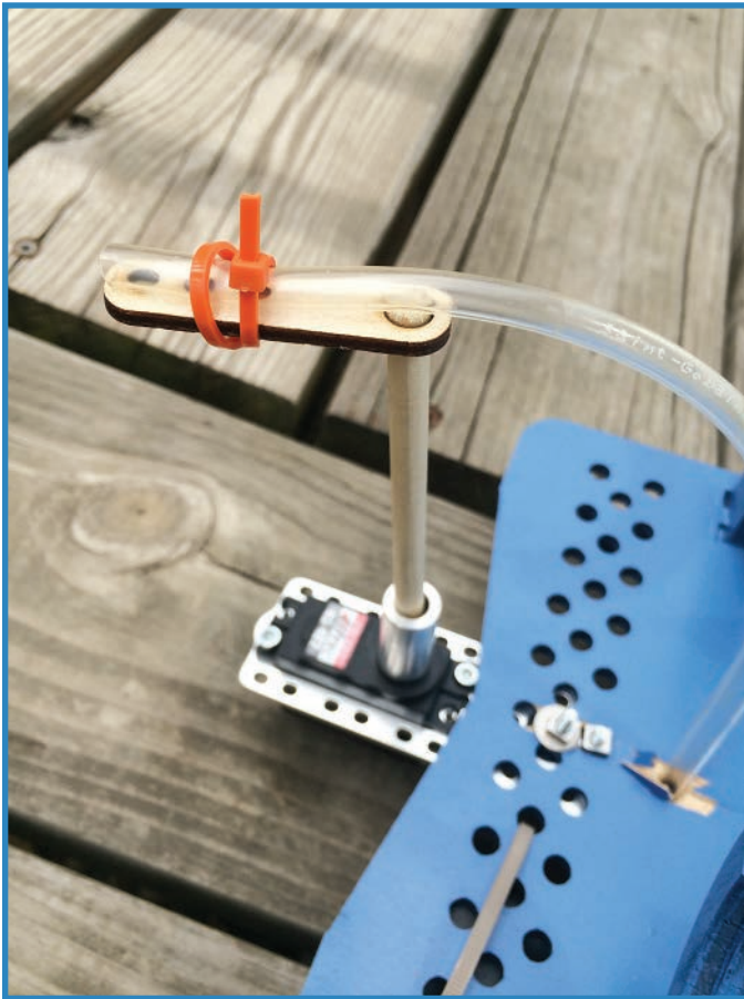
FIGURE 11.22 Angle the output tube to propel the drone forward.
