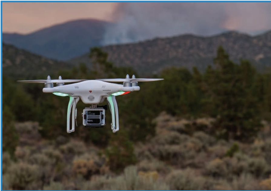
FIGURE 3.6 The Phantom's distinctive LEDs not only illuminate the quadcopter, but also tell the operator which way is forward (credit: DJI).
