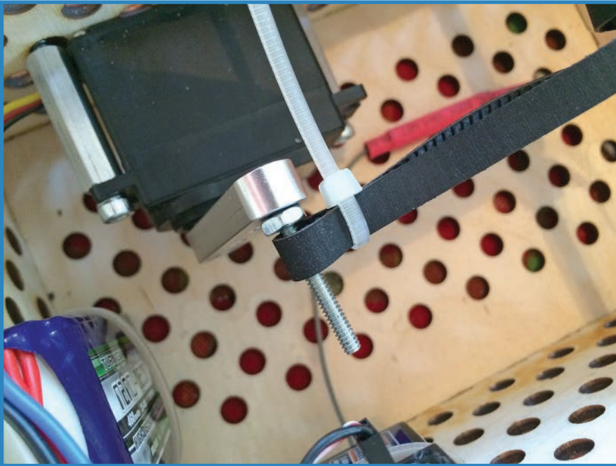
FIGURE 7.17 Zip-tie the timing belt to a #4 screw attached to the servo arm.
