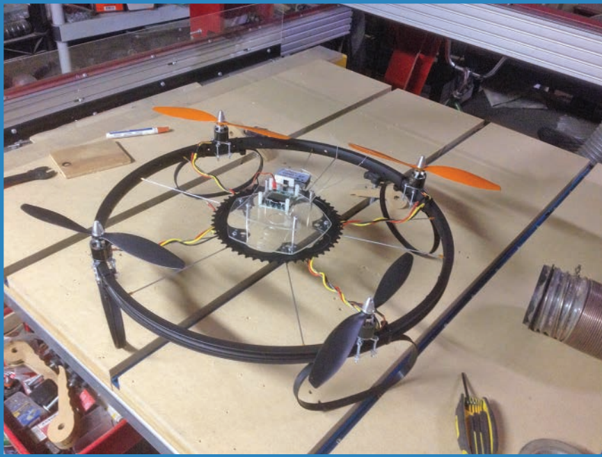
FIGURE 2.1 Sam Ley made clever use of found material to make his quadcopter's airframe (credit: Sam Ley [CC-A]).
