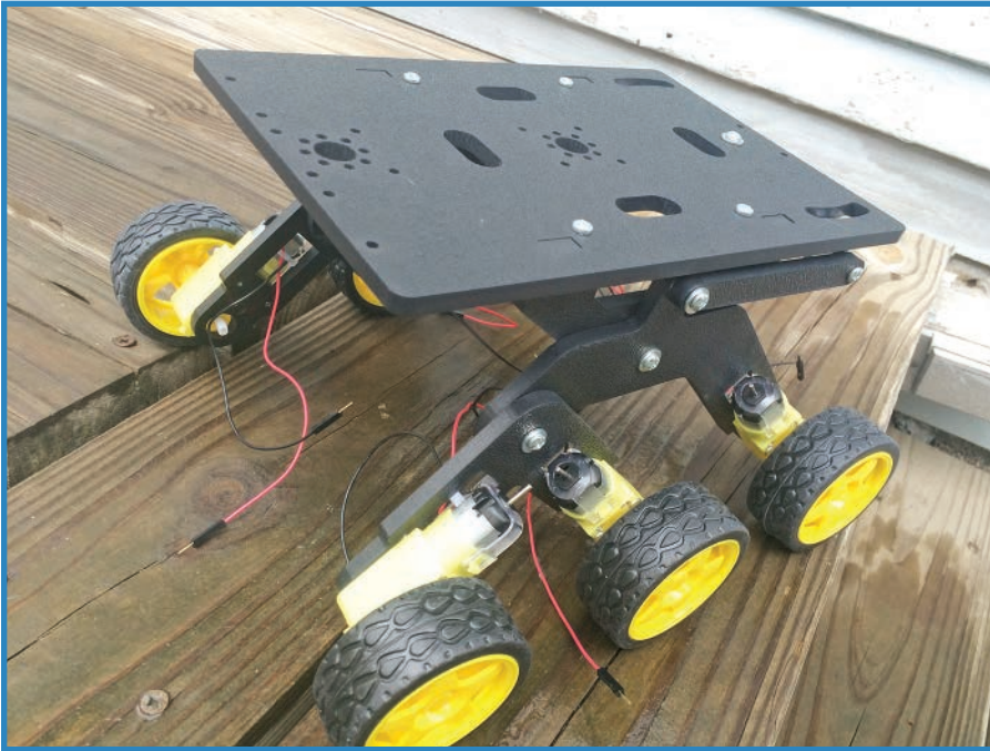
FIGURE 13.6 The Bogie offers a tough-as-nails platform for an all-terrain rover.
