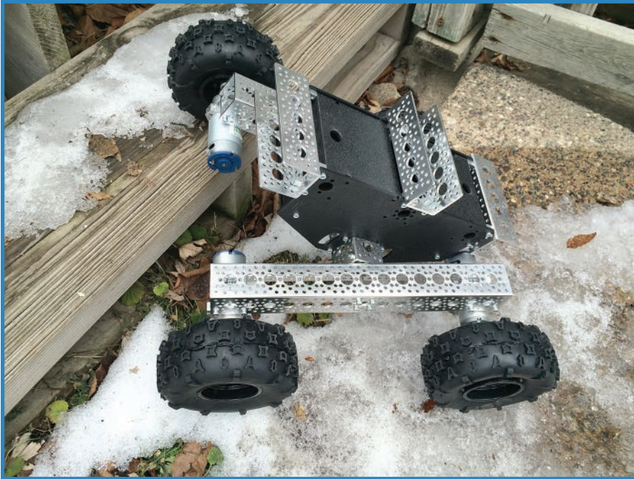
FIGURE 3.12 The knobby tires are a boon when traversing rough terrain.
