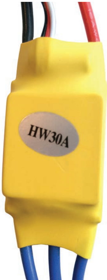
FIGURE 8.3 The HW30A is a good all-around 30-amp ESC.
