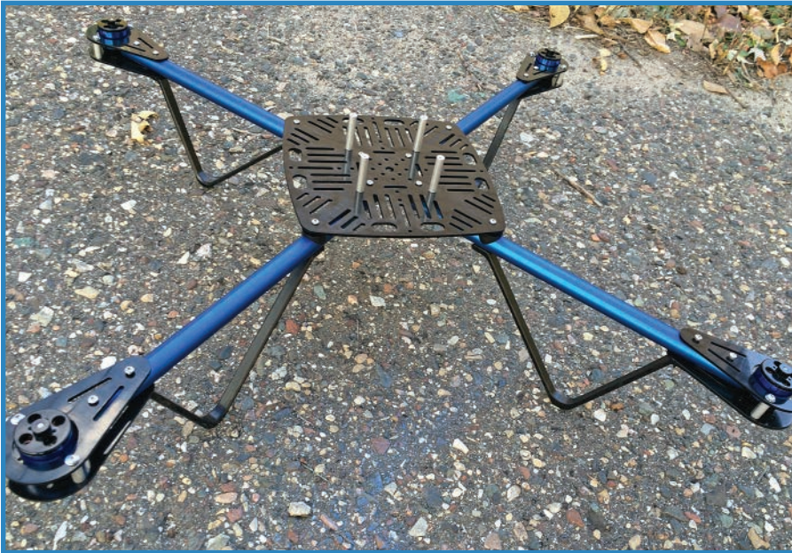
FIGURE 4.2 The Parallax ELEV-8 features a lightweight airframe made out of plastic and aluminum.
