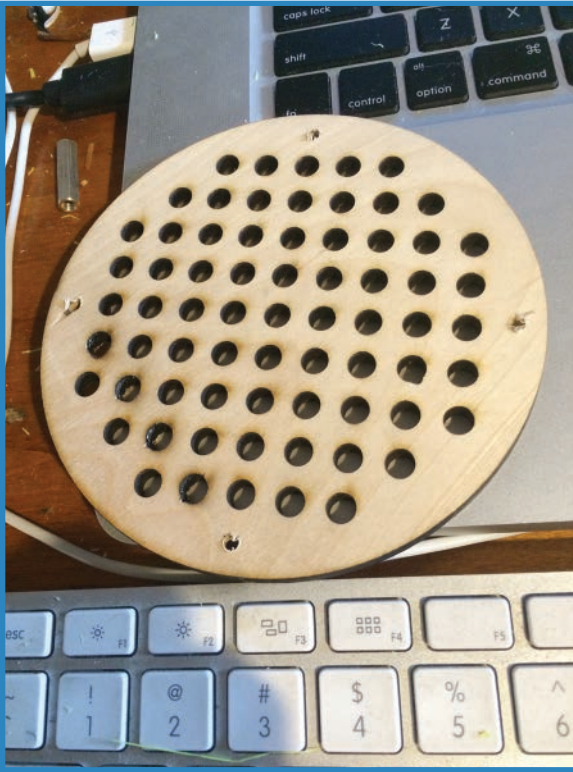
FIGURE 12.17 The laser-cut plate will protect the top of the quadcopter.
