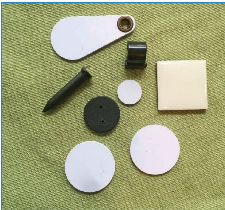
FIGURE 13.7 RFID tags come in different shapes and sizes.
