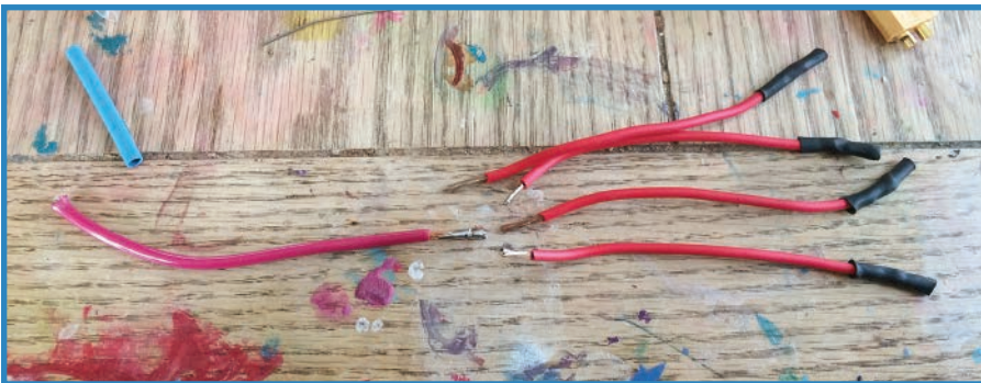
FIGURE 10.16 Solder together the wires.
