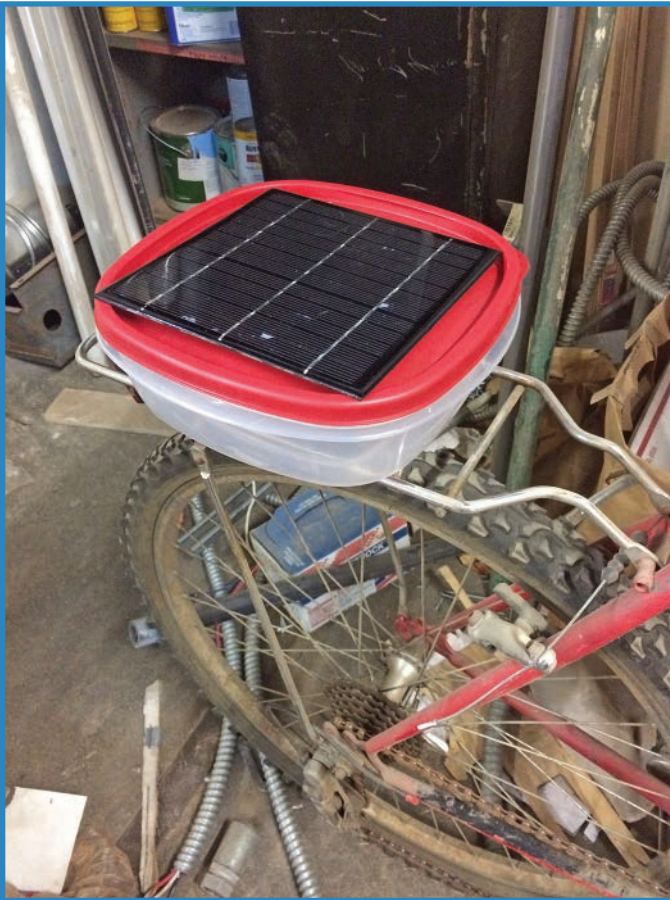
FIGURE 11.3 This food storage container makes an excellent project enclosure for not a lot of money.
