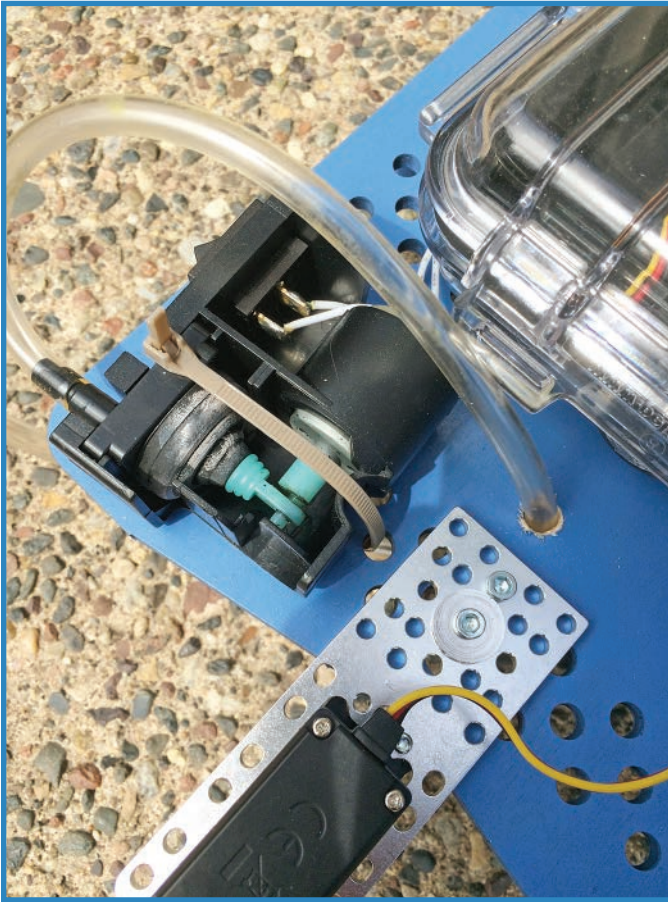
FIGURE 11.21 Slide the tube through a hole in the chassis.
