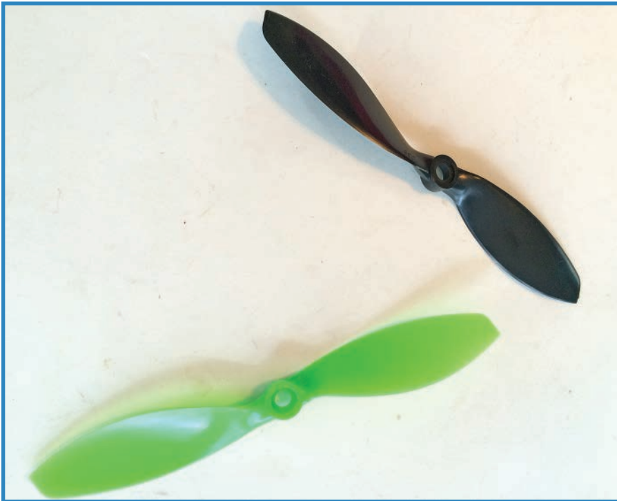
FIGURE 6.5 Regular and pusher propellers are made to rotate opposite each other.
