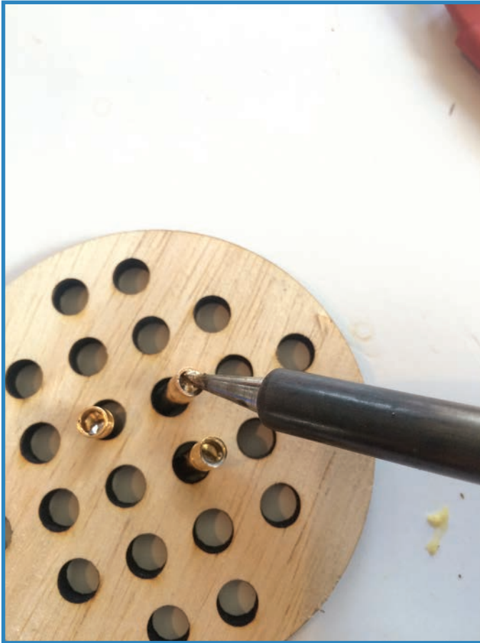
FIGURE 10.8 Fill up the bullet connectors with solder.
