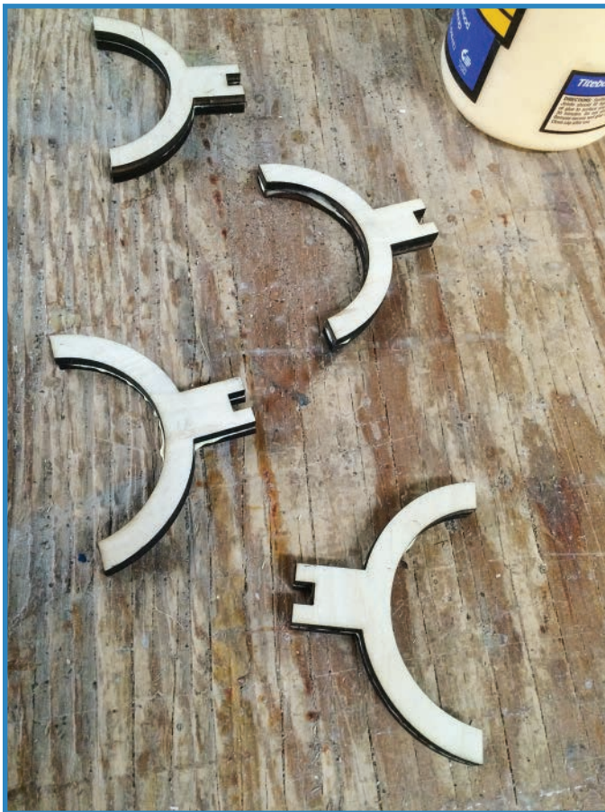
FIGURE 11.8 The chassis design includes these bottle rests.
