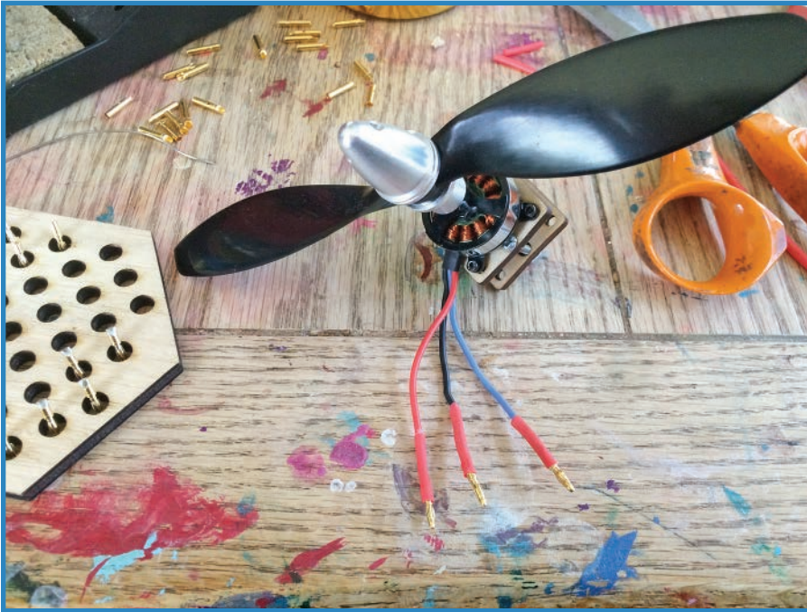
FIGURE 10.4 Bullet connectors are the preferred connection method in the RC world.
