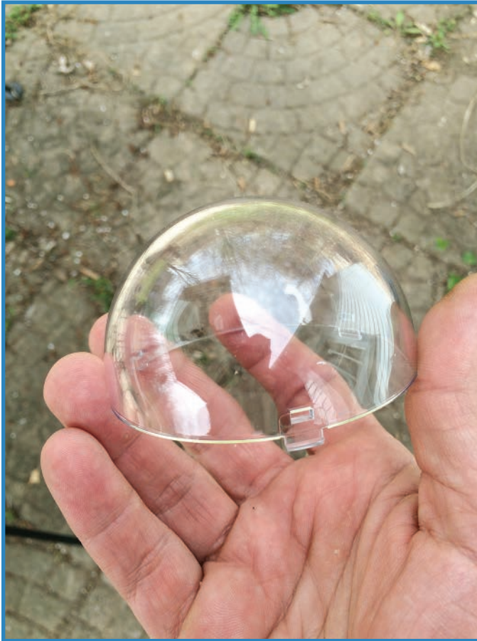
FIGURE 12.6 A protective dome can save your electronics package from a hit.
