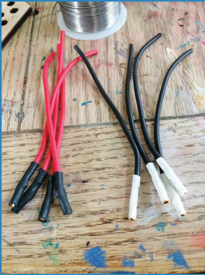
FIGURE 10.14 Add bullet connectors.
