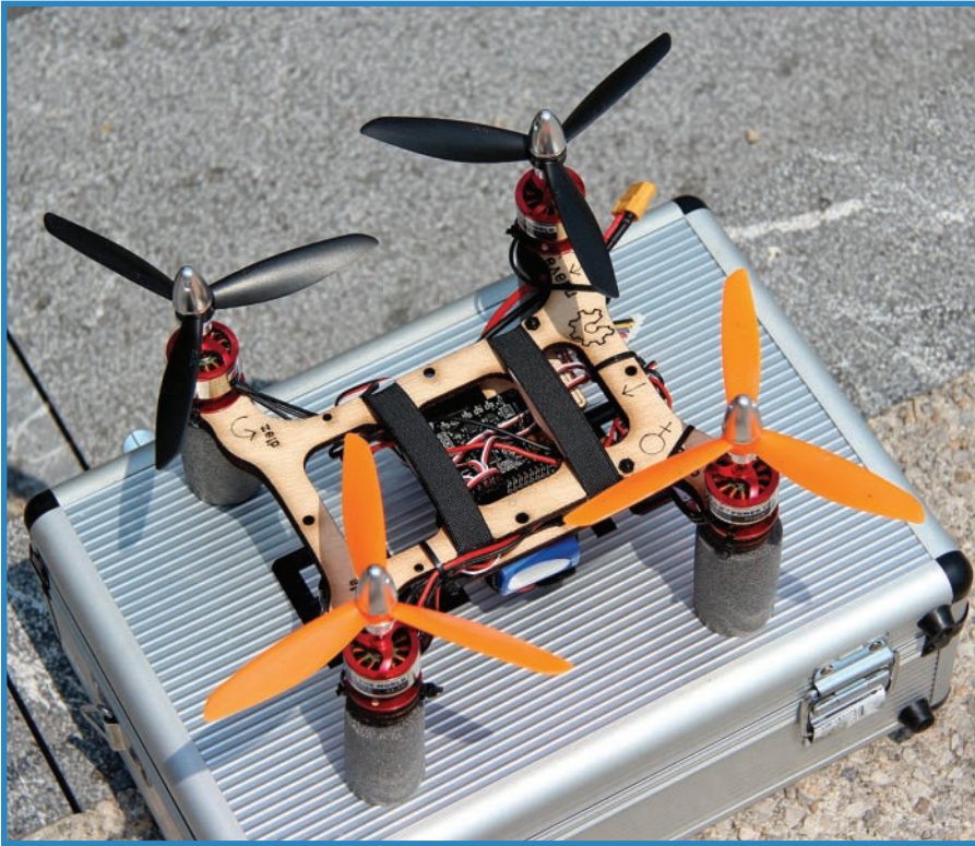
FIGURE 4.5 The Flone airframe is easily laser-cut out of a piece of wood (credit: Lot Amoros).
