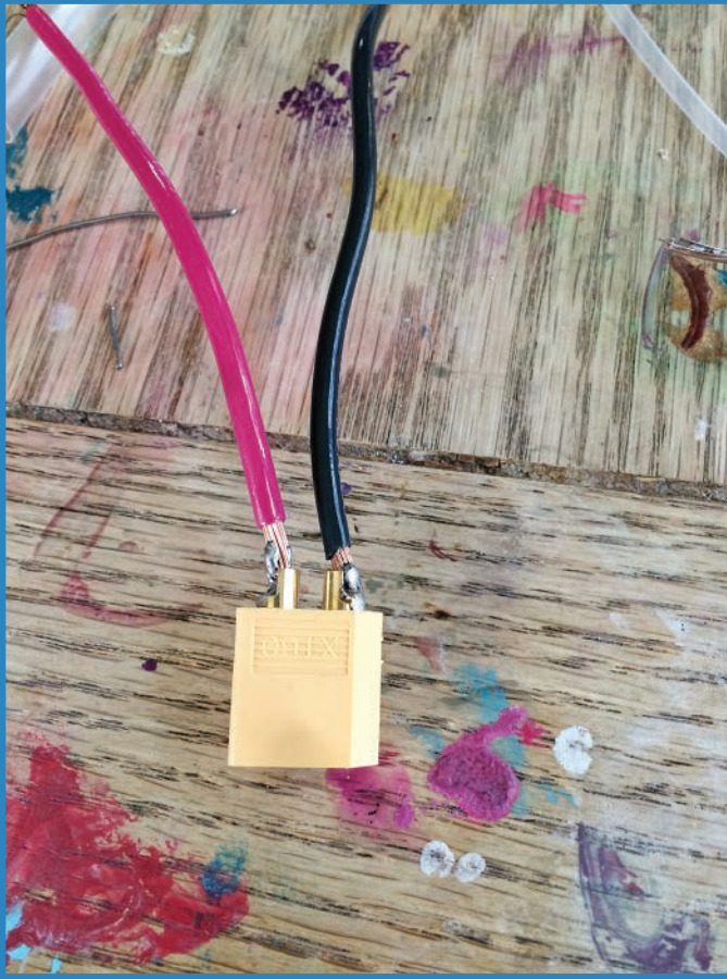
FIGURE 10.17 Add XT60 connectors to the battery ends and the 12-gauge wires.
