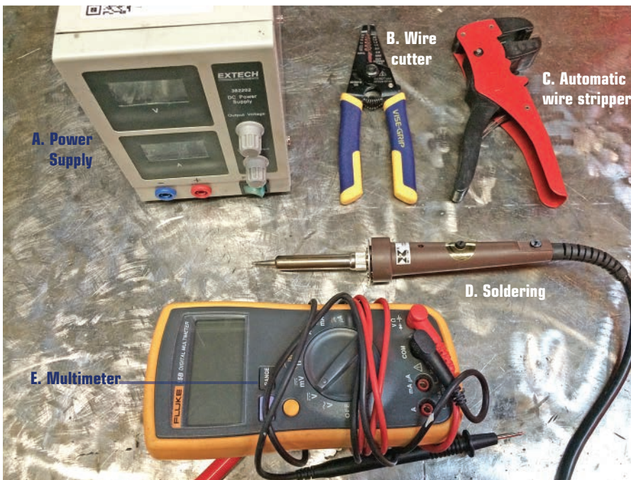
FIGURE 9.5 Working in electronics? Buy these tools.
