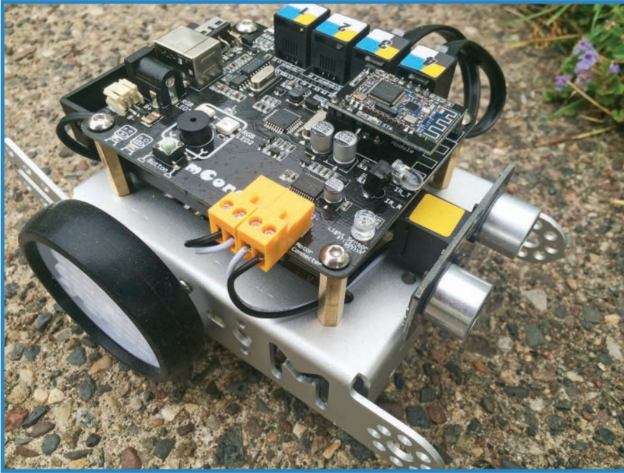
FIGURE 13.4 The mBot robot comes equipped with a bevy of sensors.
