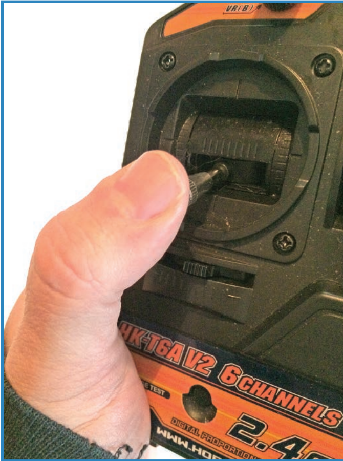
FIGURE 8.6 Use your transmitter to program your ESC.
