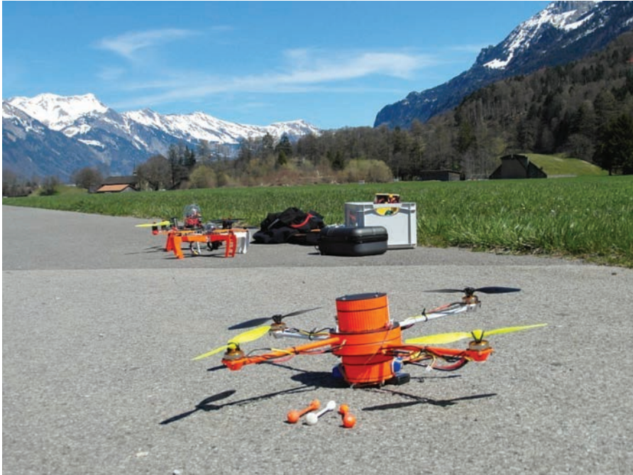
FIGURE 2.8 Roger Mueller’s foldable quadcopter survived a fall that broke its landing struts (credit: Roger Mueller).
